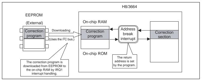
Figure 1 Specification of ROM Correction
