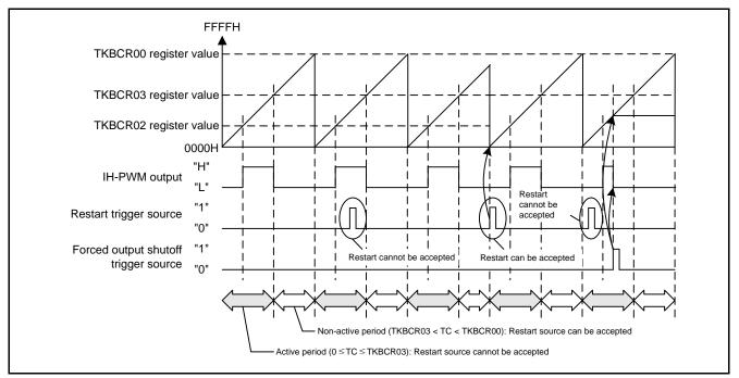
Figure 1.1 PWM Output Function for IH Control
