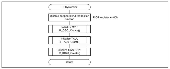
Figure 4.4 Peripheral Function Initialization
