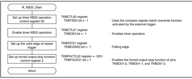
Figure 4.12 Enable Timer KB20 Operation
