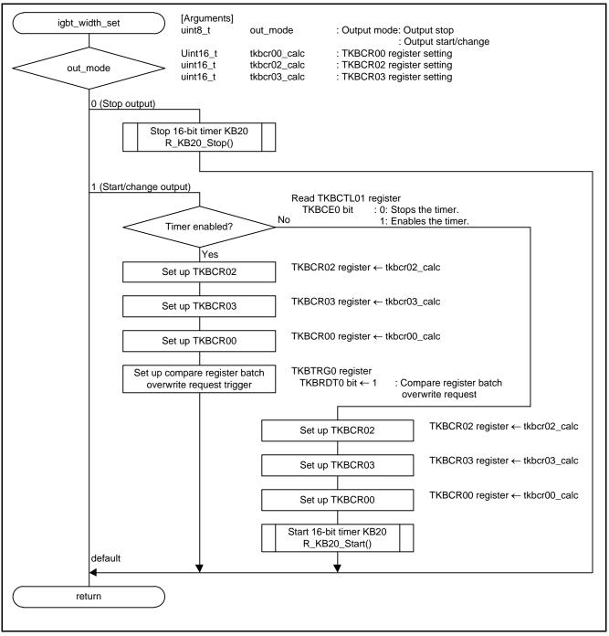
Figure 4.15 IGBT Output Setup
