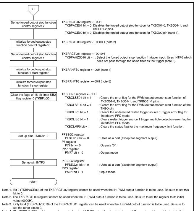
Note 4. The TKBPAHFS0 register cannot be used when the IH-PWM output function is to be used. Be sure to set the register to its initial value (00H). Be sure to set the other bits to 0.
