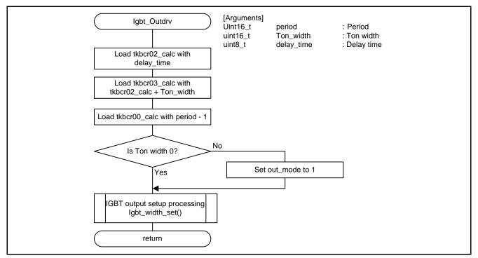
Figure 4.14 IGBT Output Driver Setup
