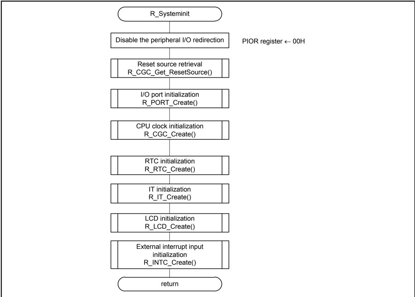
Figure 5.5 Peripheral Function Initialization
