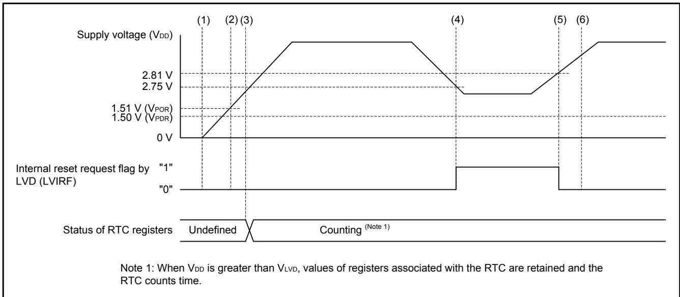
Figure 5.2 Operation Overview of Supply Voltage Shift and RTC Status
