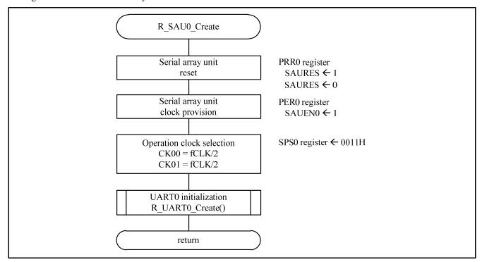
Figure 5.9 Serial array unit initialization function
