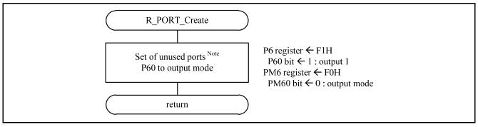
Figure 5.4 I/O Port Setup
