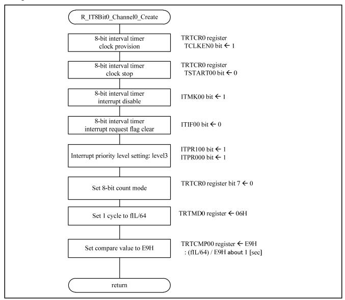
Figure 5.8 8-bit interval timer initialization function
