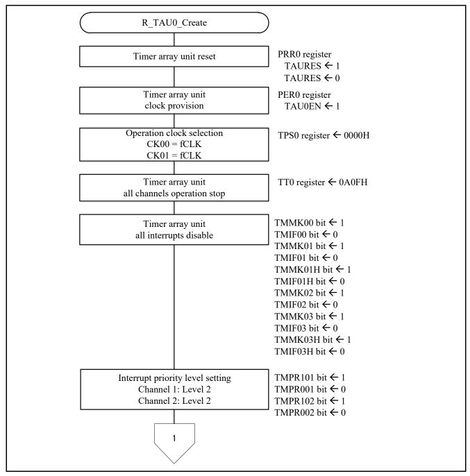
Figure 5.6 Timer array unit initialization(1/2)
