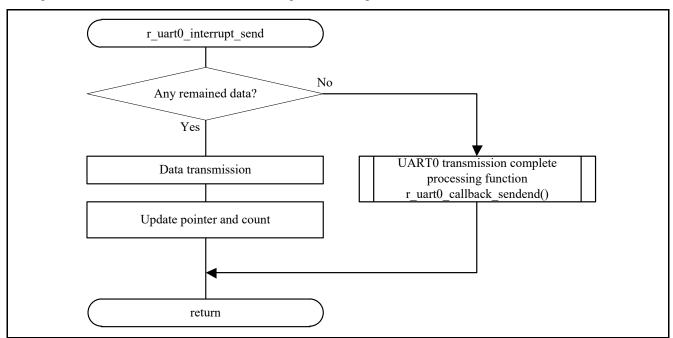
Figure 5.21 UART0 transmission complete interrupt function
