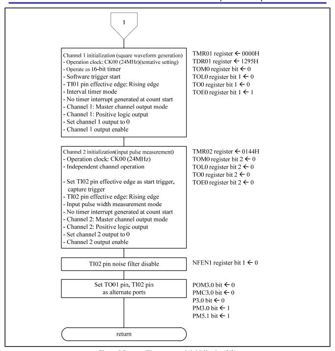
Figure 5.7 Timer array unit initialization(2/2)
