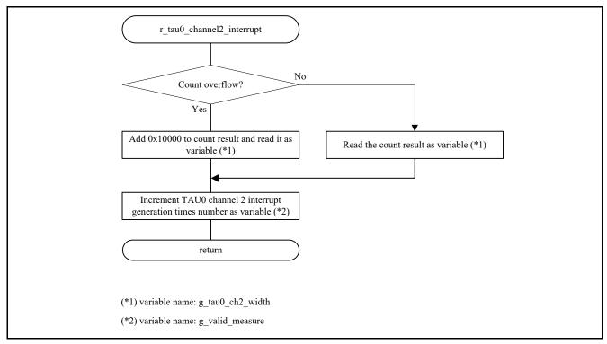
Figure 5.24 TAU channel 02 count complete interrupt function
