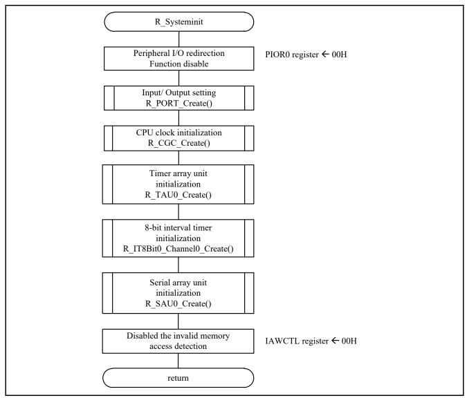
Figure 5.3 Peripheral function initialization function
