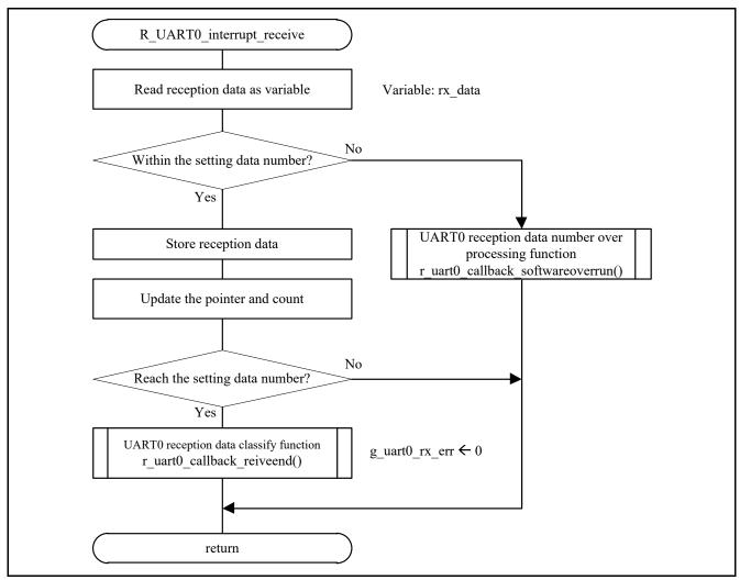
Figure 5.19 UART0 reception complete interrupt function
