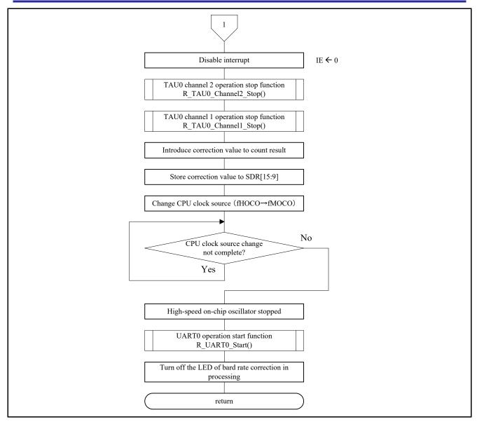
Figure 5.23 8-bit interval timer interrupt function (2/2)
