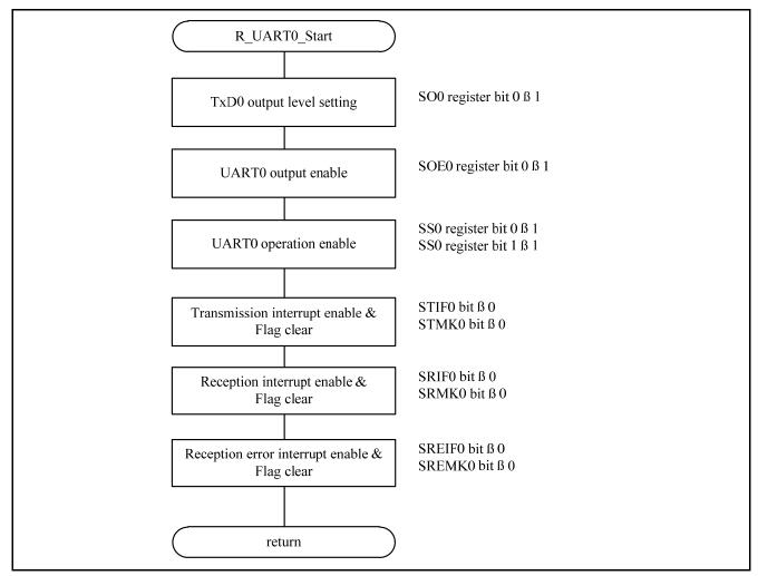
Figure 5.16 UART0 operation start function
