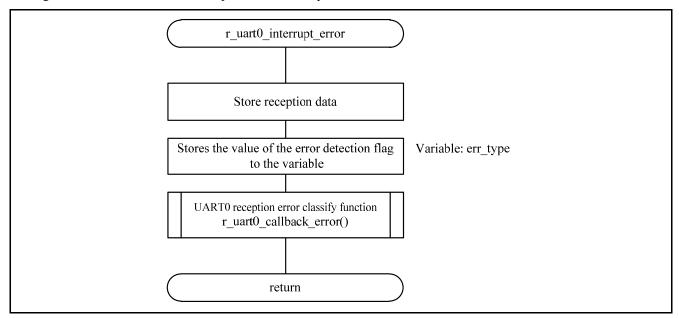
Figure 5.20 UART0 reception error interrupt function
