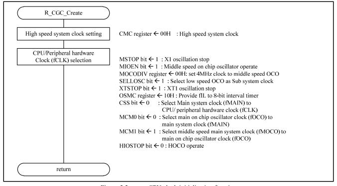
Figure 5.5 CPU clock initialization function
