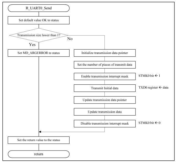
Figure 5.17 UART0 data transmission function
