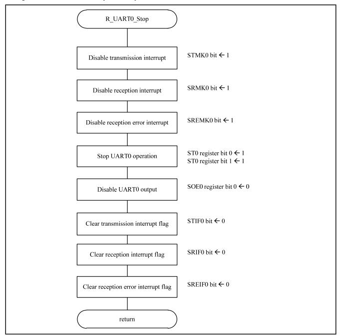
Figure 5.18 UART0 operation stop function
