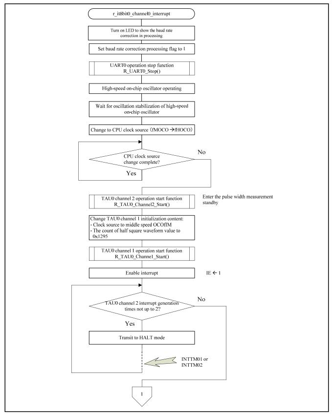
Figure 5.22 8-bit interval timer interrupt function (1/2)
