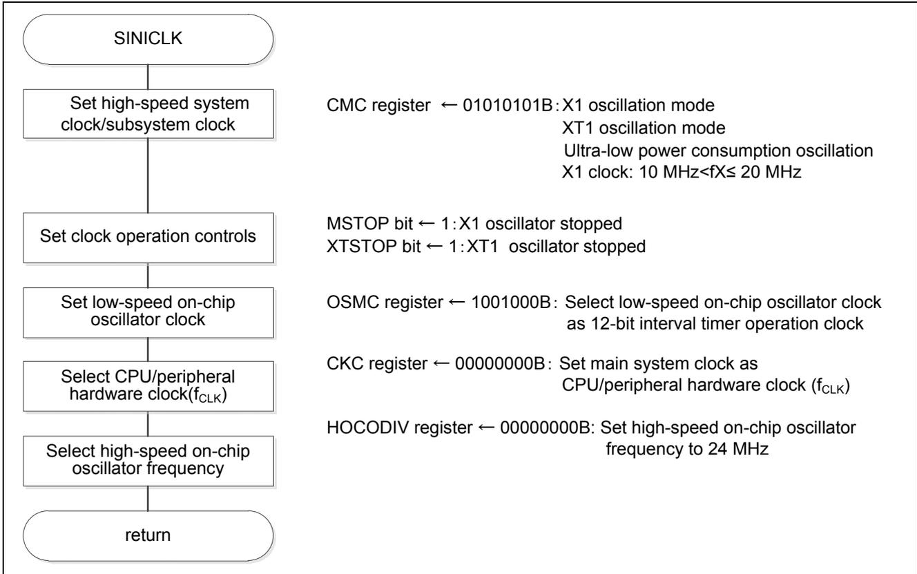
Figure 5.5 Clock Generator Setting
