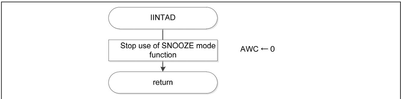
Figure 5.75 A/D Conversion Completion Interrupt Servicing
