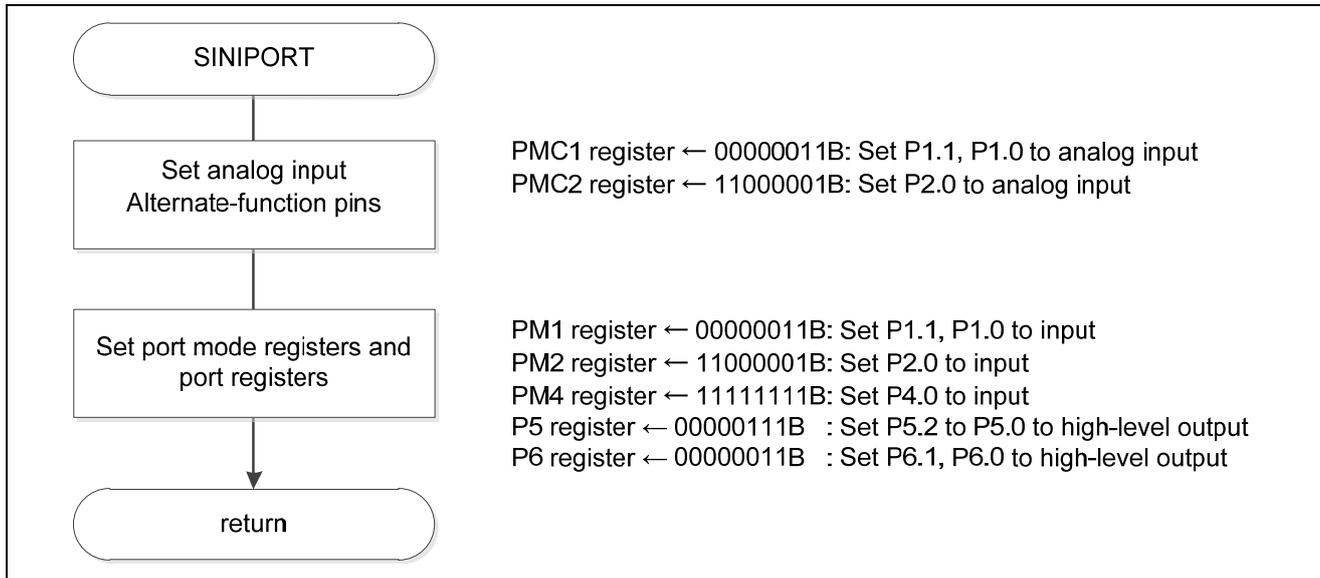
Figure 5.4 Input/Output Port Settings
