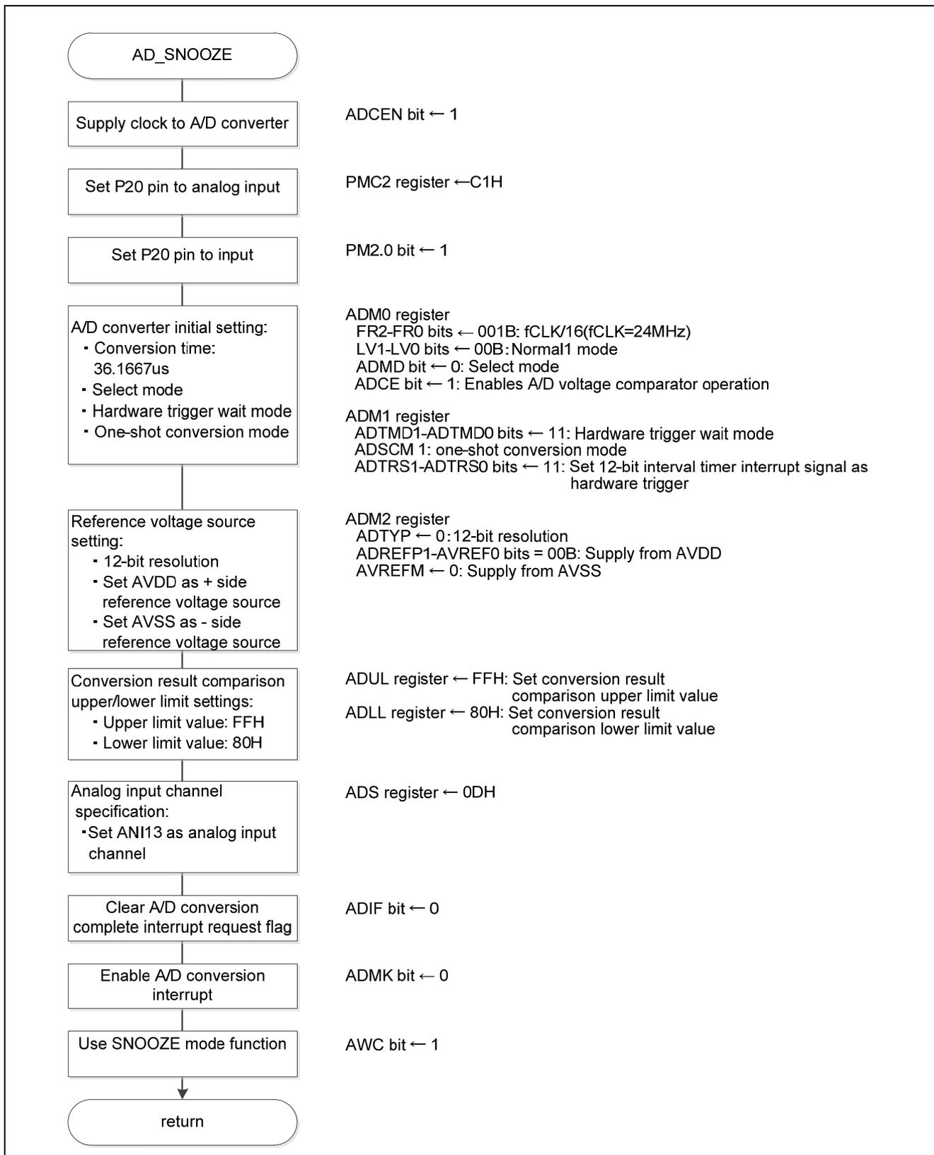
Figure 5.38 A/D Converter Setting
