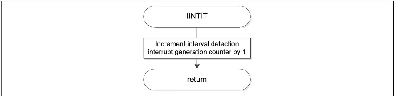
Figure 5.74 12-bit Interval Timer Interrupt Servicing
