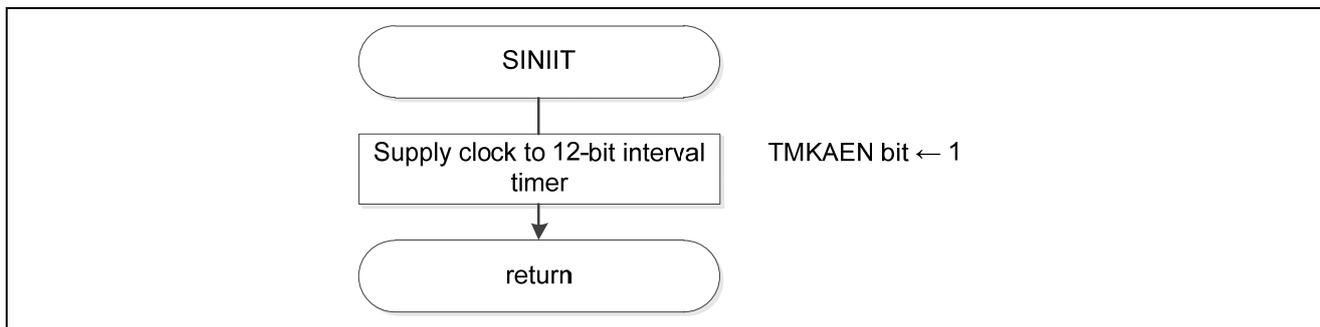
Figure 5.7 12-bit Interval Timer Setting
