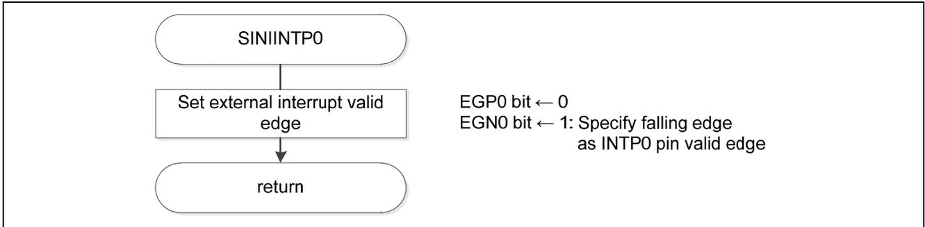
Figure 5.6 External Interrupt Setting
