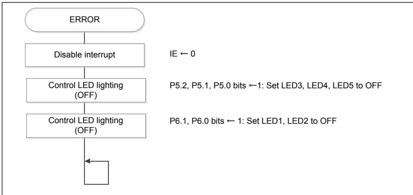
Figure 5.16 Error Processing of Status Transition
