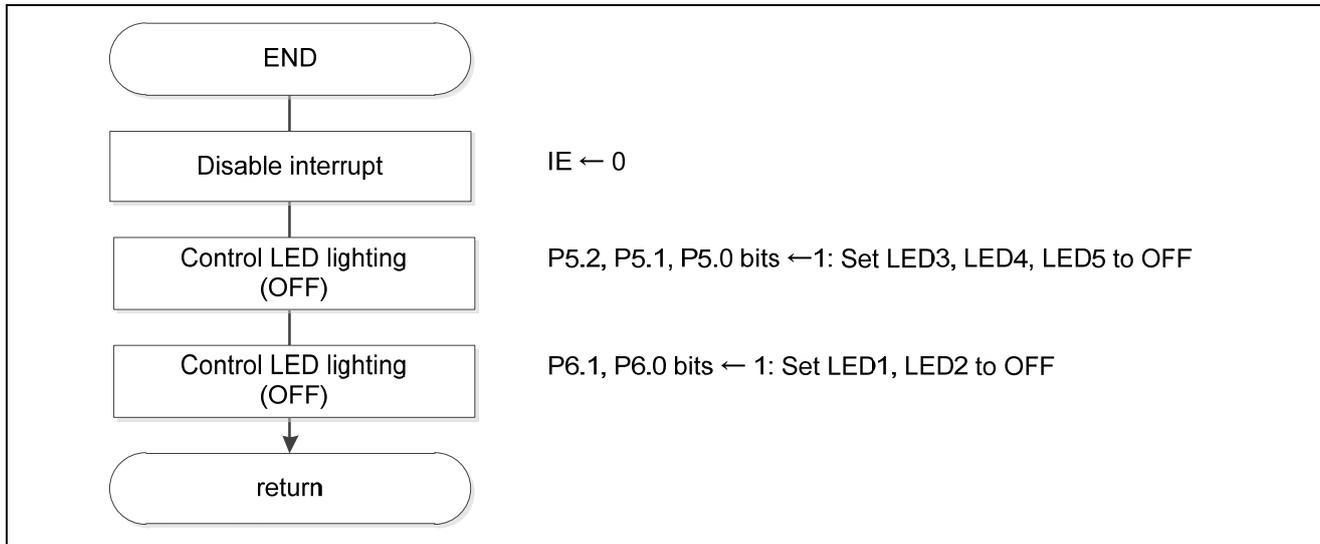
Figure 5.72 Status Transition End Processing
