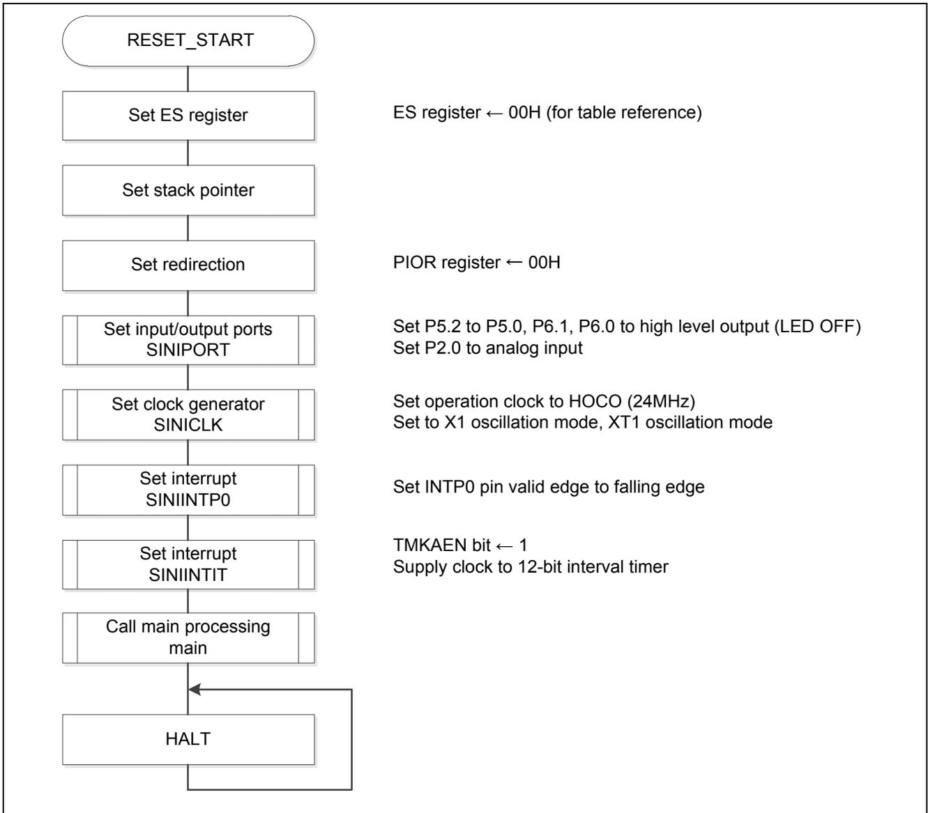
Figure 5.3 CPU Initialization Function
