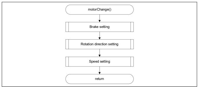
Figure 4-10 Flowchart of motorChange
