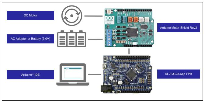
Figure 1-2 System configuration
