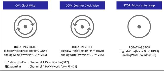
Figure 1-3 Motor shield control operation
