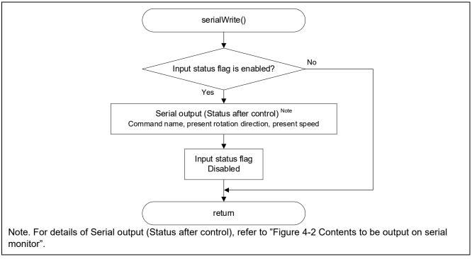
Figure 4-11 Flowchart of serialWrite
