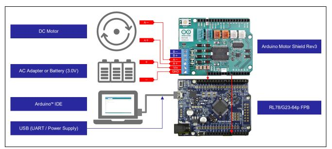
Figure 3-1 Connection of boards
