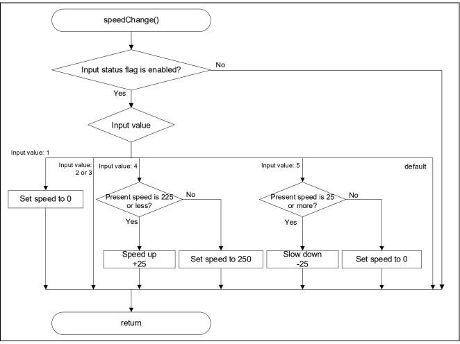
Figure 4-9 Flowchart of speedChange
