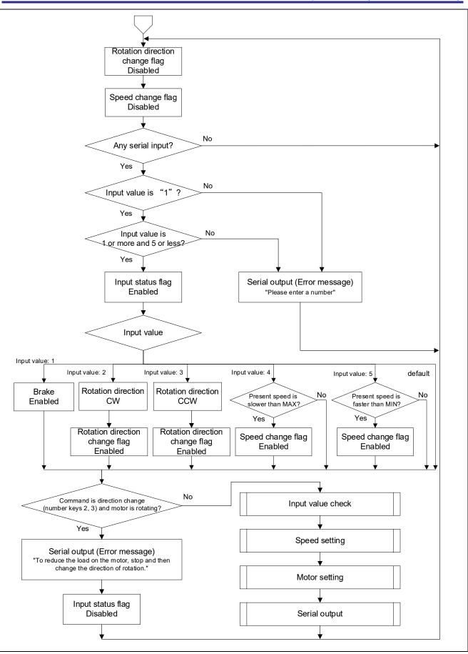
Figure 4-7 Flowchart of main processing
