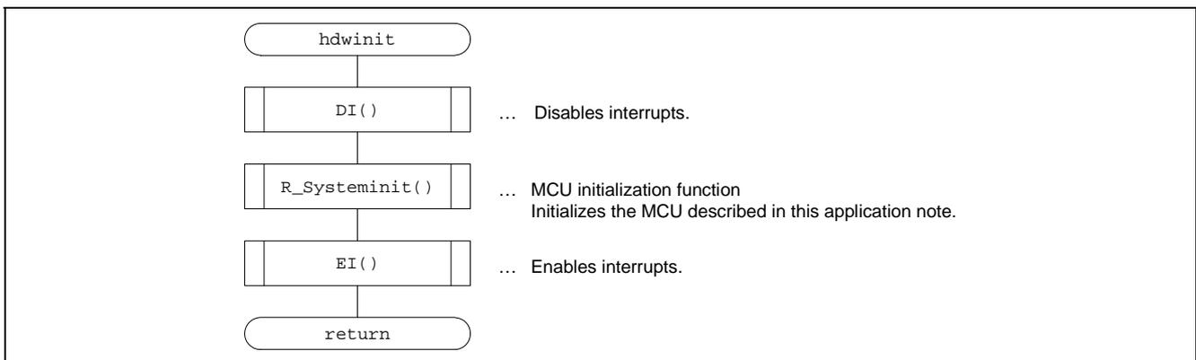
Figure 6.3 Flowchart for hdwinit Function
