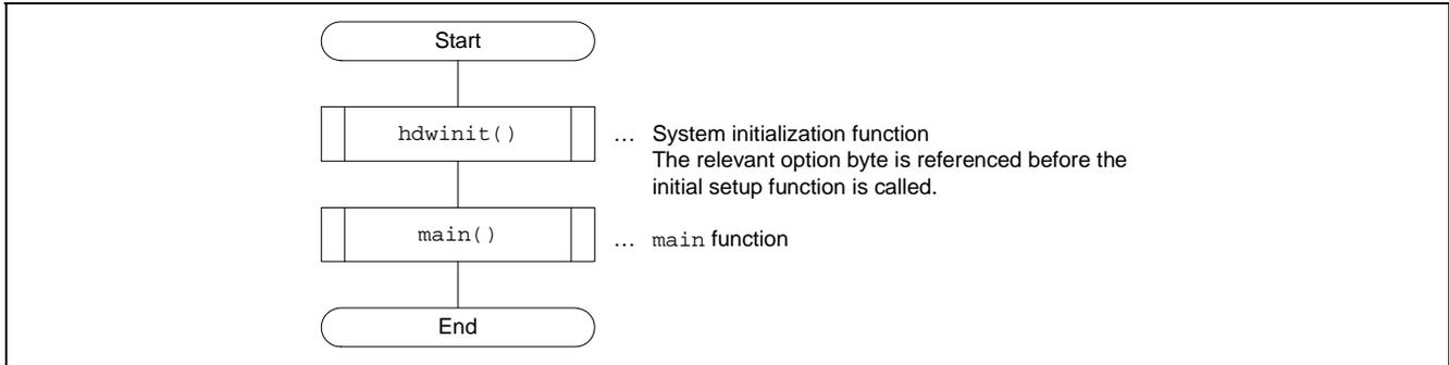
Figure 6.2 Overview of Processing Flow
