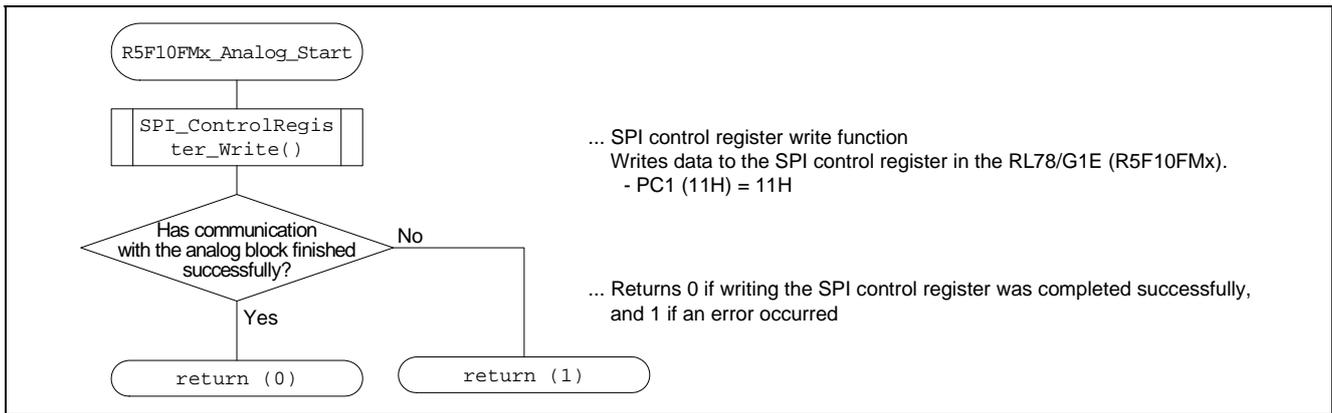
Figure 6.8 Flowchart for R5F10FMx\_Analog\_Start Function
