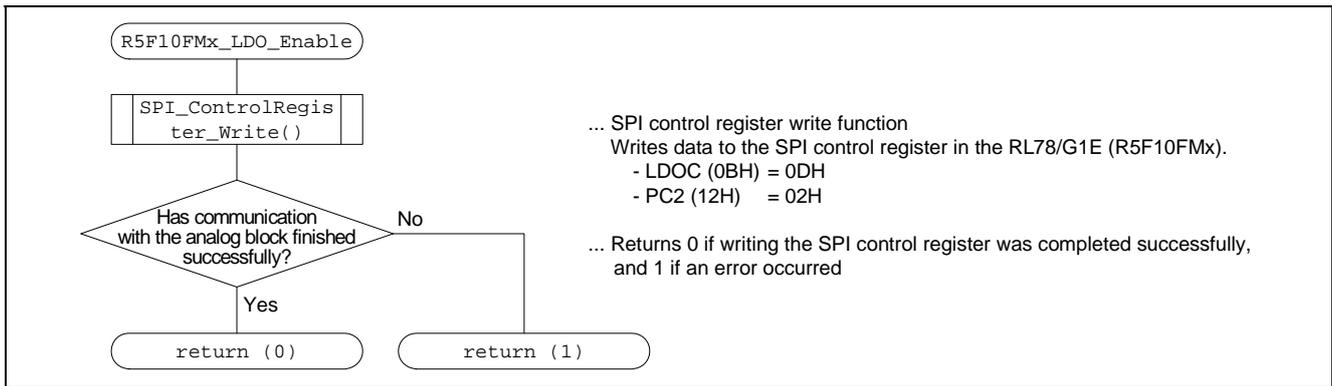
Figure 6.6 Flowchart for R5F10FMx\_LDO\_Enable Function
