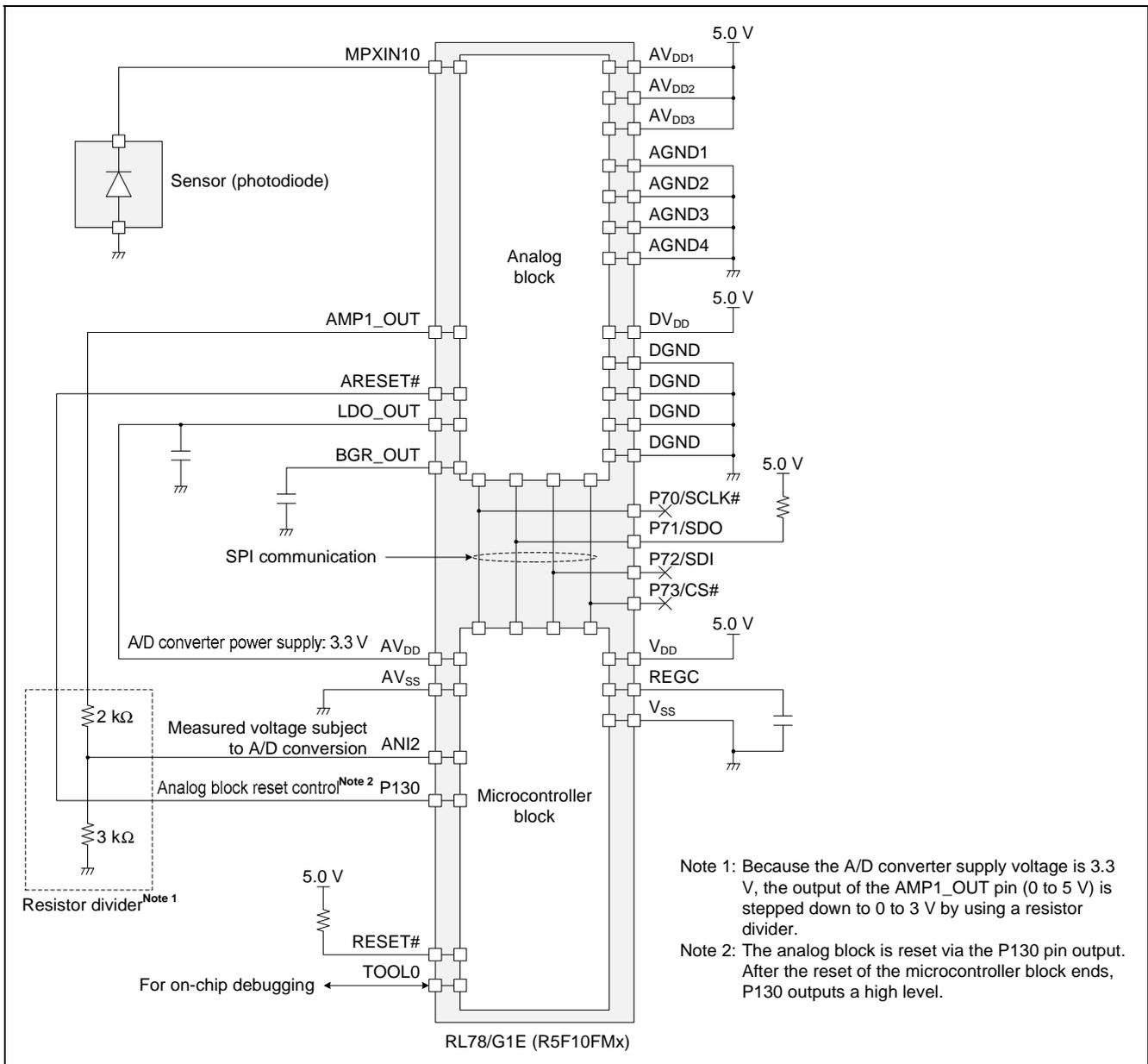
Figure 4.1 Hardware Configuration
