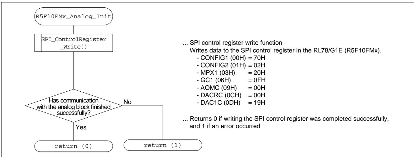
Figure 6.7 Flowchart for R5F10FMx\_Analog\_Init Function
