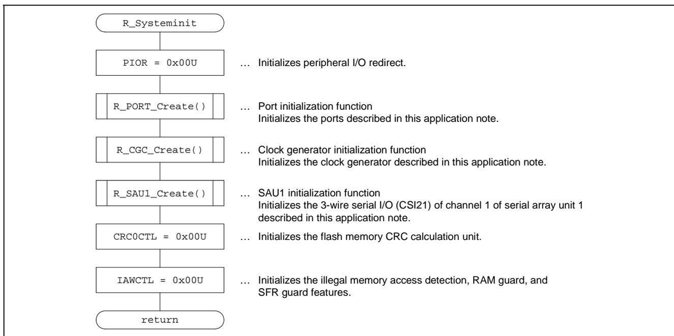
Figure 6.4 Flowchart for R\_Systeminit Function
