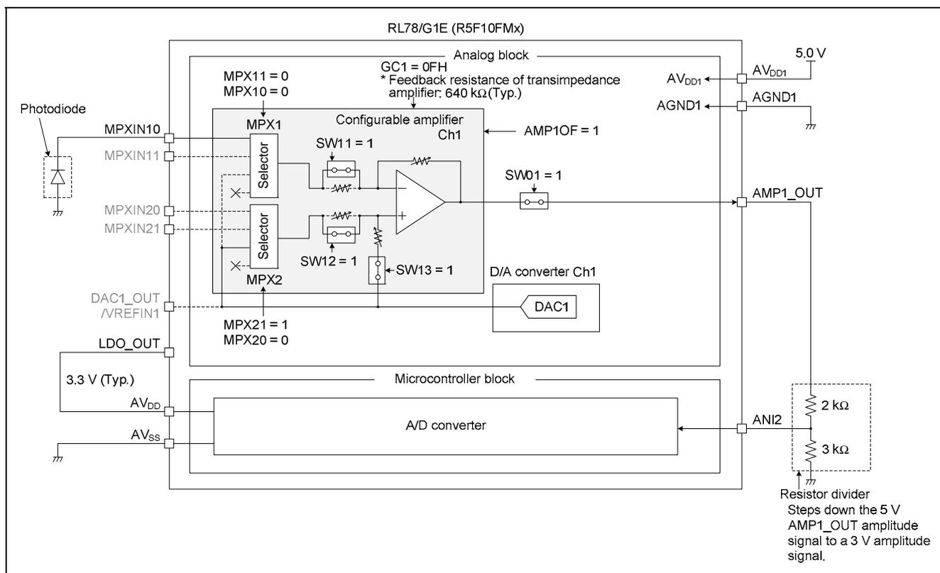
**Figure 5.2 Connection Between Configurable Amplifier Ch1 and Photodiode, and Between Configurable Amplifier Ch1 and A/D Converter**
