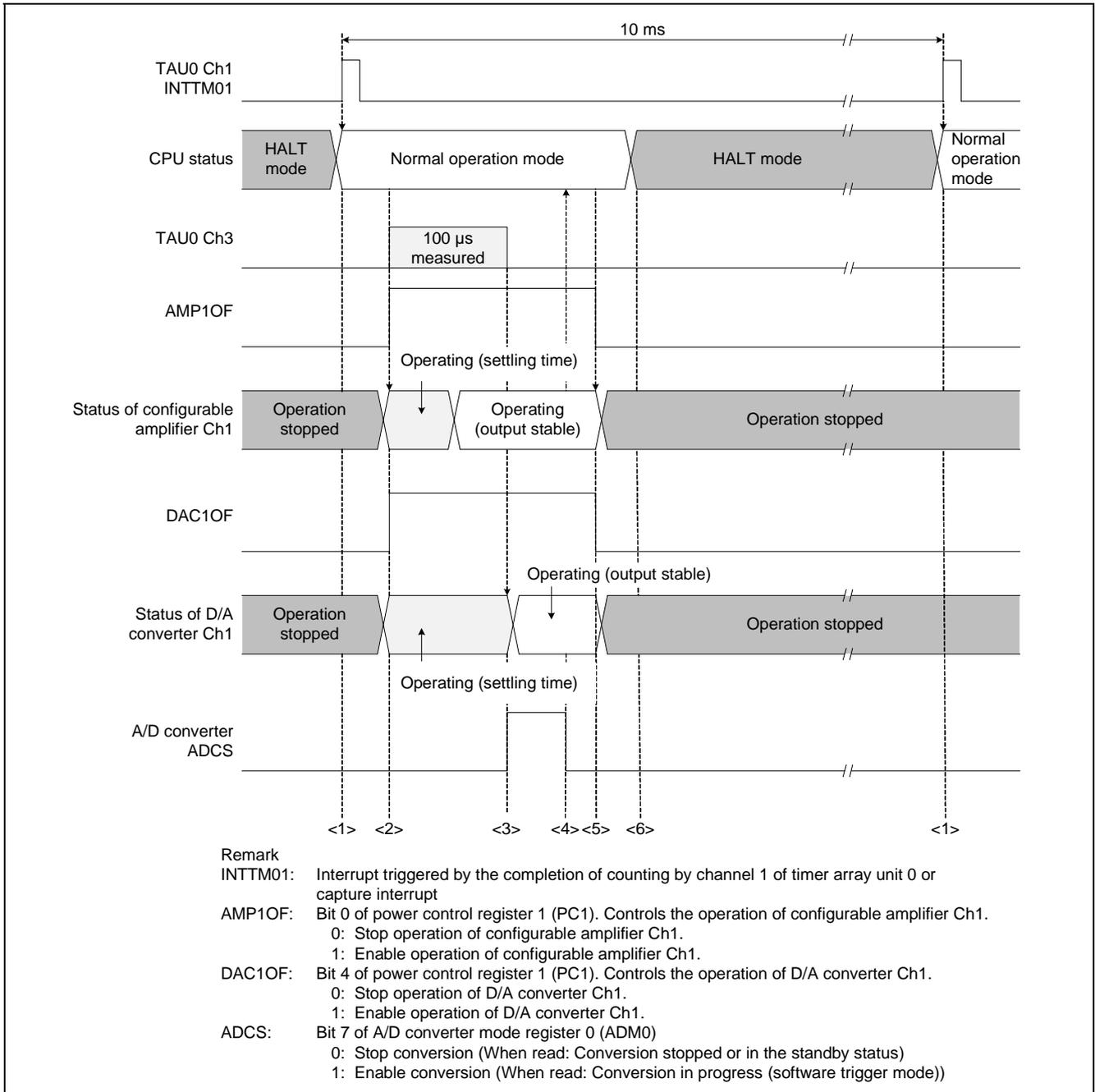
Figure 6.1 Timing Chart for Intermittent Operation
