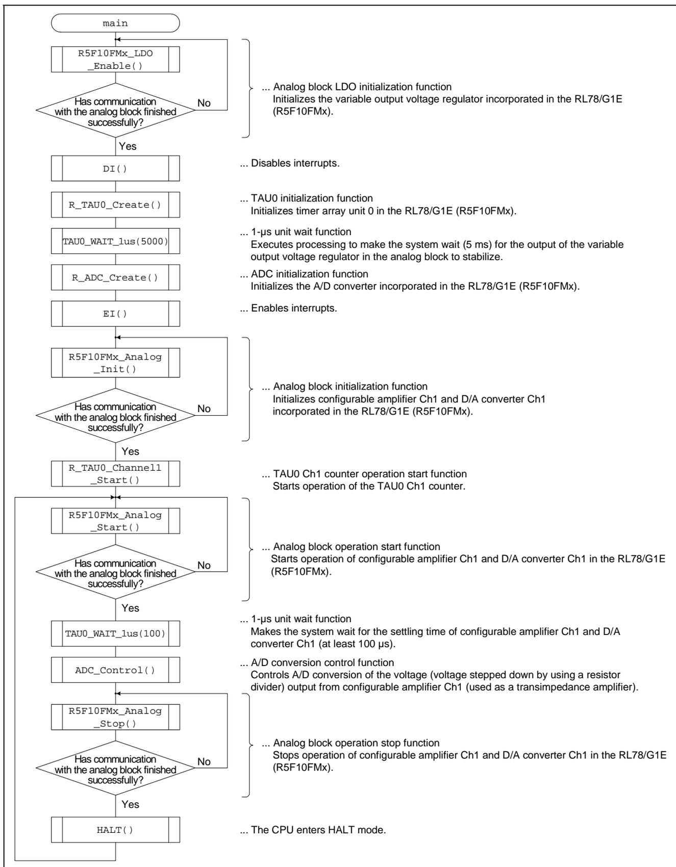
Figure 6.5 Flowchart for main Function
