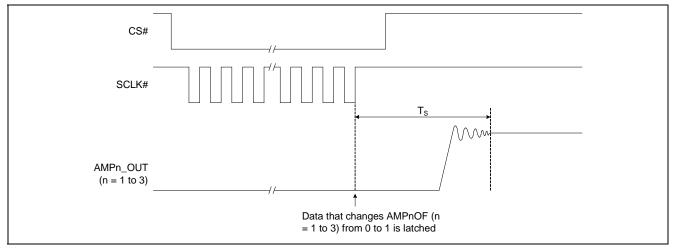
Figure 5.3 Settling Time of Configurable Amplifier (Used as Transimpedance Amplifier)
