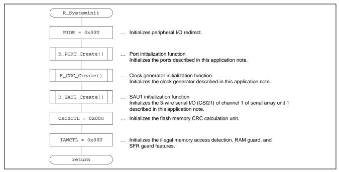
Figure 6.4 Flowchart for R\_Systeminit Function
