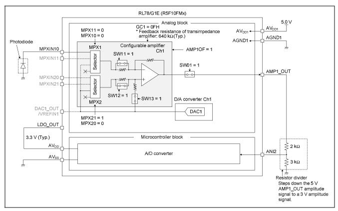
Figure 5.2 Connection Between Configurable Amplifier Ch1 and Photodiode, and Between Configurable Amplifier Ch1 and A/D Converter
