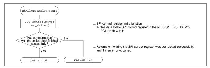
Figure 6.8 Flowchart for R5F10FMx\_Analog\_Start Function
