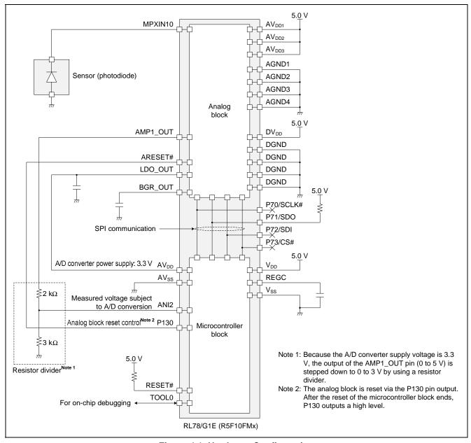
Figure 4.1 Hardware Configuration
