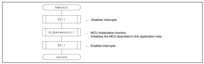
Figure 6.3 Flowchart for hdwinit Function
