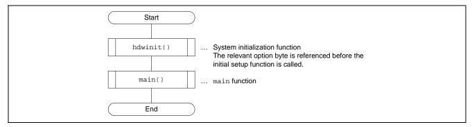
Figure 6.2 Overview of Processing Flow
