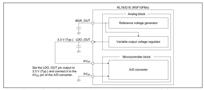
Figure 5.1 Connection Between Variable Output Voltage Regulator and A/D Converter
