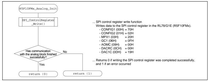
Figure 6.7 Flowchart for R5F10FMx\_Analog\_Init Function
