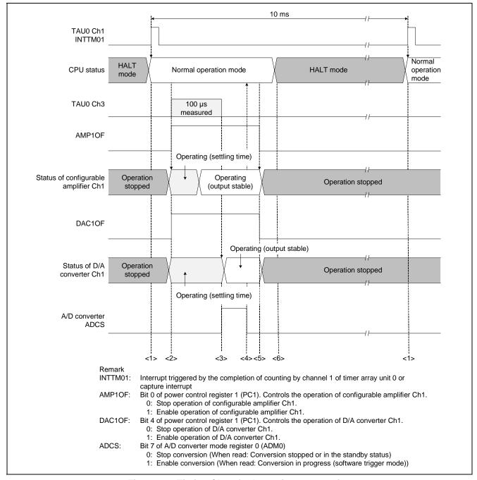
Figure 6.1 Timing Chart for Intermittent Operation
