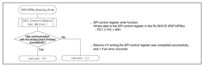
Figure 6.9 Flowchart for R5F10FMx\_Analog\_Stop Function
