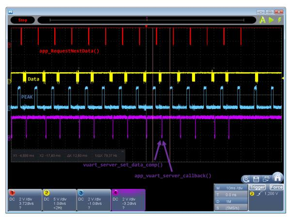
Figure 7: Oscillogram of continuous data transfer
