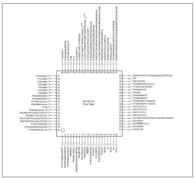
Figure 2.2 RL78/G14 (80-pin products) Pin Configuration
