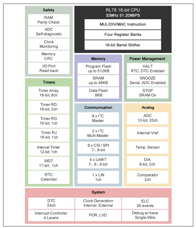
Figure 2.1 RL78/G14 Block Diagram
