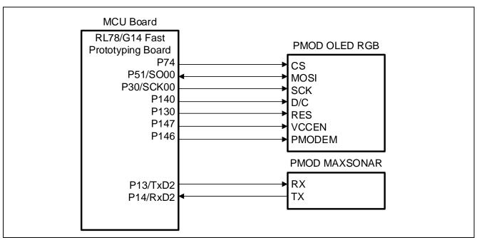
Figure 3.3 Connection of RL78/G14 FPB, PMOD OLED RGB and the Digilent PMOD MAXSONAR
