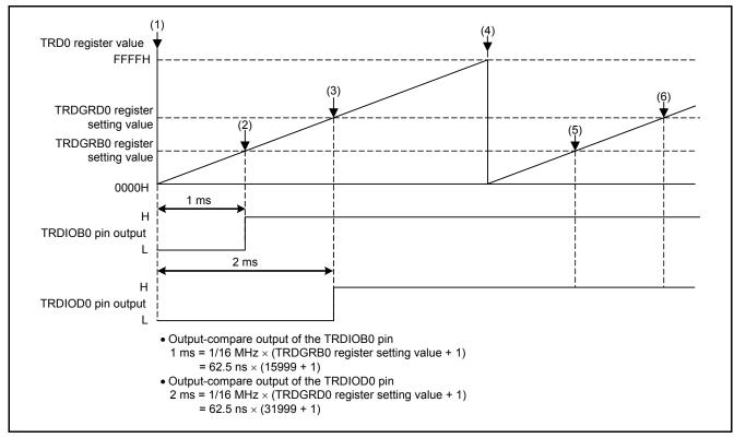
Figure 4.2 Operation Example of Output Compare
