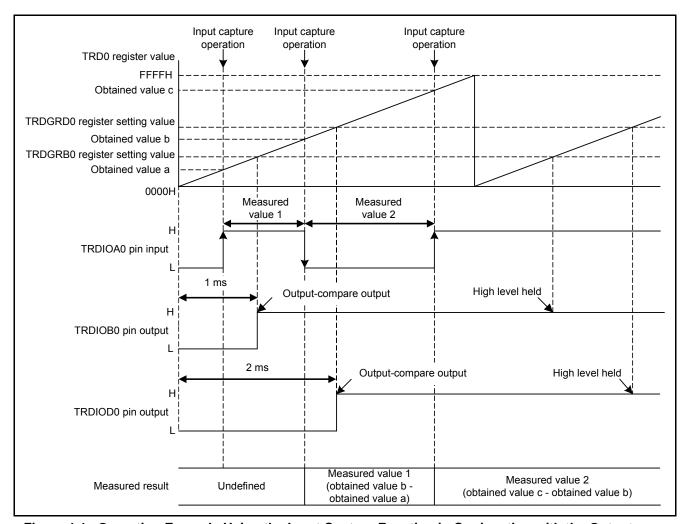
Figure 1.1 Operation Example Using the Input Capture Function in Conjunction with the Output Compare Function
