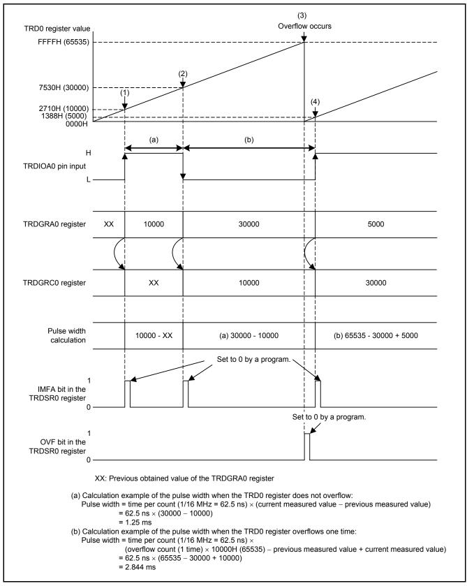
Figure 4.1 Operation Example of Input Capture
