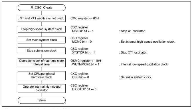
Figure 4.6 Initial Setting of the CPU
