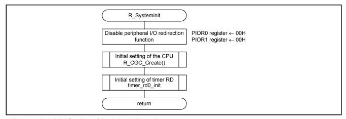
Figure 4.5 Initial Setting of Peripheral Functions
