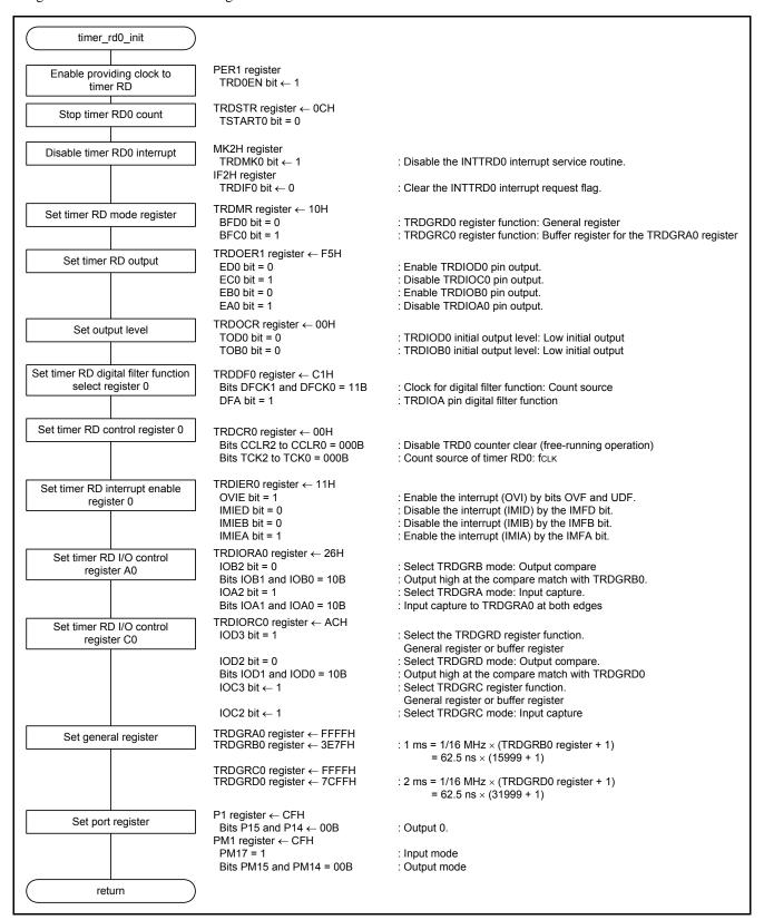
Figure 4.7 Initial Setting of Timer RD
