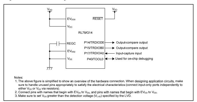
Figure 3.1 Hardware Configuration
