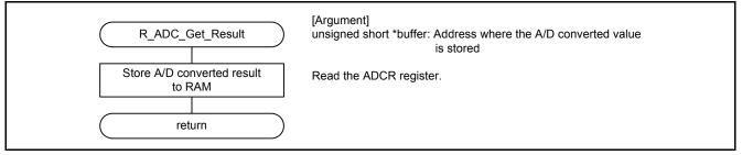
Figure 5.14 A/D Converted Result Obtained
