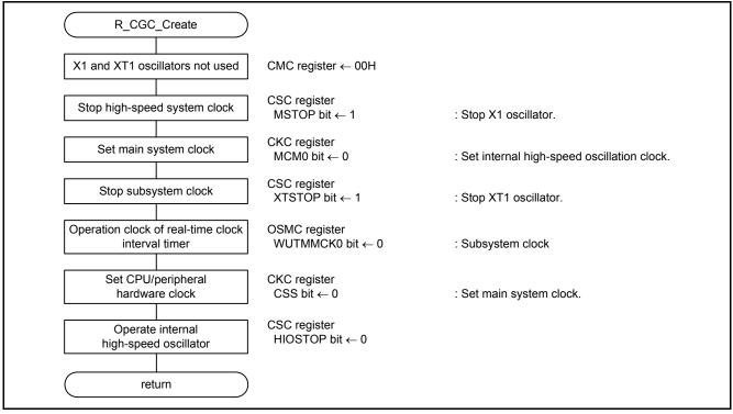
Figure 5.5 Initial Setting of the CPU
