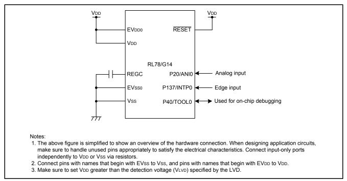
Figure 4.1 Hardware Configuration
