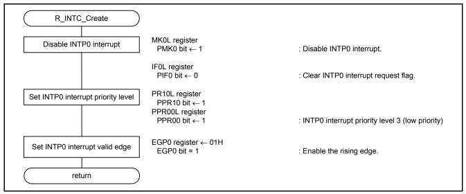
Figure 5.8 Initial Setting of INTP0
