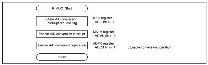
Figure 5.12 A/D Conversion Operation Enable Setting
