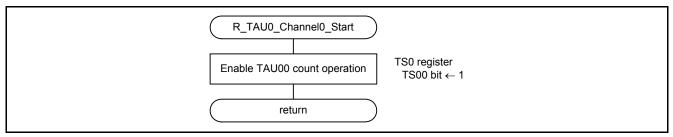
Figure 5.11 TAU00 Operation Enable Setting
