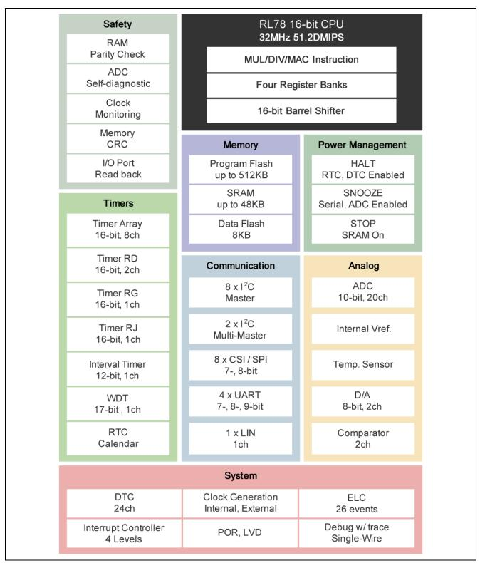
Figure 2.1 RL78/G14 Block Diagram
