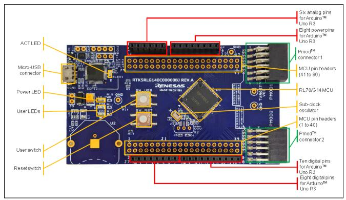
Figure 4.2 RL78/G14 FPB Board Layout (Top Side)
