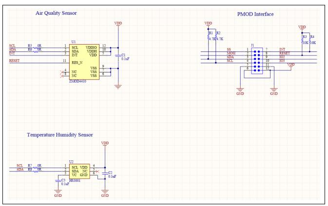
Figure 4.2 Sensor Board Circuit
