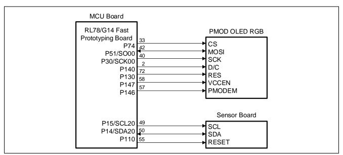
Figure 3.3 Connection of RL78/G14 FPB, PMOD OLED RGB and the Sensor Board
