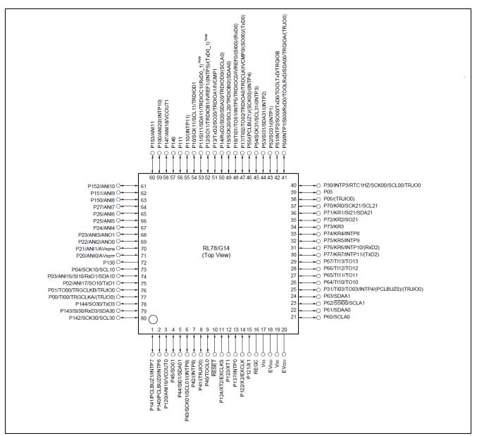
Figure 2.2 RL78/G14 (80-pin products) Pin Configuration
