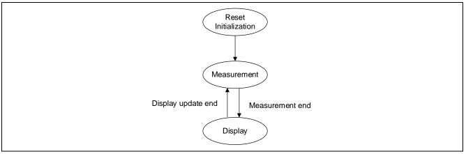
Figure 5.1 Tasks Transition Block Diagram
