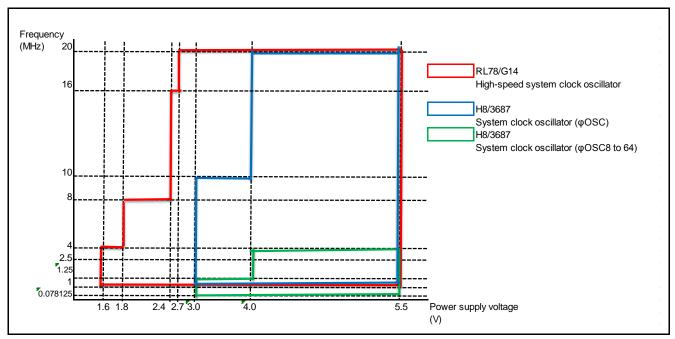
Figure 1.1 Comparison of Operating Frequencies of System Clock Oscillators
