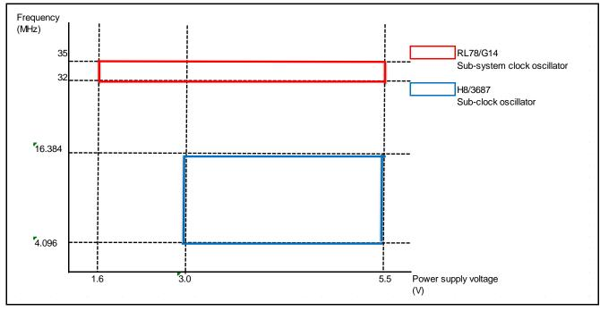
Figure 1.3 Comparison of Operating Frequencies of XCIN Clock Oscillators
