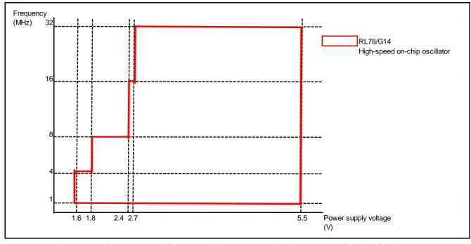
Figure 1.2 Comparison of Operating Frequencies of the High-speed On-chip Oscillator
