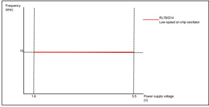
Figure 1.4 Comparison of Operating Frequencies of the Low-speed On-chip Oscillator
