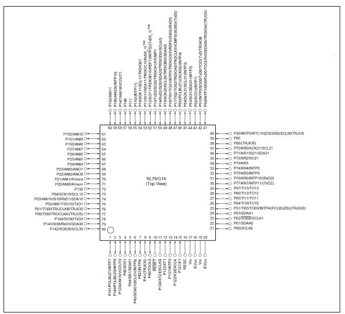
Figure 2.2 RL78/G14 (80-pin products) Pin Configuration
