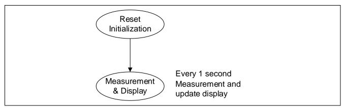
Figure 5.1 Tasks Transition Block Diagram
