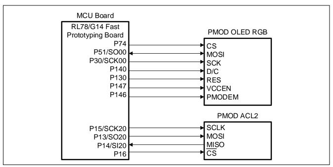
Figure 3.3 Connection of RL78/G14 FPB, PMOD OLED RGB and the Digilent PMOD ACL2
