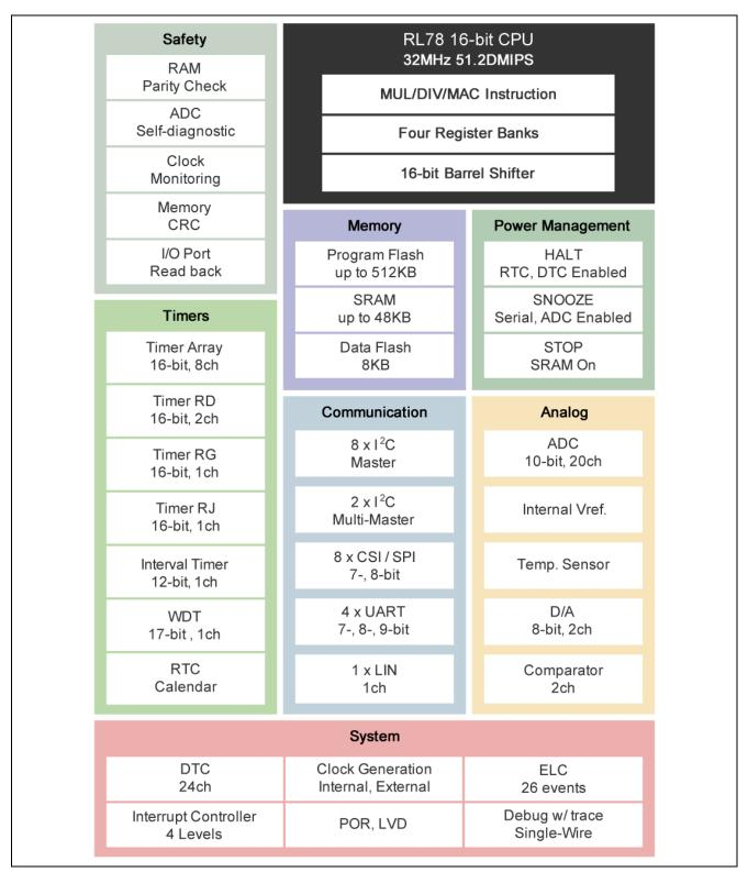
Figure 2.1 RL78/G14 Block Diagram
