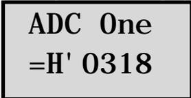
3. Adjust the setting of the potentiometer, press SW1 to observe the change in the value.
