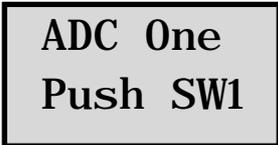
2. Observe the LCD display — the RL78G13 will make an ADC reading of the potentiometer, RV1, after pressing SW1 and display the 10-bit value on the LCD.
