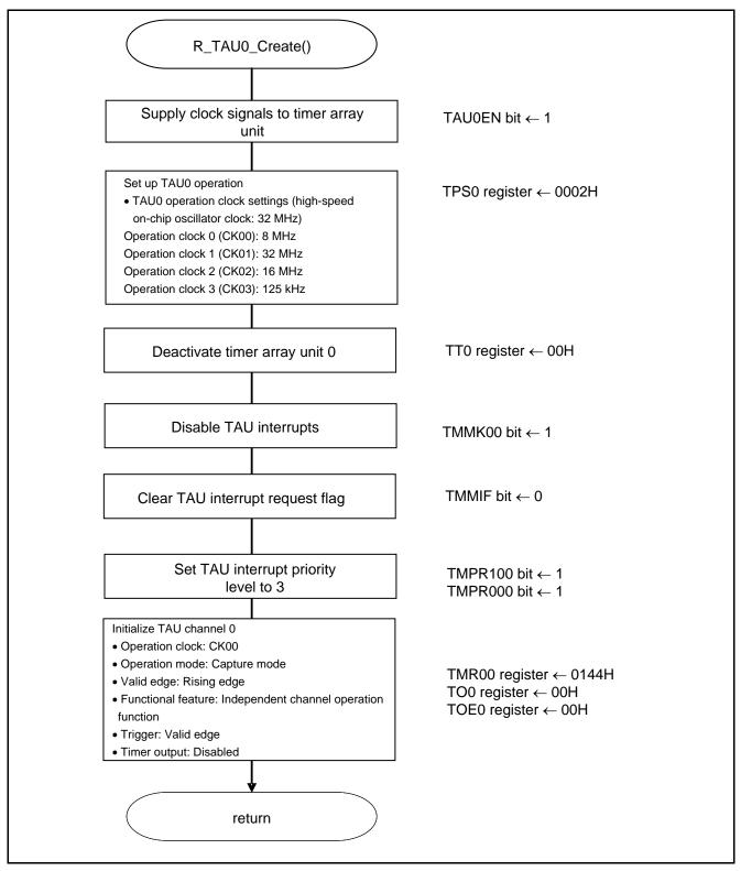
Figure 5.6 Timer Array Unit Setup
