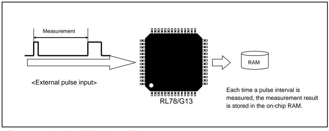
Figure 1.1 Overview of Pulse Interval Measurement
