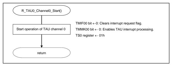
Figure 5.8 **Timer Array Unit Startup**
