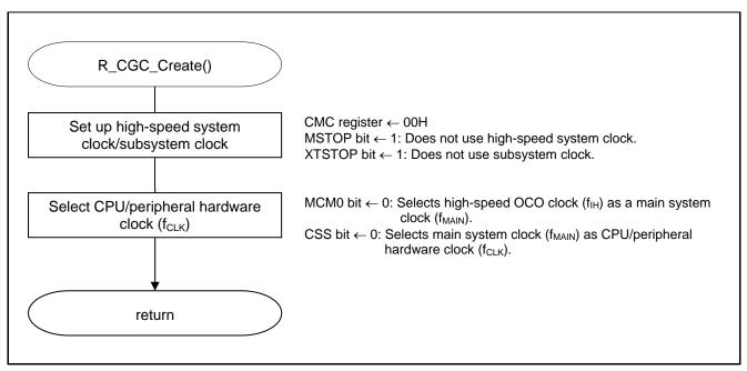
Figure 5.5 CPU Clock Setup
