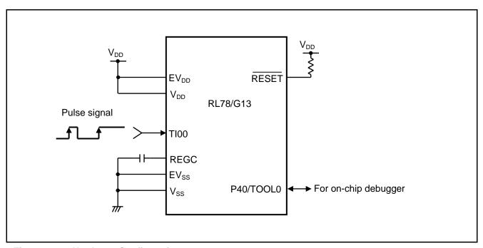
Figure 4.1 **Hardware Configuration**
