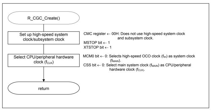
Figure 5.5 CPU Clock Setup
