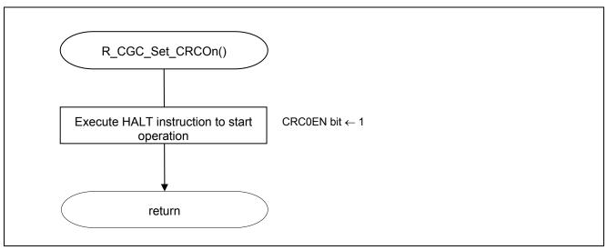
Figure 5.10 Enabling High-speed CRC Operation
