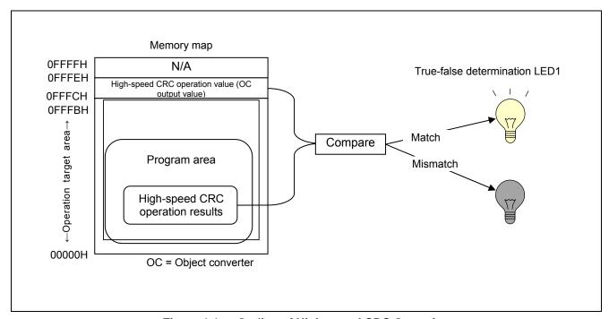
Figure 1.1 **Outline of High-speed CRC Operation**
