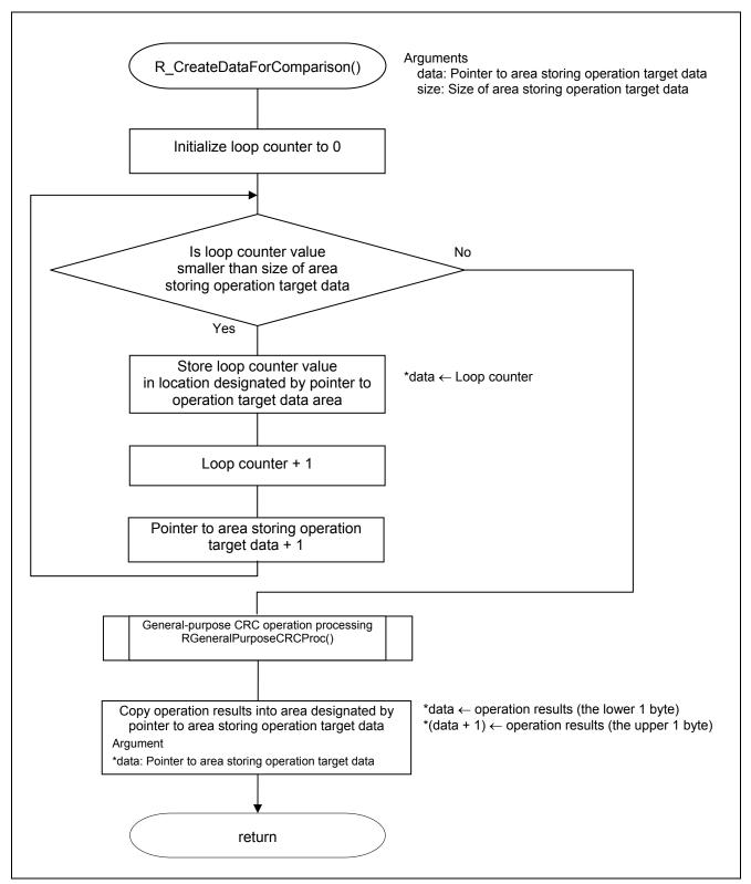
Figure 5.12 Creating General-purpose CRC Operation Target Data
