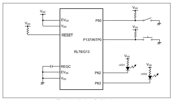
Figure 4.1 Hardware Configuration
