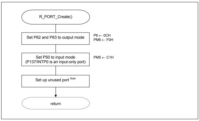
Figure 5.4 I/O Port Setup
