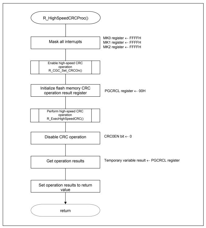
Figure 5.9 High-speed CRC Operation Processing
