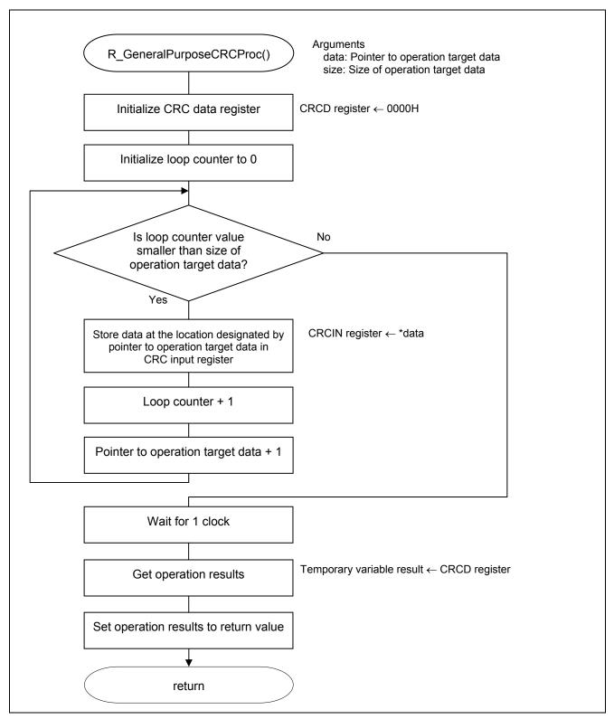
Figure 5.13 General-purpose CRC Operation Processing
