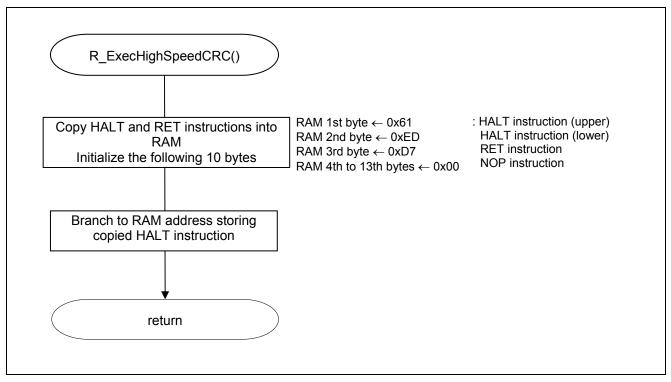
Figure 5.11 Performing High-speed CRC Operation
