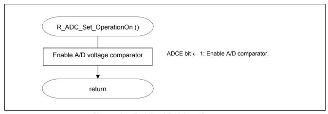
Figure 5.8 Enabling A/D Voltage Comparator
