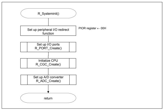
Figure 5.3 System Initialization Function
