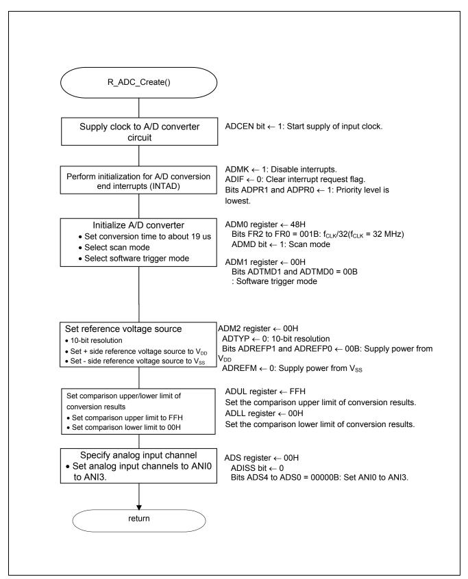
Figure 5.6 A/D Converter Setup
