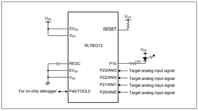
Figure 4.1 Hardware Configuration
