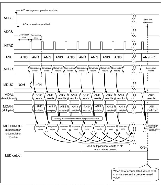
Figure 1.2 Outline of Multiplication-Accumulation Operation
