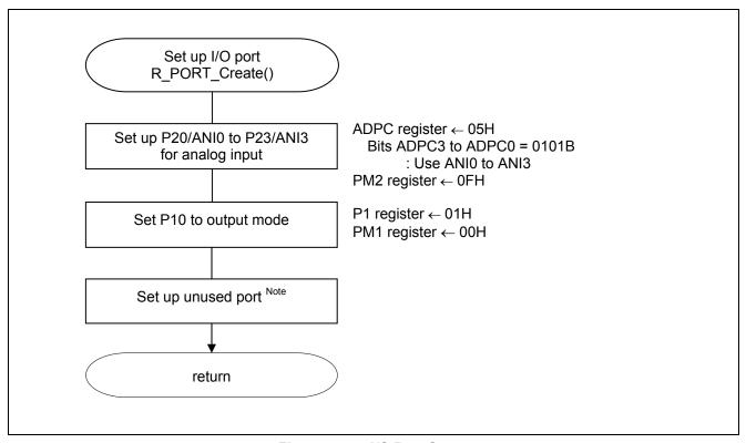
Figure 5.4 I/O Port Setup
