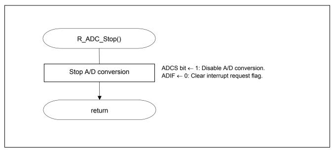
Figure 5.11 Stopping A/D Conversion
