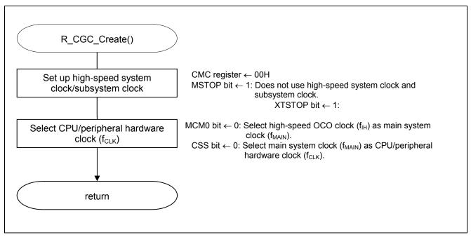
Figure 5.5 CPU Clock Setup
