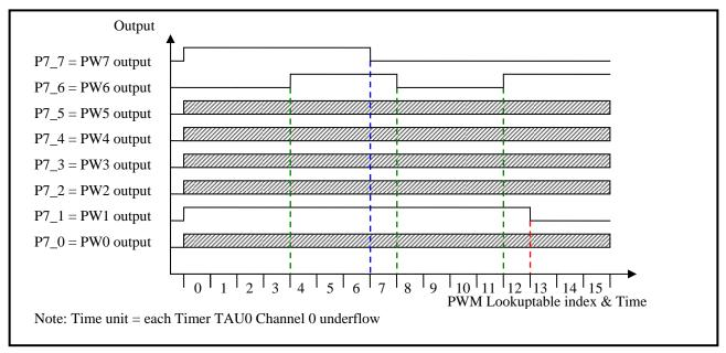
Figure 2 Port output states & PWM Look-up table relationship during DMA transfers
