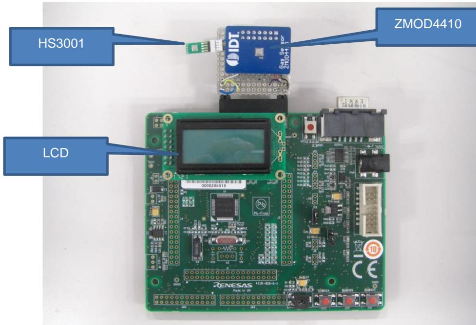
Figure 2.1 Example of connection between RSK and sensor modules
