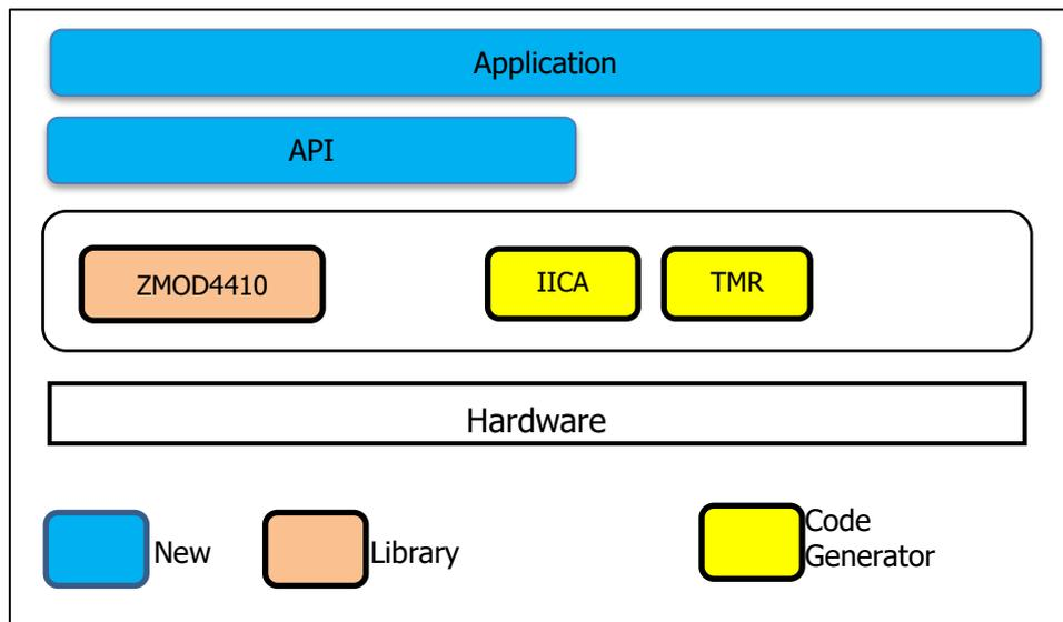
Figure 5.1 Software Structure
