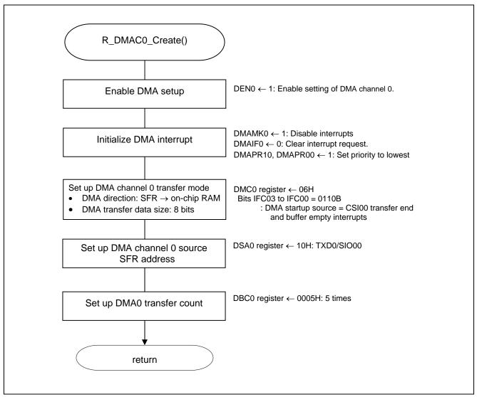
Figure 5.8 DMA Controller Initialization
