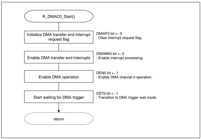
Figure 5.12 DMA Transfer Enable Processing
