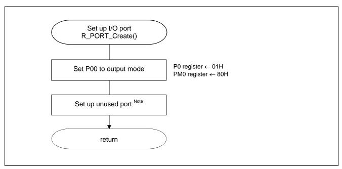
Figure 5.4 I/O Port Setup
