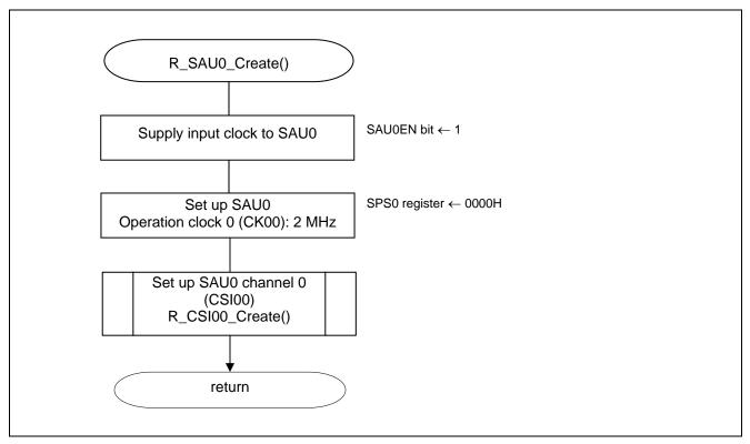
Figure 5.6 Serial Array Unit 0 Setup
