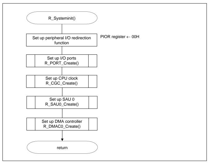
Figure 5.3 System Initialization Function
