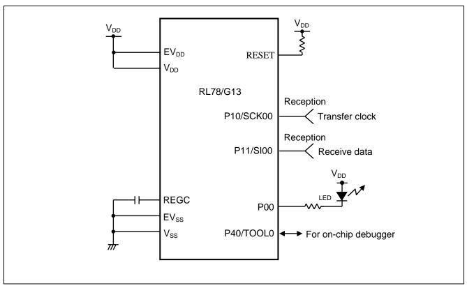
Figure 4.1 Hardware Configuration
