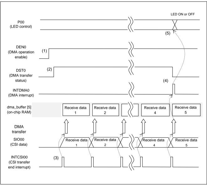
Figure 1.2 DMA Controller Timing Chart
