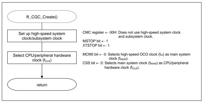
Figure 5.5 CPU Clock Setup
