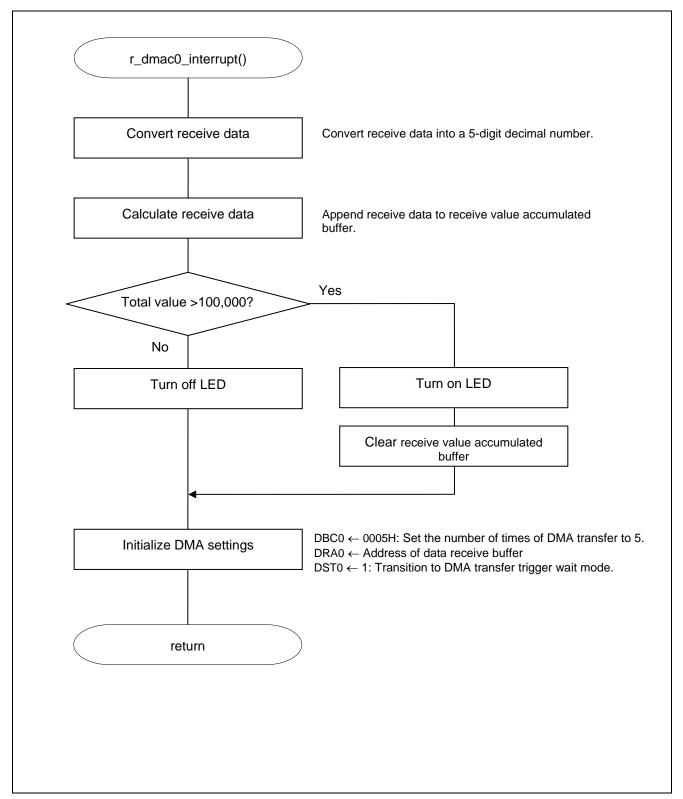
Figure 5.13 DMA Transfer End Interrupt Processing
