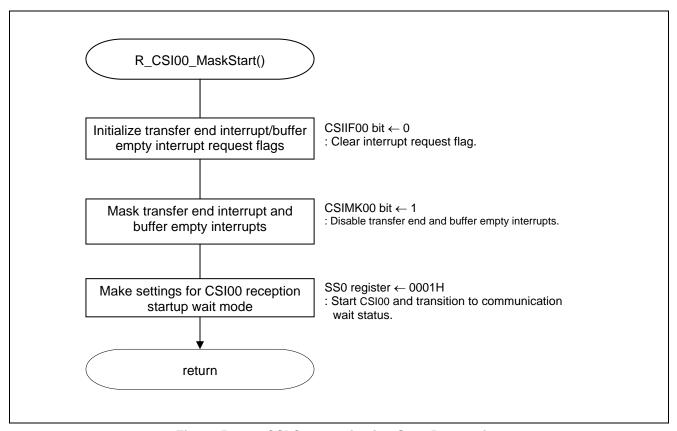
Figure 5.11 CSI Communication Start Processing
