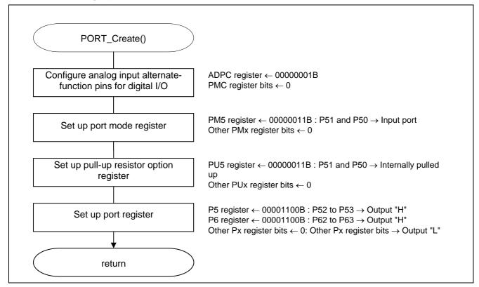
Figure 5.4 I/O Port Setup
