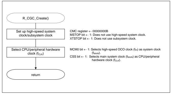
Figure 5.5 CPU Clock Setup
