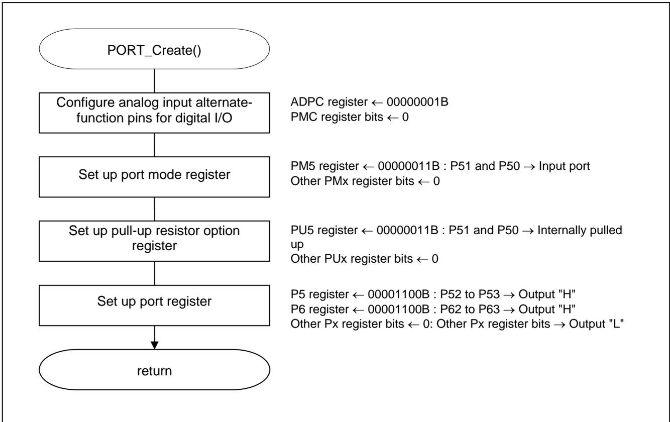
Figure 4.4 I/O Port Setup
