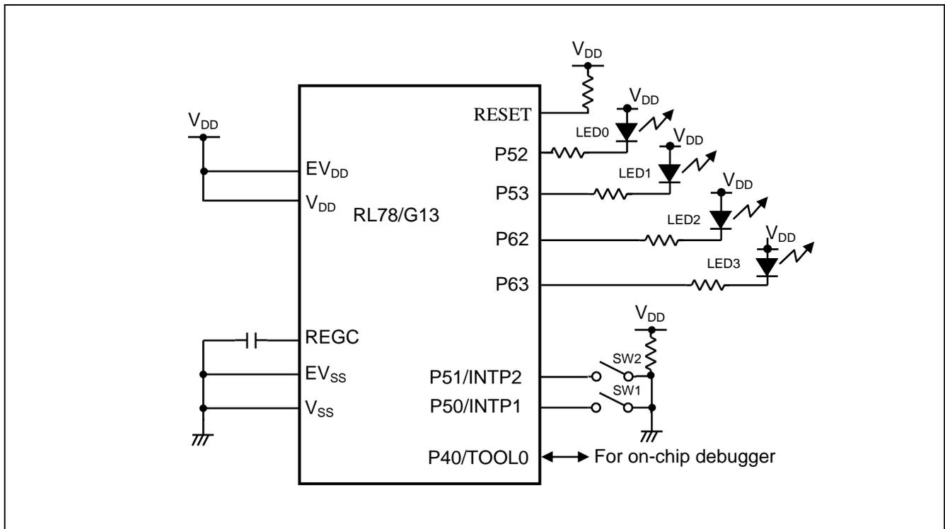
**Figure 4.1 Hardware Configuration**
