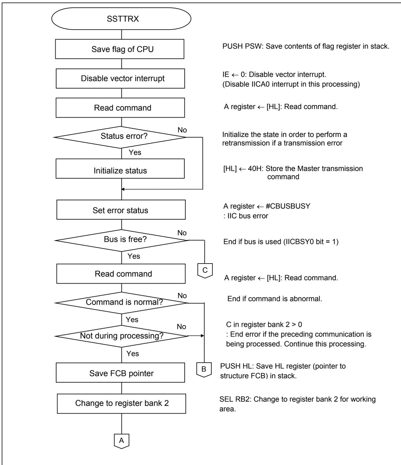
Figure 5.10 Master Transmission Start Processing (1/2)
