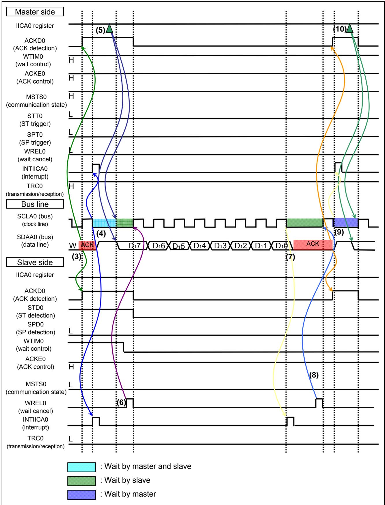
Figure 1.3 IIC Communication Timing Chart (Master-to-Slave Communication Example) (2/4)
