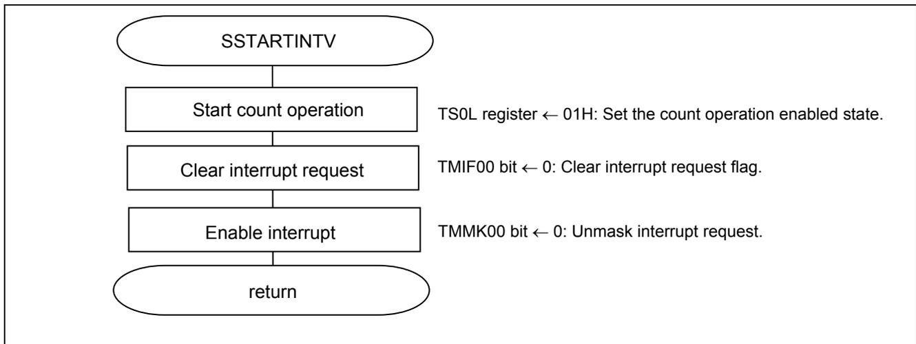
**Figure 5.9 Startup of 10-ms interval timer**
