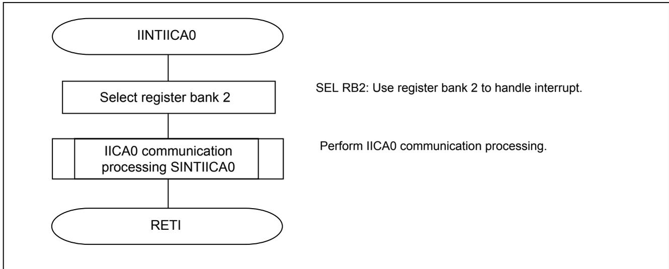
**Figure 5.14 IICA0 Interrupt Processing**
