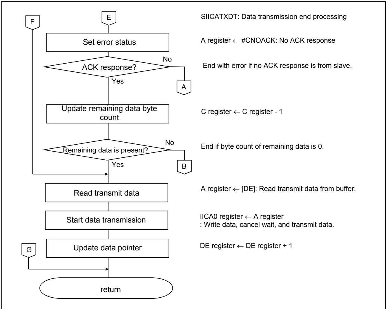
Figure 5.17 IICA0 Master Communication Processing (3/3)
