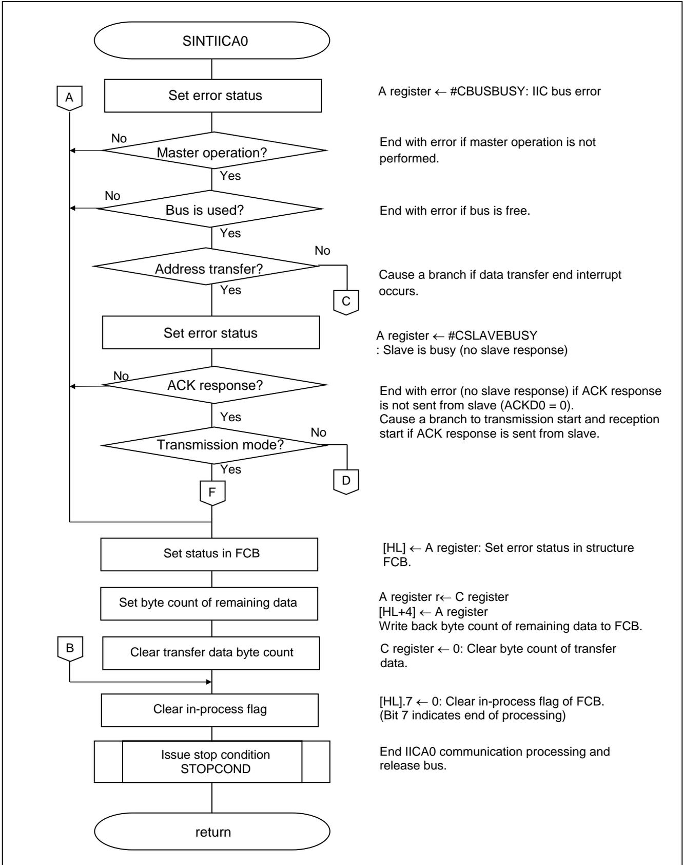
Figure 5.15 IICA0 Master Communication Processing (1/3)
