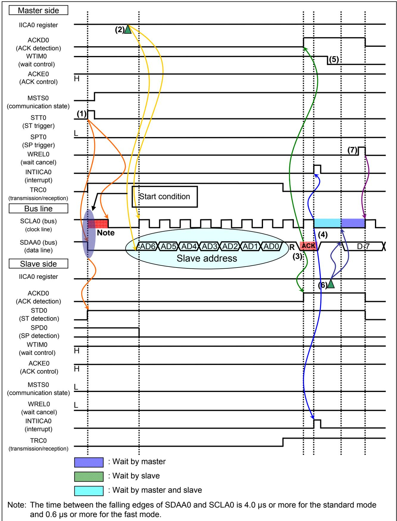
Figure 1.6 IIC Communication Timing Chart (Slave-to-Master Communication Example) (1/3)
