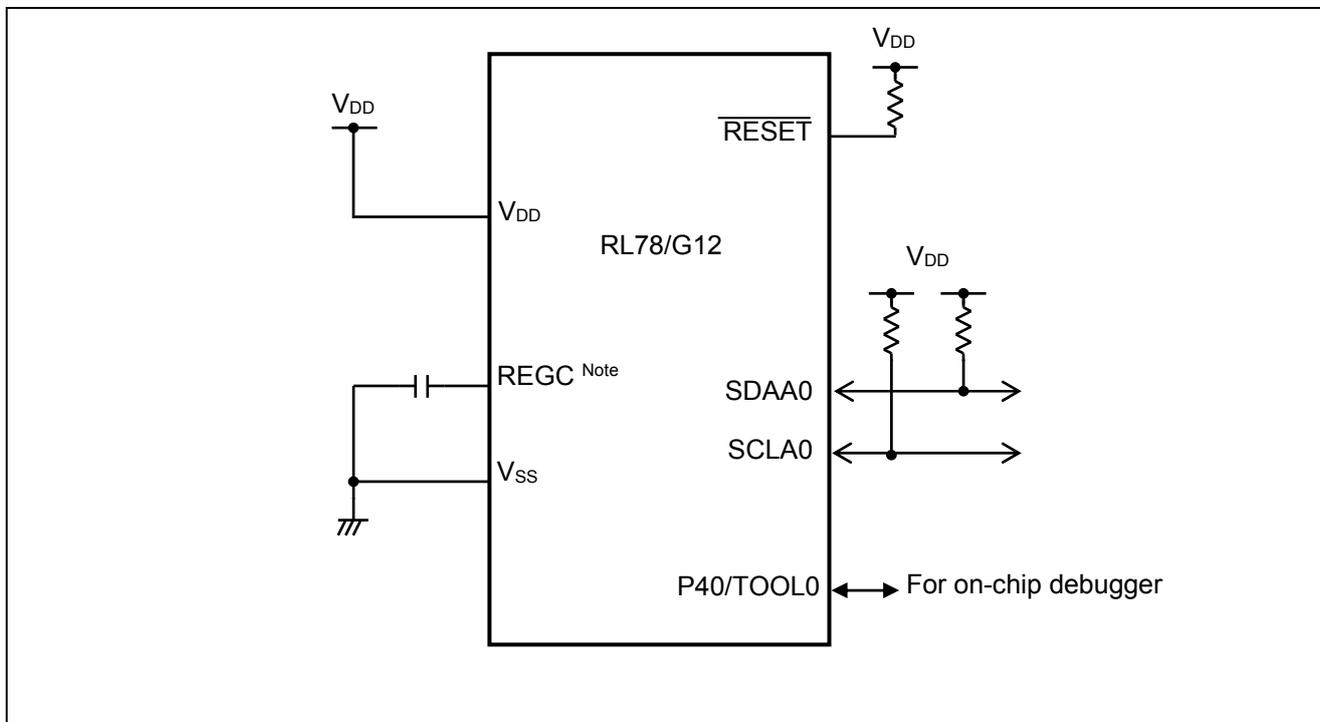
**Figure 4.1 Hardware Configuration**
