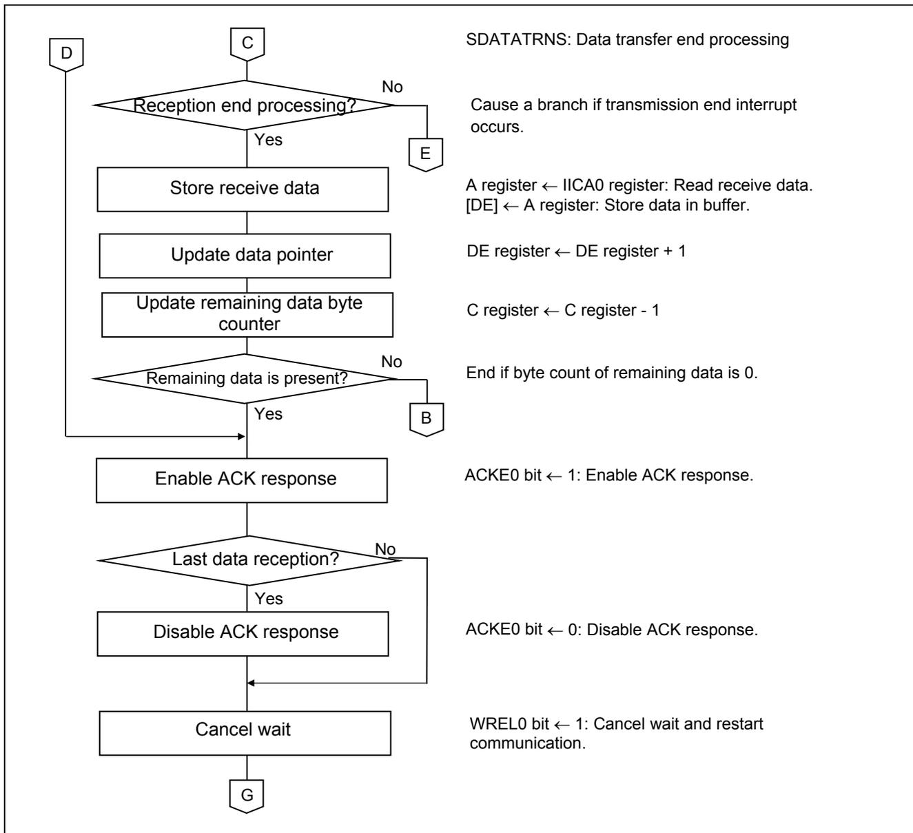
Figure 5.16 IICA0 Master Communication Processing (2/3)
