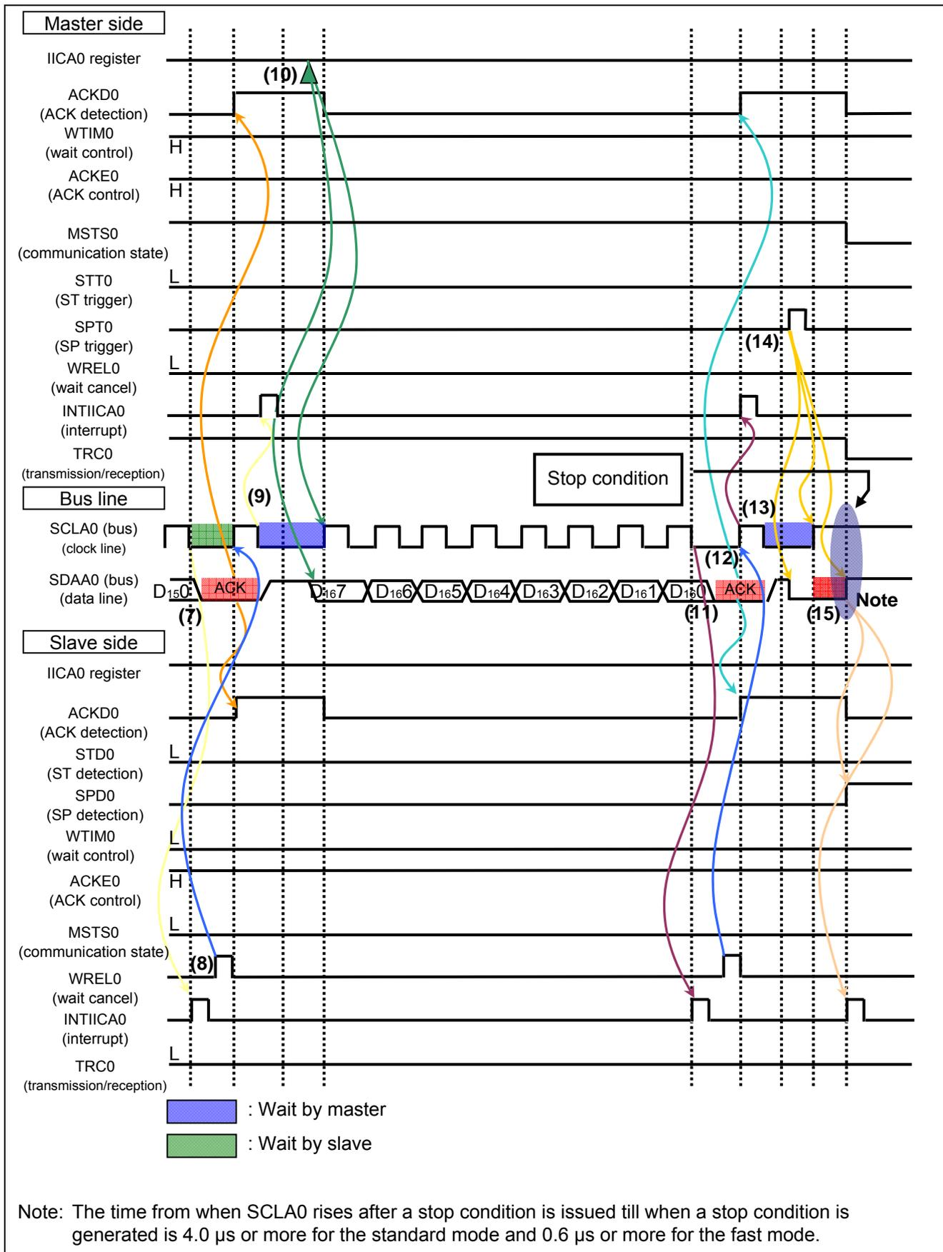
Figure 1.4 IIC Communication Timing Chart (Master-to-Slave Communication Example) (3/4)
