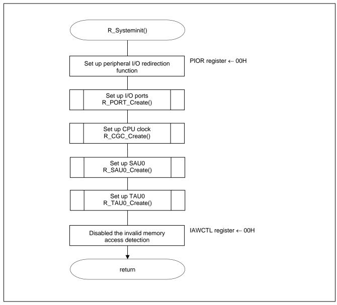
Figure 5.3 System Initialization Function
