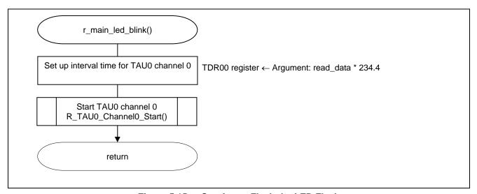
Figure 5.15 Starting to Flash the LED Flash
