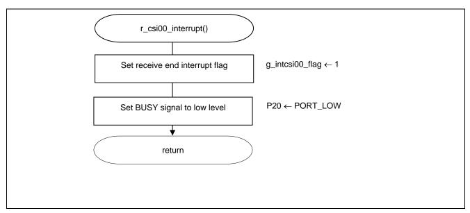
Figure 5.14 CSI00 Receive End Interrupt
