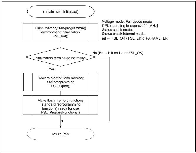
Figure 5.24 Flash Memory Self-Programming Initialization
