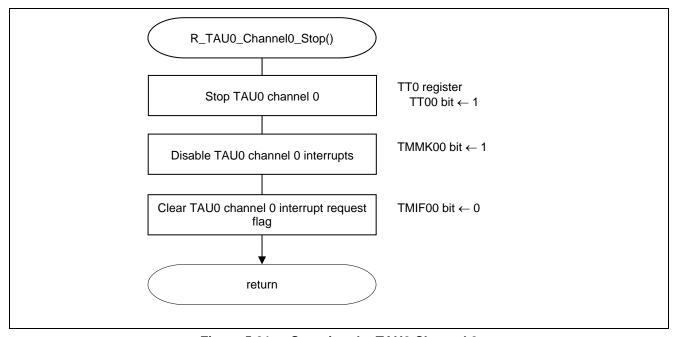
Figure 5.21 Stopping the TAU0 Channel 0
