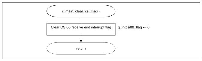
Figure 5.20 Clearing the CSI00 Transfer End Interrupt Flag
