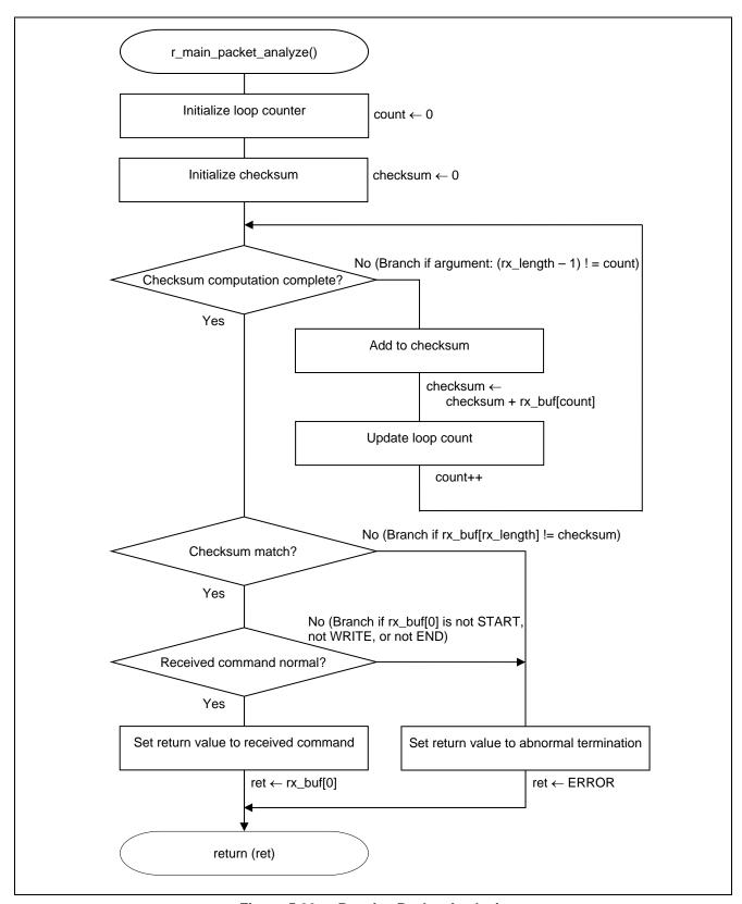
Figure 5.22 Receive Packet Analysis
