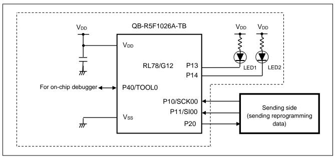
Figure 4.1 Hardware Configuration
