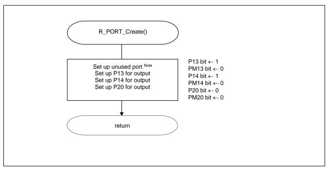
Figure 5.4 I/O Port Setup
