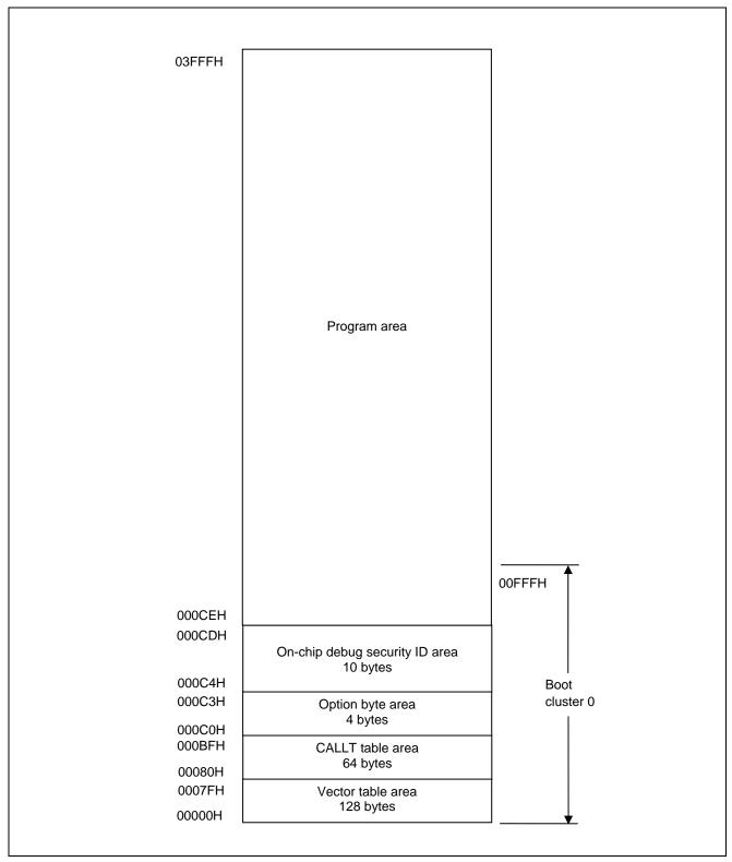
Figure 1.1 Code Flash Memory Configuration
