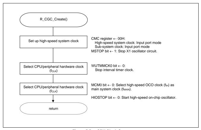
Figure 5.5 CPU Clock Setup
