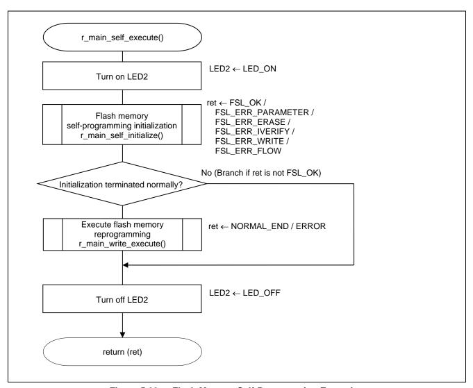
Figure 5.23 Flash Memory Self-Programming Execution
