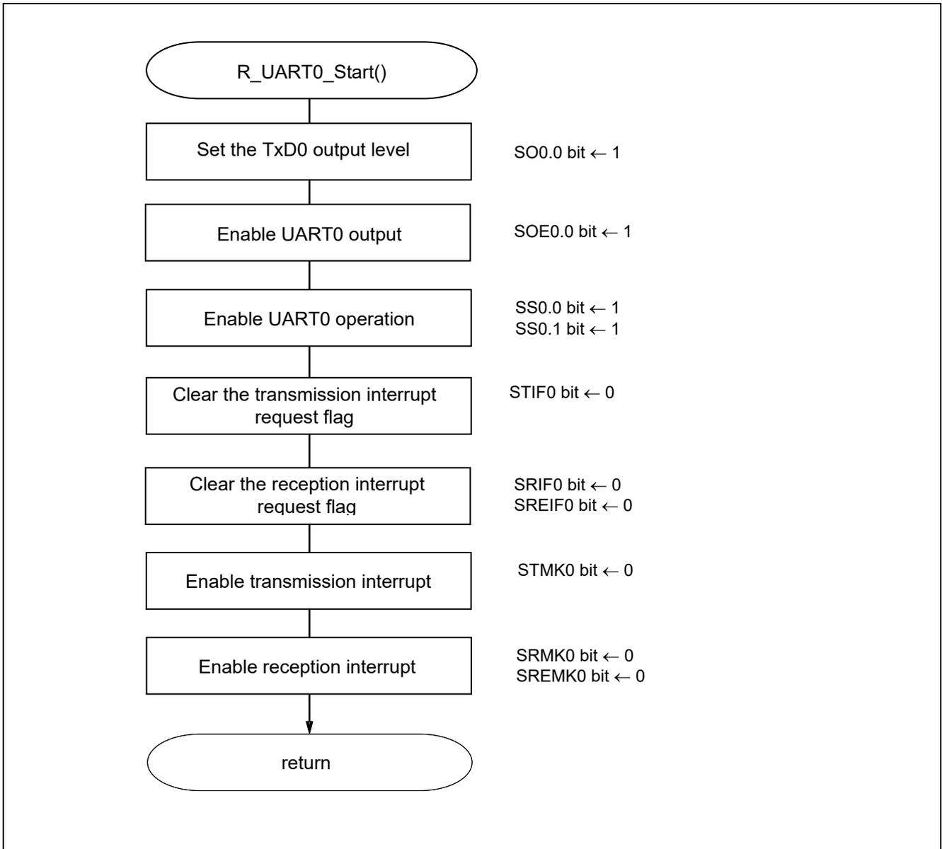
**Figure 5.15 UART0 Operation Start Function**
