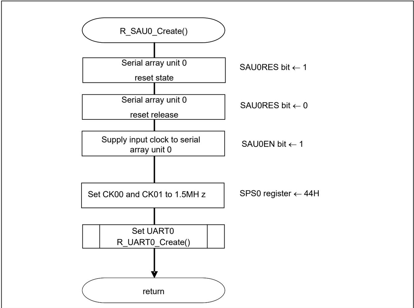
**Figure 5.9 Serial Array Unit Setup**
