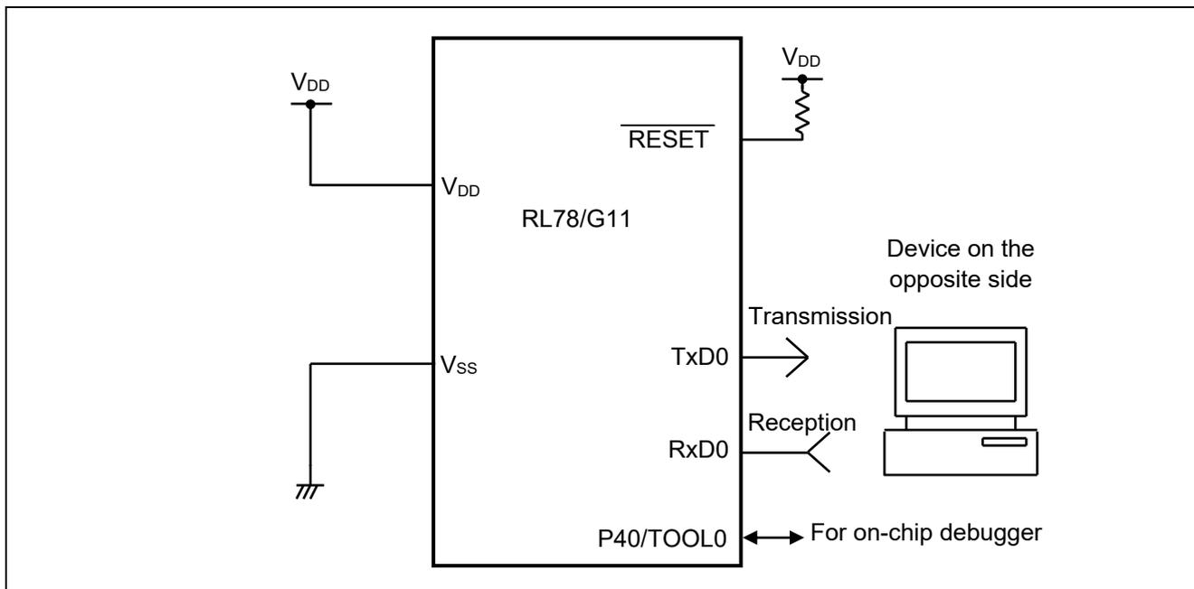
**Figure 4.1 Hardware Configuration**
