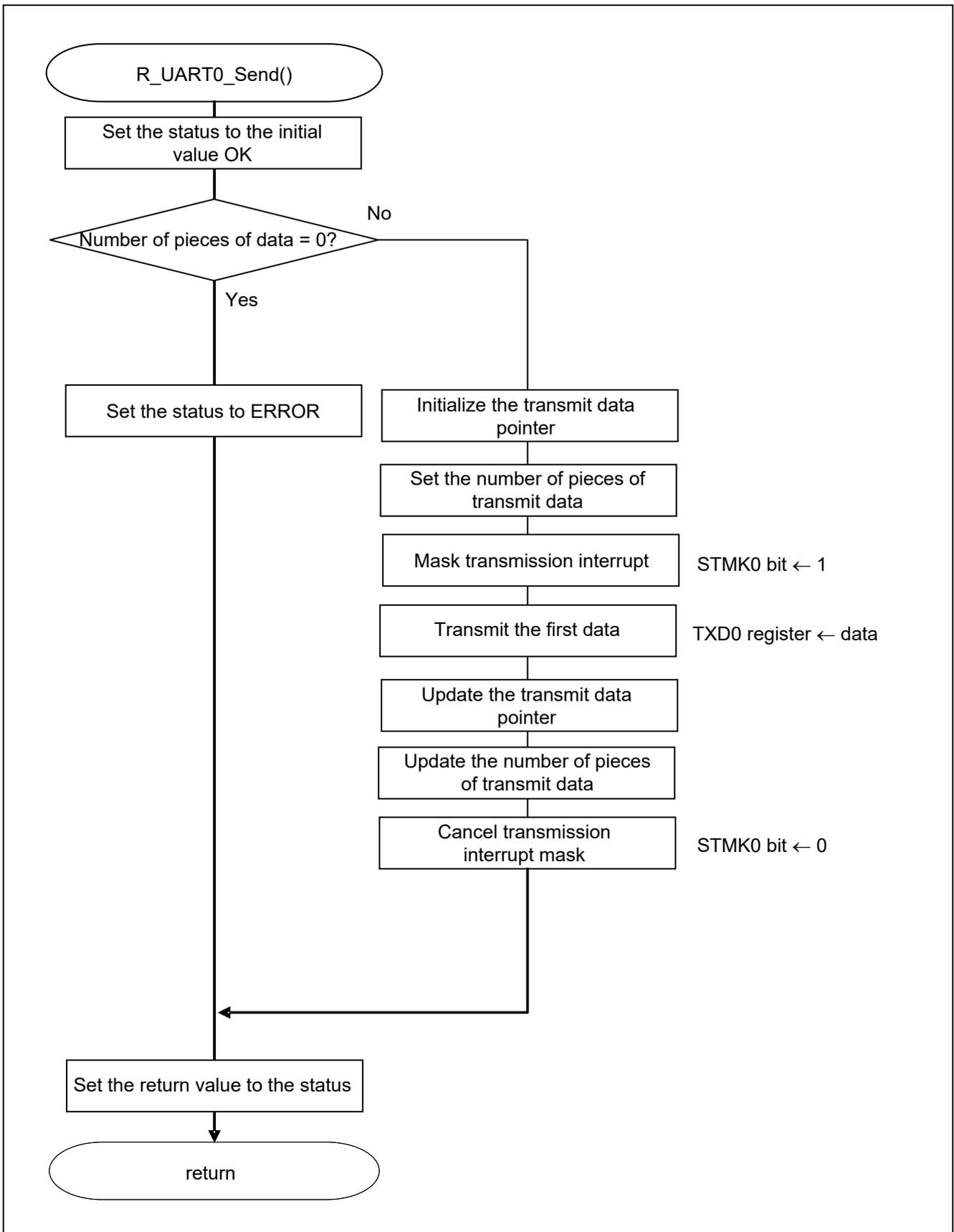
Figure 5.18 UART0 Data Transmission Function
