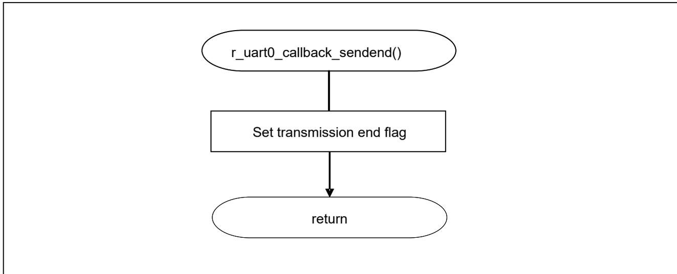
Figure 5.22 UART0 Transmission End Processing Function
