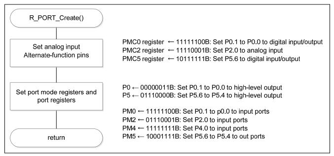
Figure 5.8 Input/Output Port Settings
