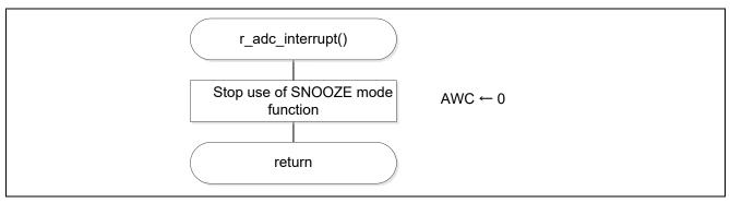
Figure 5.63 A/D Conversion Completion Interrupt Servicing
