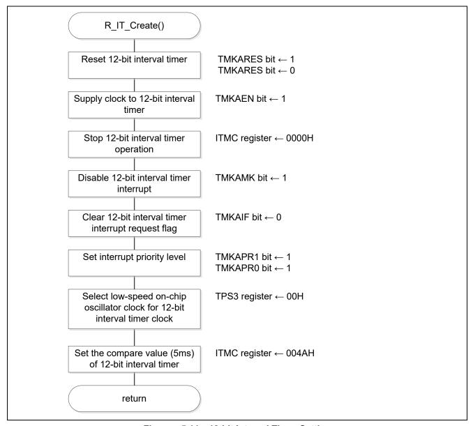
Figure 5.11 12-bit Interval Timer Setting
