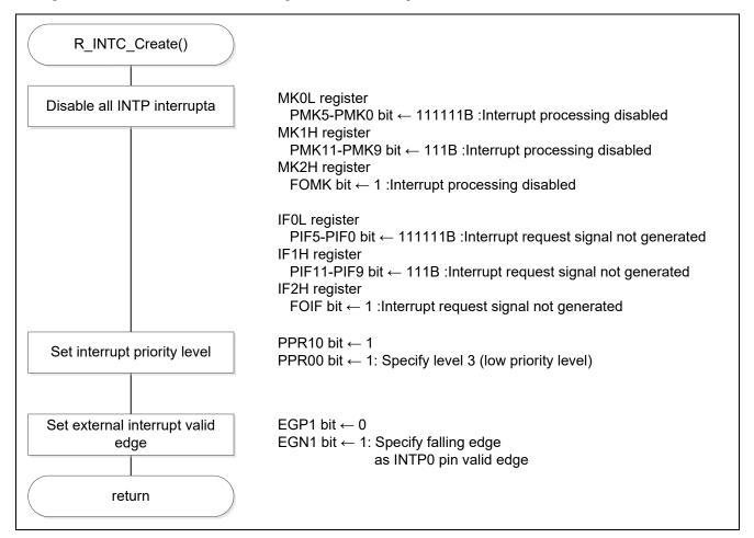
Figure 5.10 External Interrupt Setting
