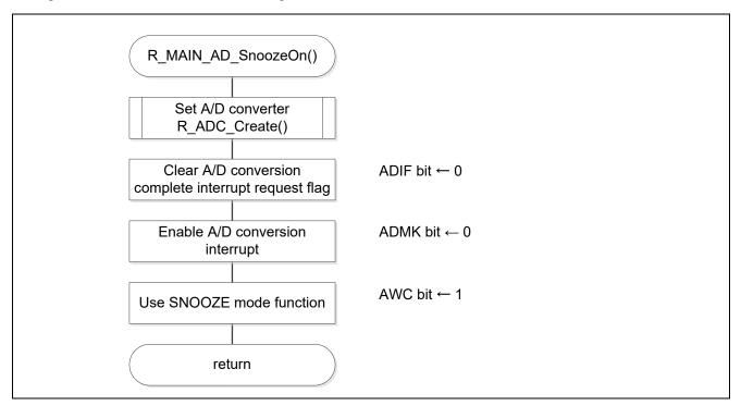
Figure 5.29 A/D Converter Setting
