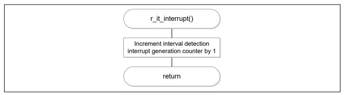
Figure 5.62 12-bit Interval Timer Interrupt Servicing
