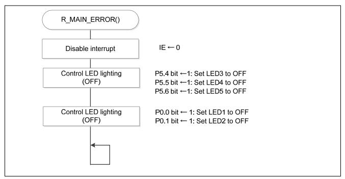
Figure 5.17 Error Processing of Status Transition
