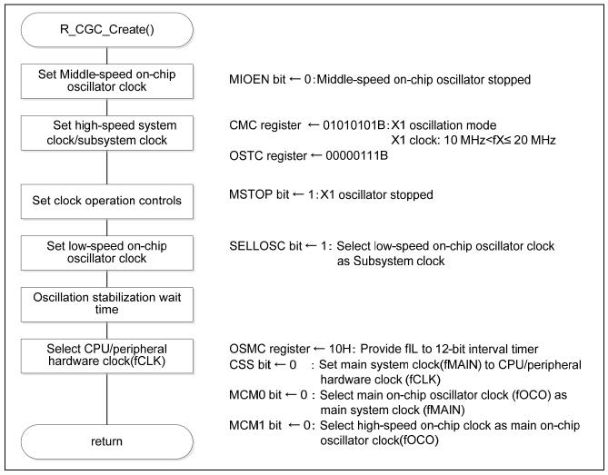
Figure 5.9 Clock Generator Setting
