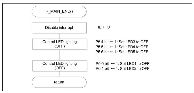
Figure 5.60 Status Transition End Processing
