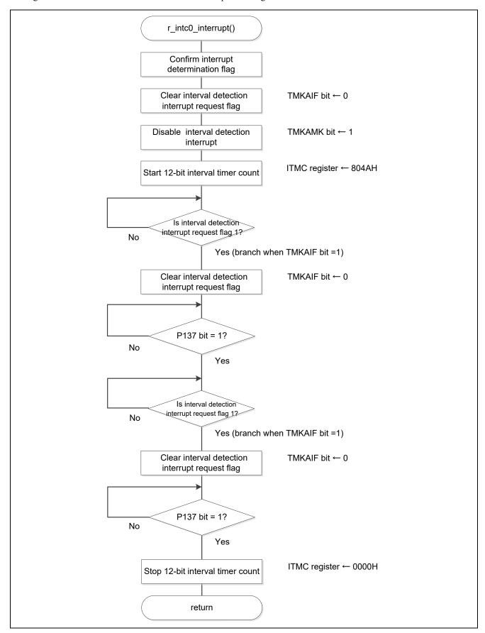
Figure 5.61 External Interrupt Servicing
