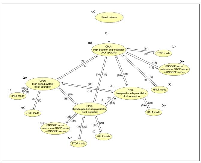
Figure 1.1 Operating Mode Status Transition Diagram
