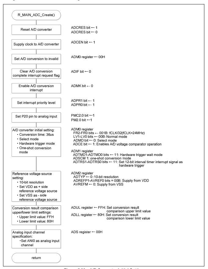
Figure 5.30 A/D Converter Initial Setting
