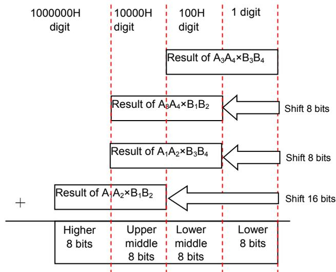
Figure 3.1 Data Scaling of 16 bits×16 bits
