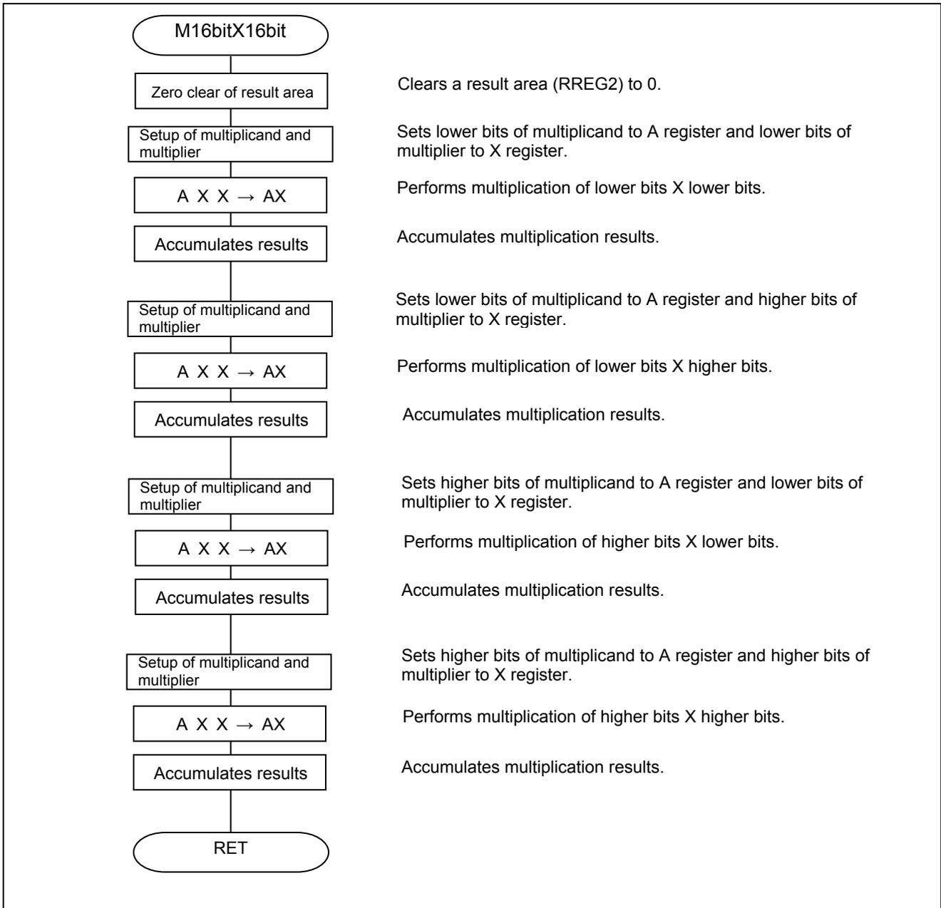
**Figure 3.9 Multiplication Processing of 16 Bits Data**
