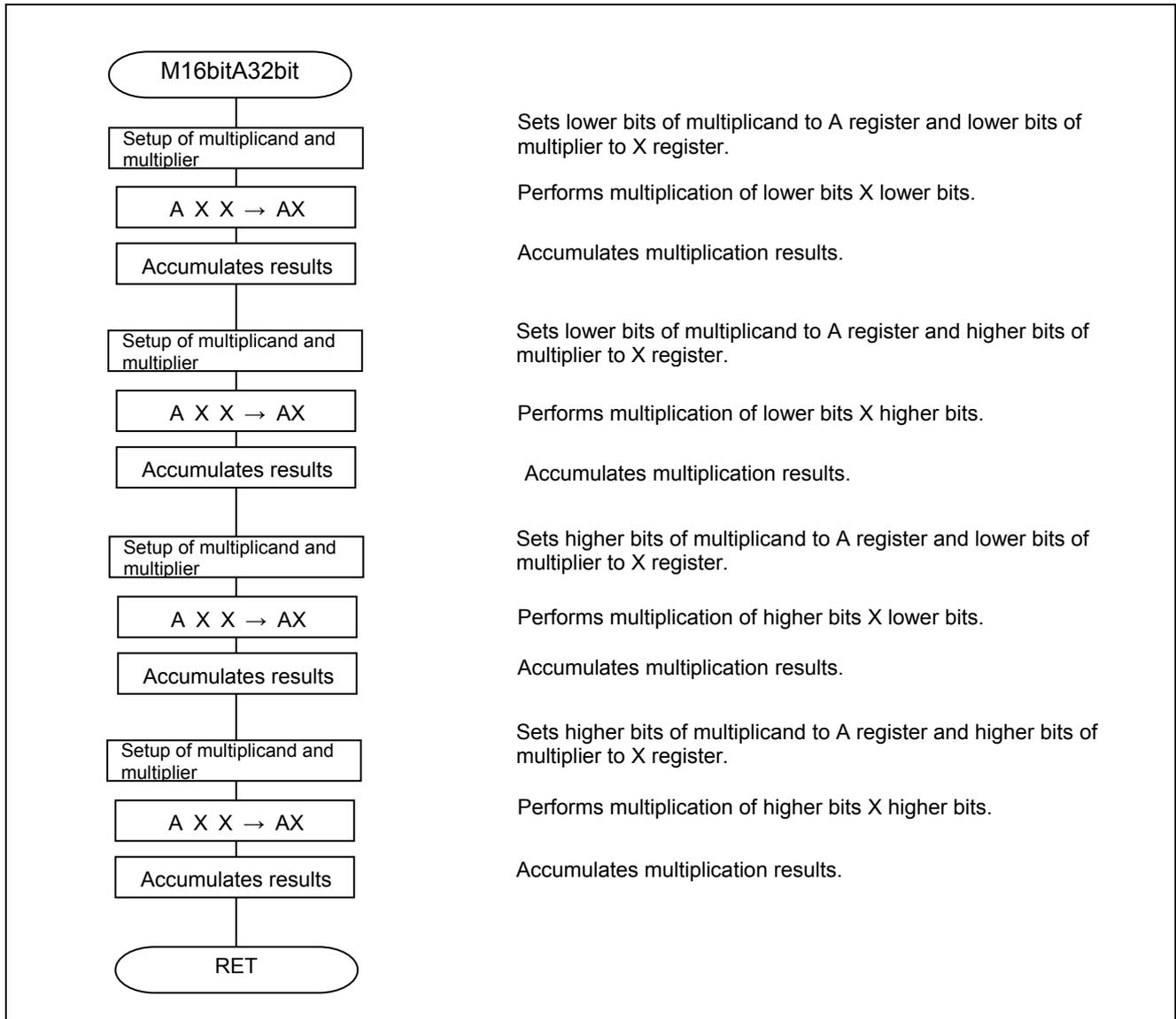
Figure 3.10 Multiply and Accumulation Processing
