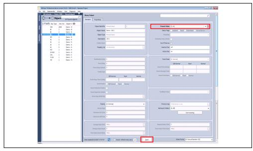
*Step 7.* Press Send button with checked Present Value 1 [ON]. In Suitcase #1, RED LED #1 is turned ON. Try again Present Value 0 [OFF] to turn off the RED LED #1 in Suitcase #1.
