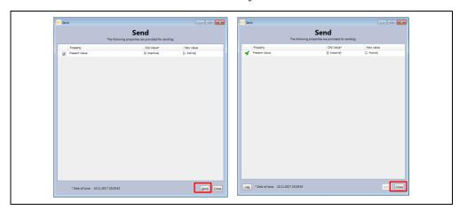
Step 9. Show updated value in object Windows. When object BO 0 "Fan" is active, light up the Green LED in the Suitcase #2. (Try object BO 0"Fan" for value [0] Inactive to turn off the Green LED)
