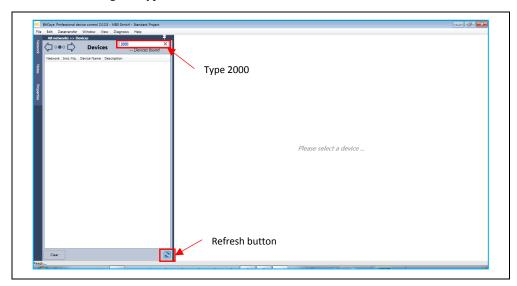
Step 4. Select device "2000" in device list will show the list of device objects in the Device filed
