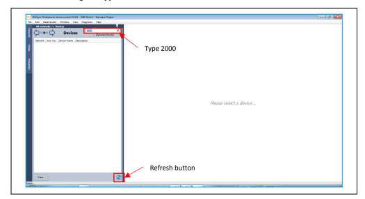
Step 4. Click back arrow (Network button) to check number of Notes in the connected network. The All Networks Windows shows the numbers of devices in the network
