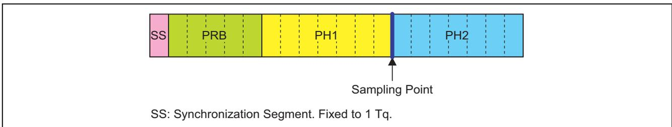
Figure 4.5.1 Bit Timing
