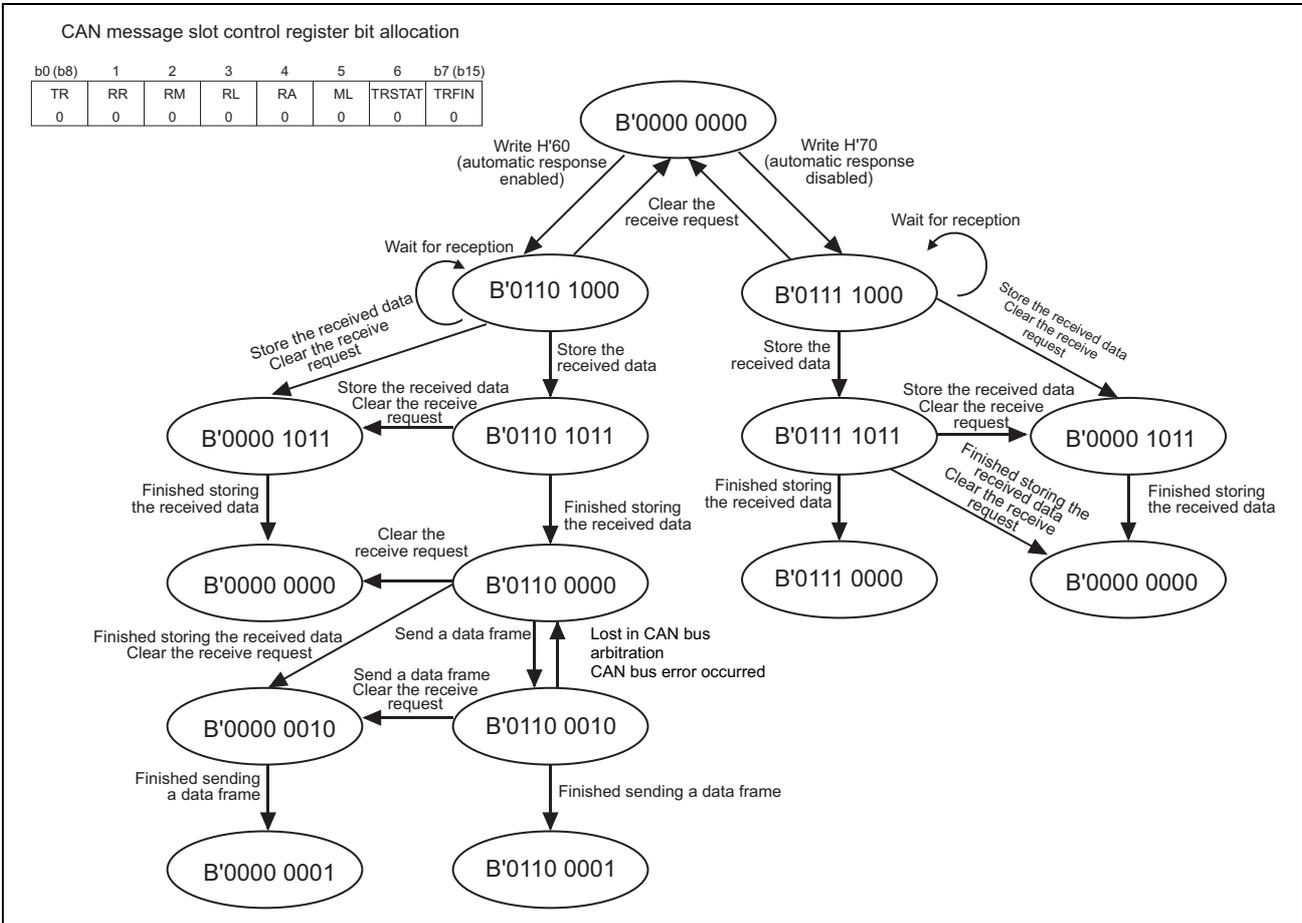
Figure 4.4.1 The State of CAN Message Slot Control Registers during Remote Frame Reception
