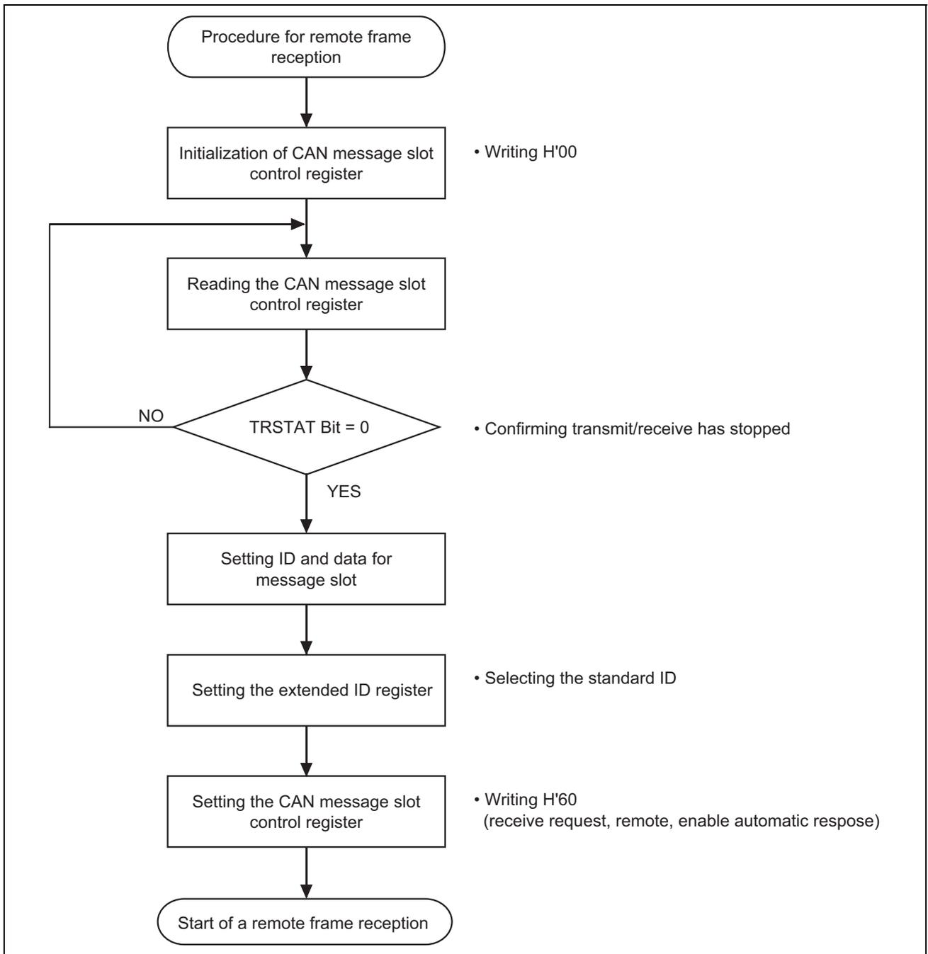
Figure 4.3.1 Remote Frame Reception Processing
