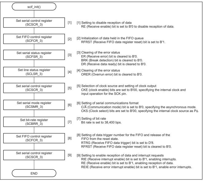
Figure 6 Flow for Initialization of Data Reception in Asynchronous Mode
