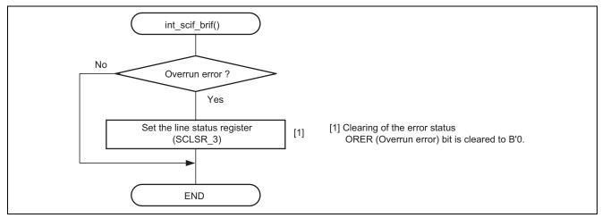
Figure 9 Flow for Handling of Receive Error Interrupts in Asynchronous Mode
