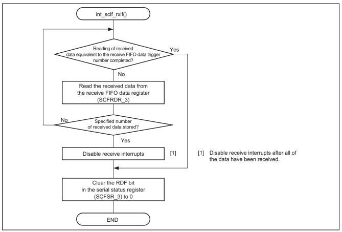
Figure 8 Flow for Handling of Receive Interrupts in Asynchronous Mode
