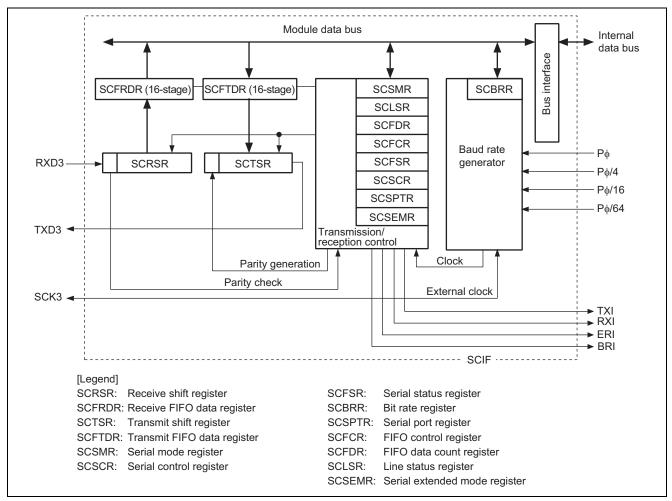
Figure 2 Block Diagram of the SCIF
