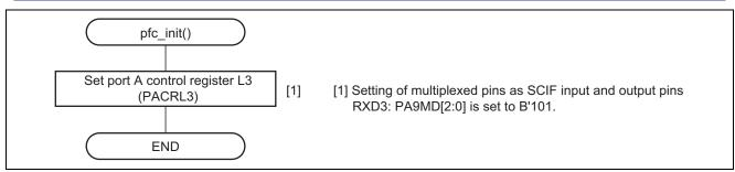
Figure 7 Flow for Setting up the Pin Function Controller
