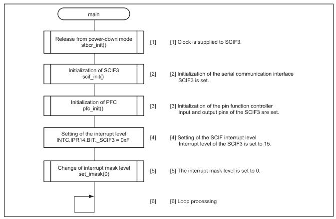
Figure 4 Flow of Processing by the Sample Program
