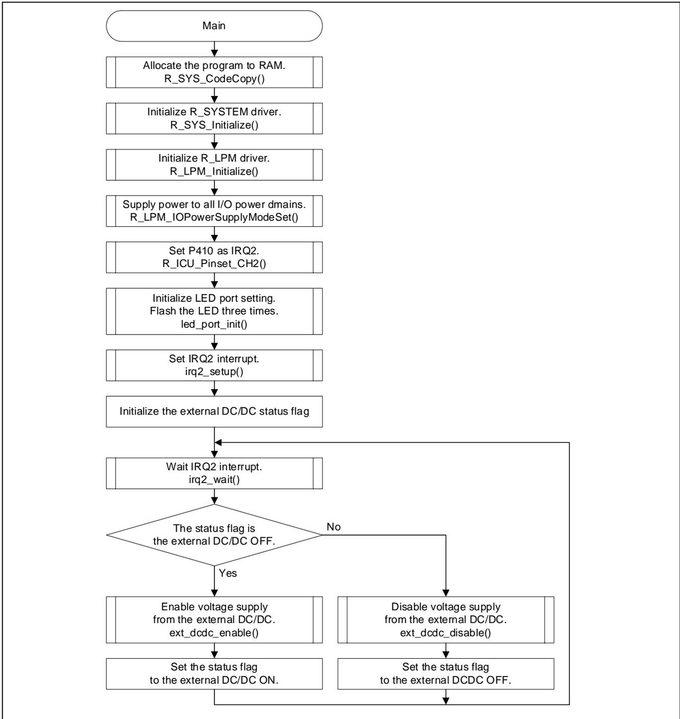
Figure 7-2 Main process of changing the voltage supply to the internal circuit
