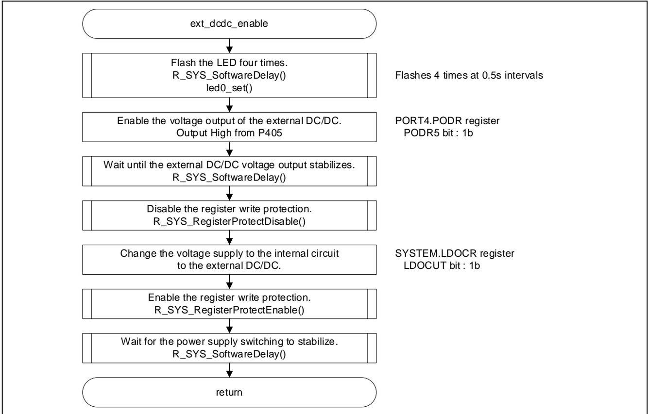
Figure 7-3 Validation of voltage supply from the external DC/DC
