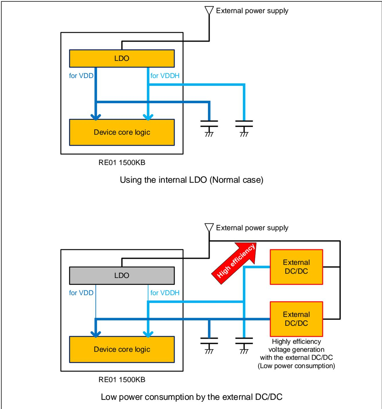
Figure 1-1 Image of low power consumption by the external DC/DC
