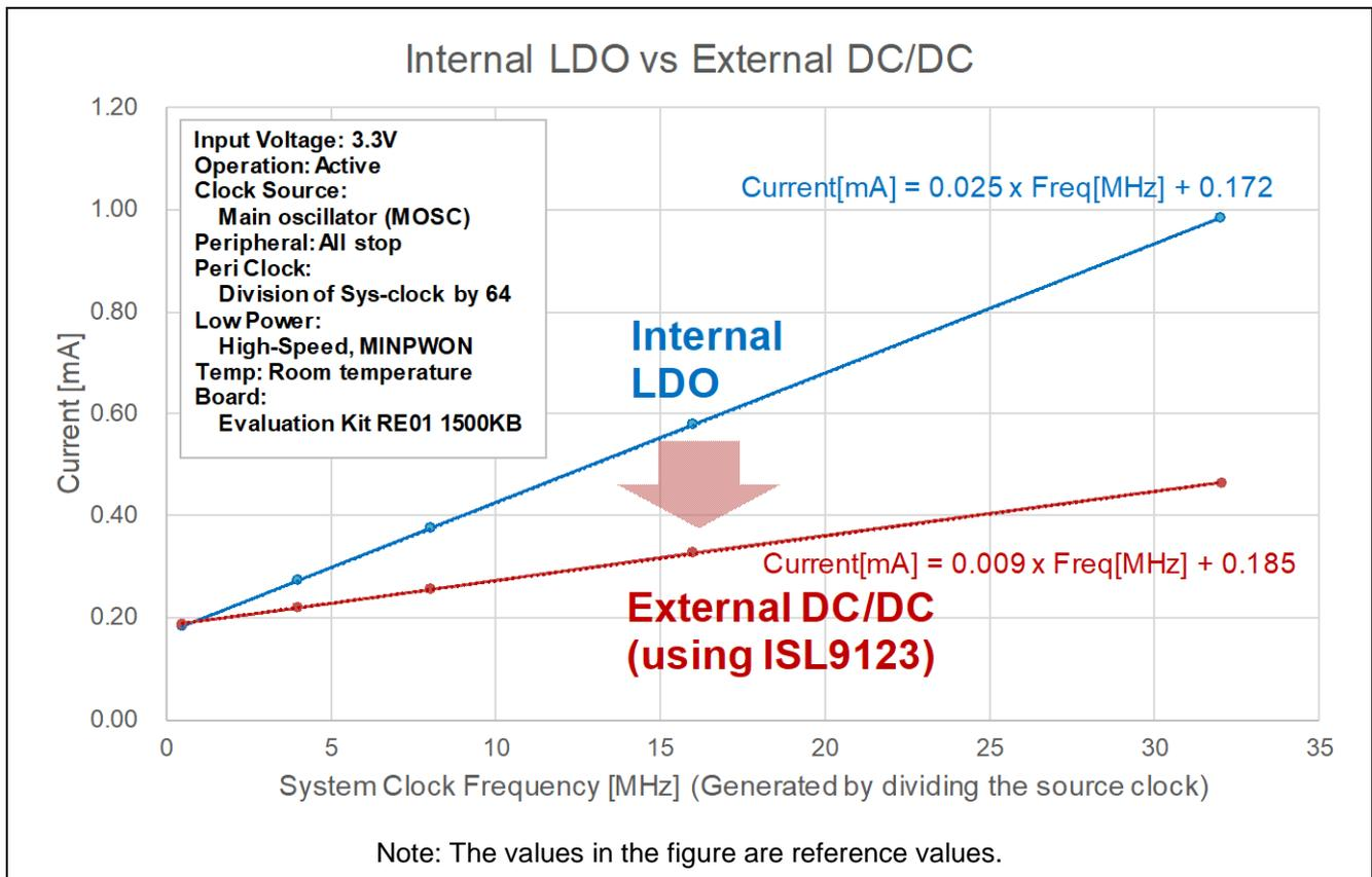
Figure 3-1 Difference in current consumption between the internal LDO and the external DC/DC
