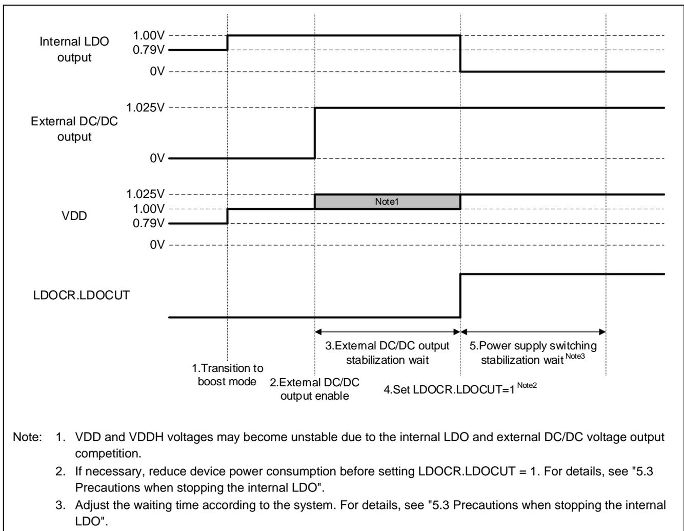
Figure 5-2 Timing chart for enabling the external DC/DC (when transitioning to boost mode)
