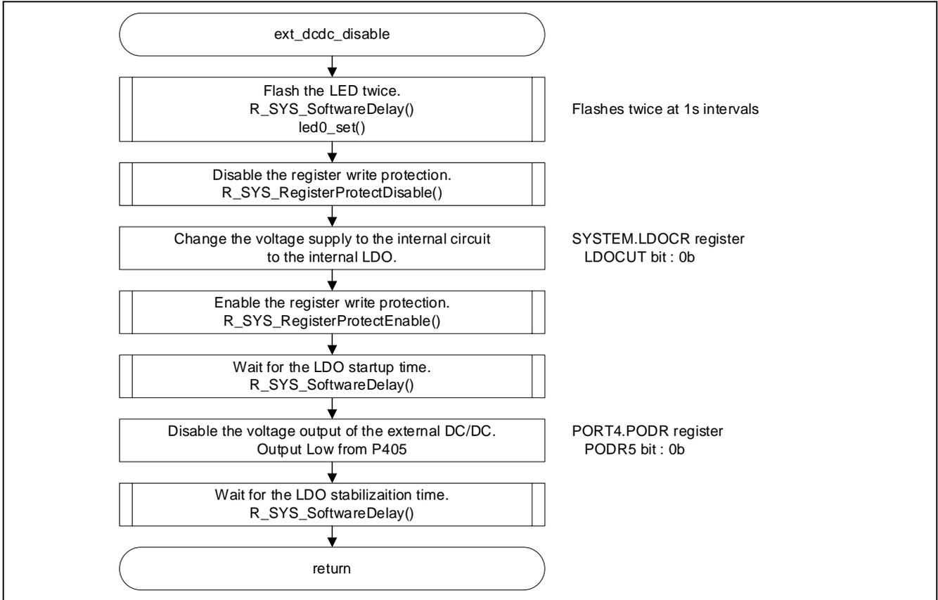
Figure 7-4 Disabling voltage supply from the external DC/DC
