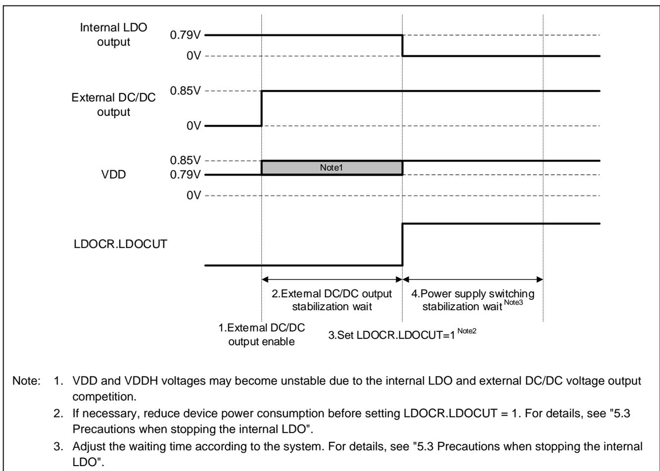
Figure 5-1 Timing chart for enabling the external DC/DC (when not transitioning to boost mode)
