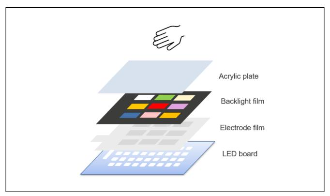
Figure 1.2 Touchless Button Electrode Board Configuration
