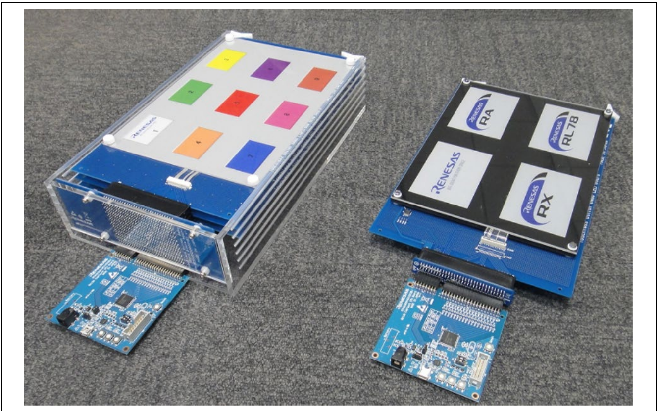
Figure 1.1 Touchless Button Electrode Board (Left: with housing, Right: without housing)
