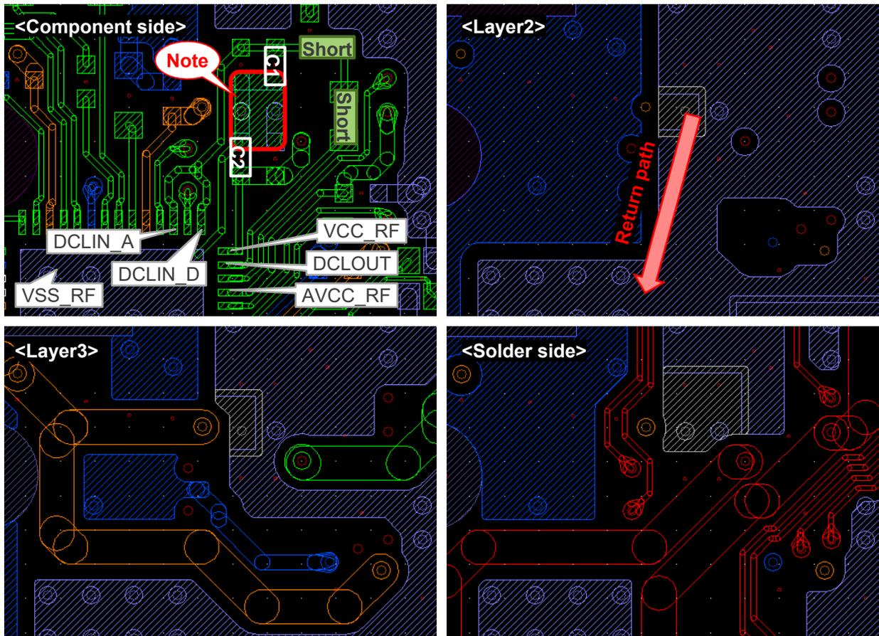
Note: Ground pattern in the loop which is enclosed with line connecting “DCLOUT” and “DCLIN\_A”.
