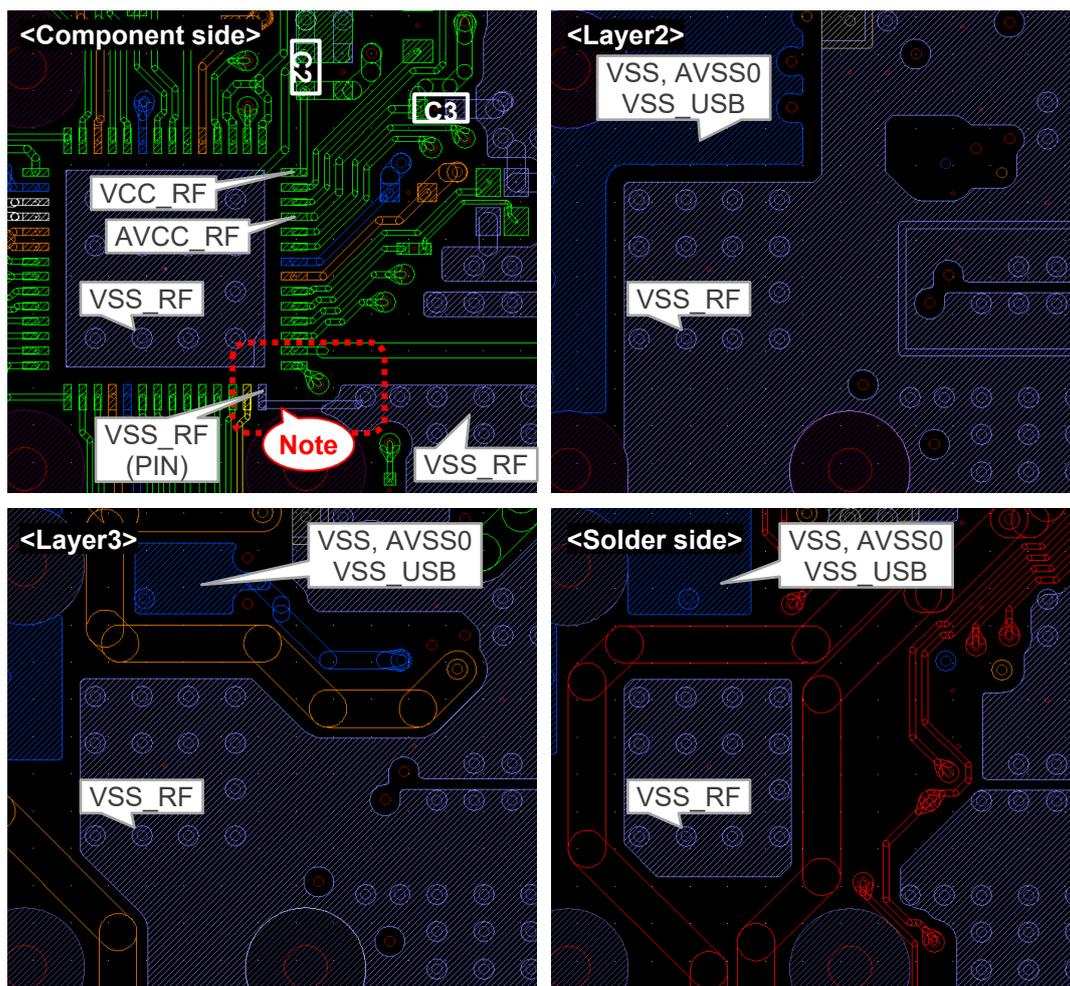
Note: Separate the ground area for "VSS\_RF (Exposed Die Pad)" and "VSS\_RF (PIN)" on the component side of the board.
