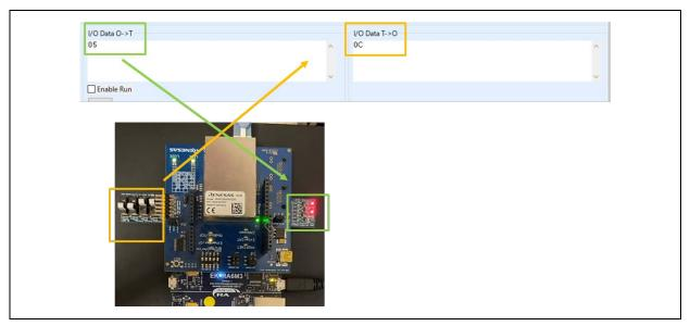
Figure 3-41 Remote-IO (LED/Switch) control [EtherNet/IP]
