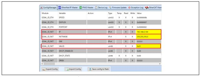
Figure 3-20 Set IP address on R-IN32M3 module
