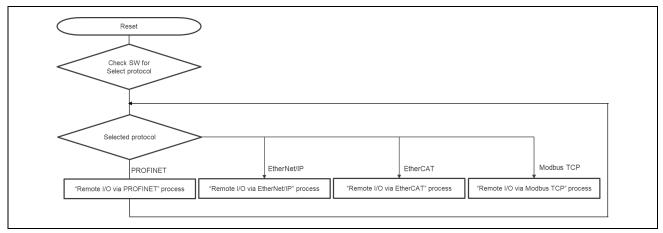
Figure 3-51 Multi-protocol selector flow
