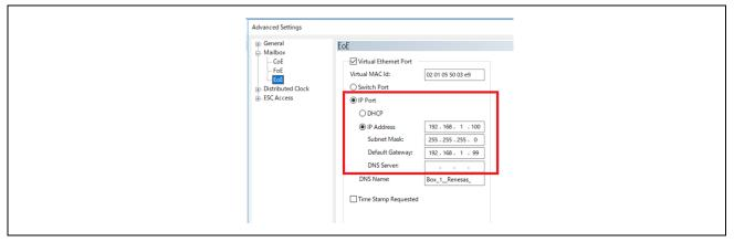
Figure 3.58 TwinCAT Network setting
