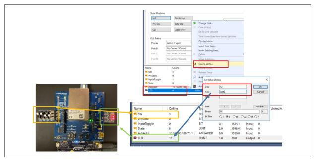
Figure 3-48 Remote I/O control [EtherCAT]
