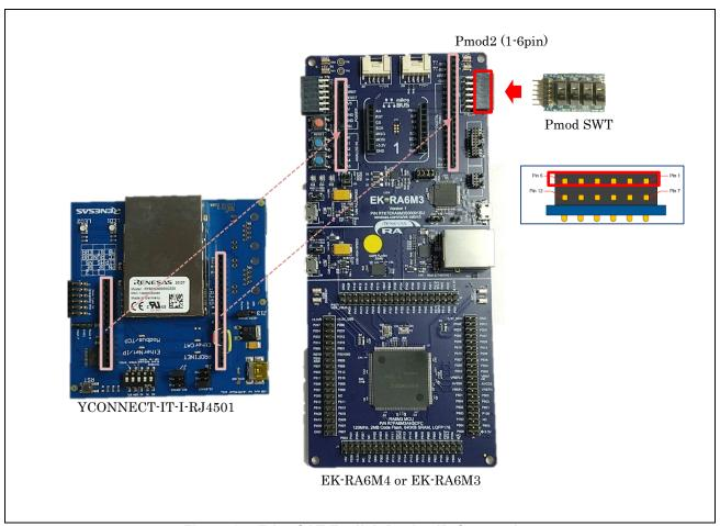
Figure 2-5 EtherCAT Explicit Device ID Connection
