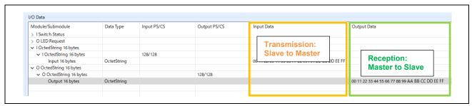
Figure 3-27 Mirror control [PROFINET]
