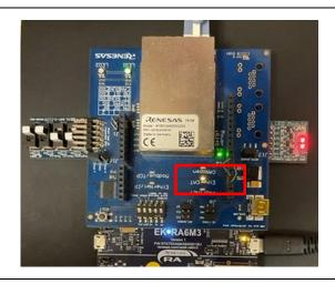
Figure 3-43 Protocol LED: EtherCAT
