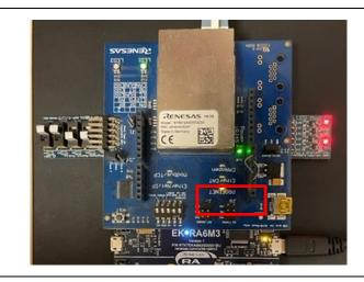
Figure 3-14 Protocol LED: PROFINET
