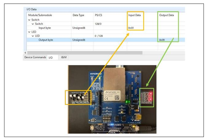
Figure 3-26 Remote I/O control [PROFINET]
