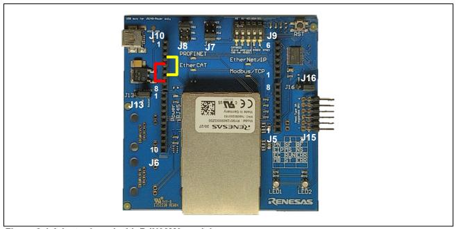
Figure 2-1 Adaptor board with R-IN32M3 module
