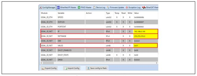
Figure 3-34 Set IP address on R-IN32M3 module
