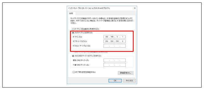
Figure 3-15 Set Static IP address
