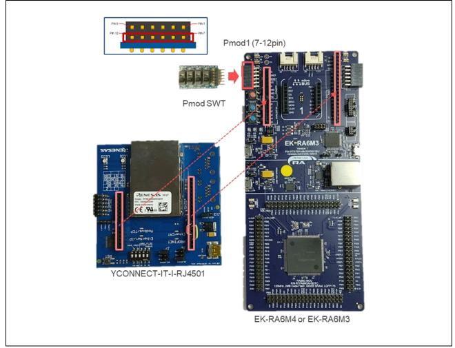
Figure 2-3 Multi-protocol Selector Connection
