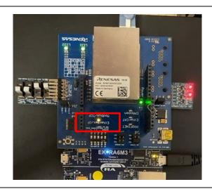
Figure 3-28 Protocol LED: EtherNet/IP
