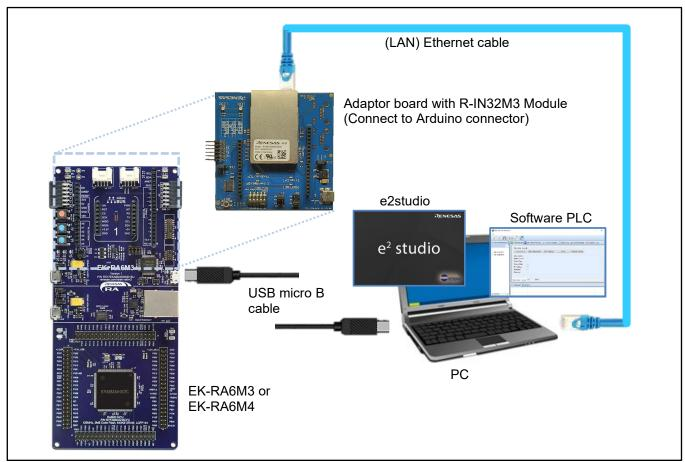
Figure 3-1 Connection configuration
