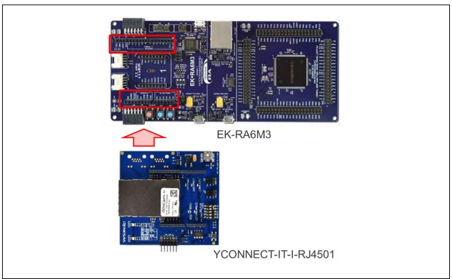
Figure 2-2 Arduino<sup>™</sup> Connection
