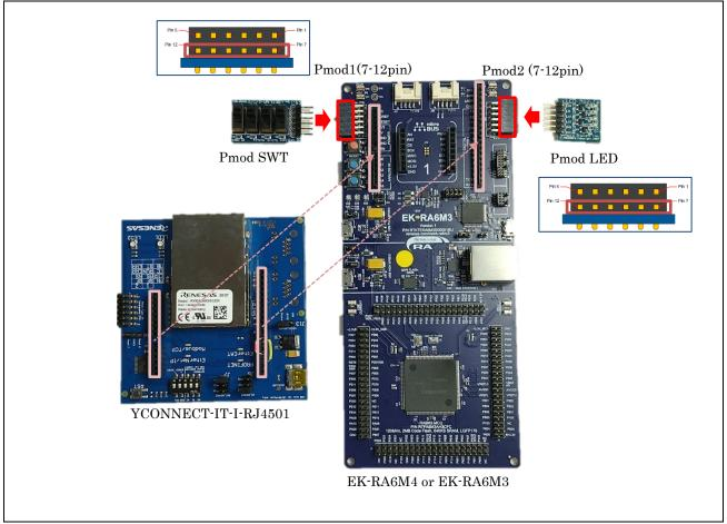
Figure 2-4 Remote I/O Connection
