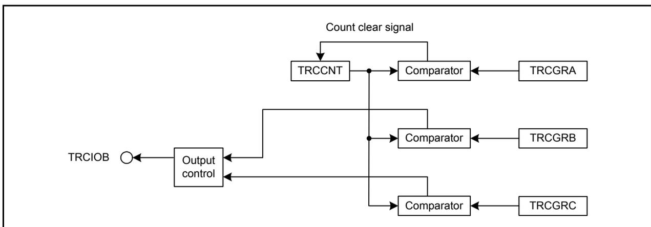
Figure 3.1 Block Diagram
