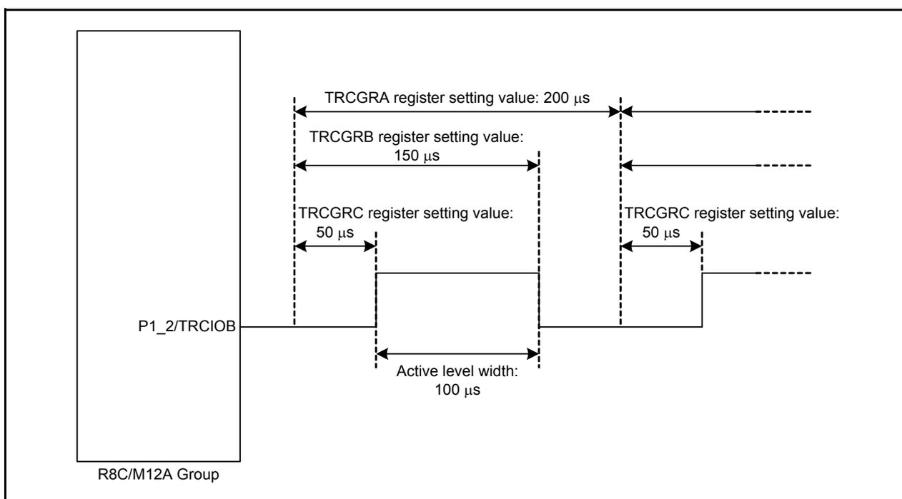
Figure 3.2 Timing Diagram
