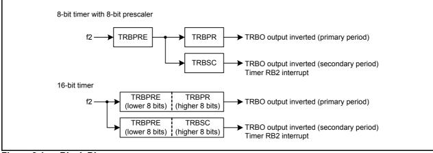
Figure 3.1 Block Diagram
