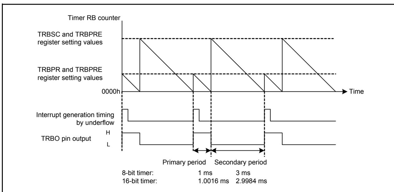
Figure 3.2 Timing Diagram
