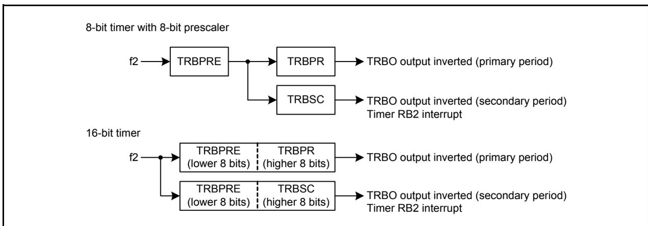
Figure 3.1 Block Diagram
