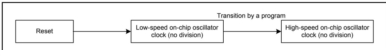
**Figure 1.1 Transition Diagram of the System Base Clock (Sample Program 1)**
