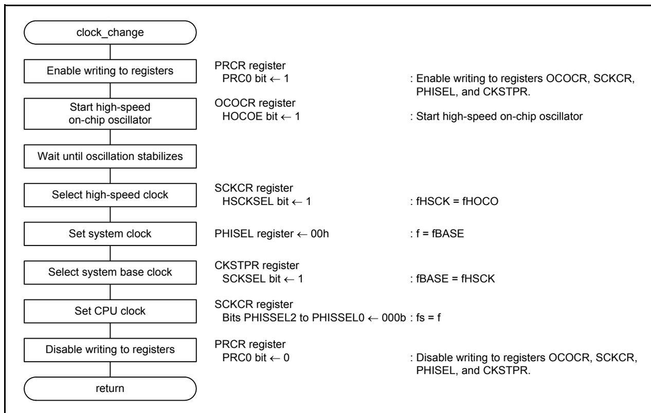
Figure 6.4 System Base Clock Switching
