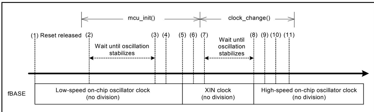
Figure 6.1 Timing Diagram of the Sample Program 4 Setting
