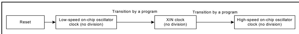
**Figure 1.4 Transition Diagram of the System Base Clock (Sample Program 4)**
