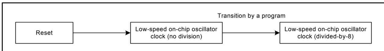
**Figure 1.2 Transition Diagram of the System Base Clock (Sample Program 2)**
