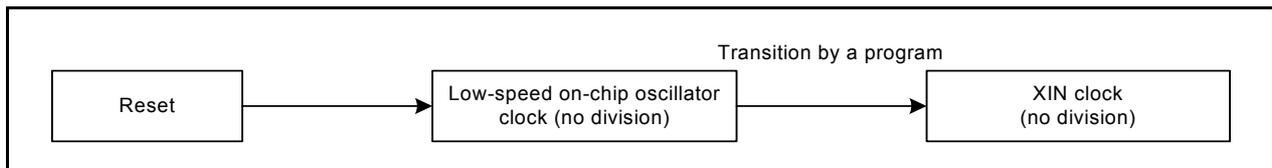
**Figure 1.3 Transition Diagram of the System Base Clock (Sample Program 3)**
