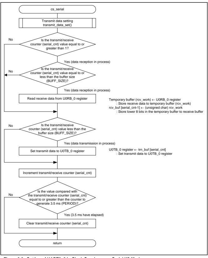
Figure 3.6 Setting of UART0\_0 in Clock Synchronous Serial I/O Mode
