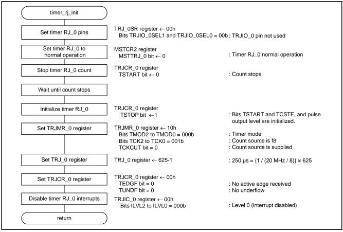
Figure 3.4 Initial Setting of Timer RJ\_0
