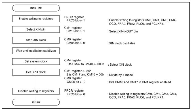
Figure 3.3 System Clock Setting
