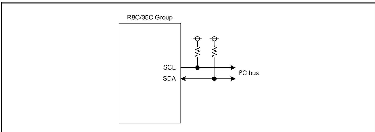
Figure 3.2 Block Diagram
