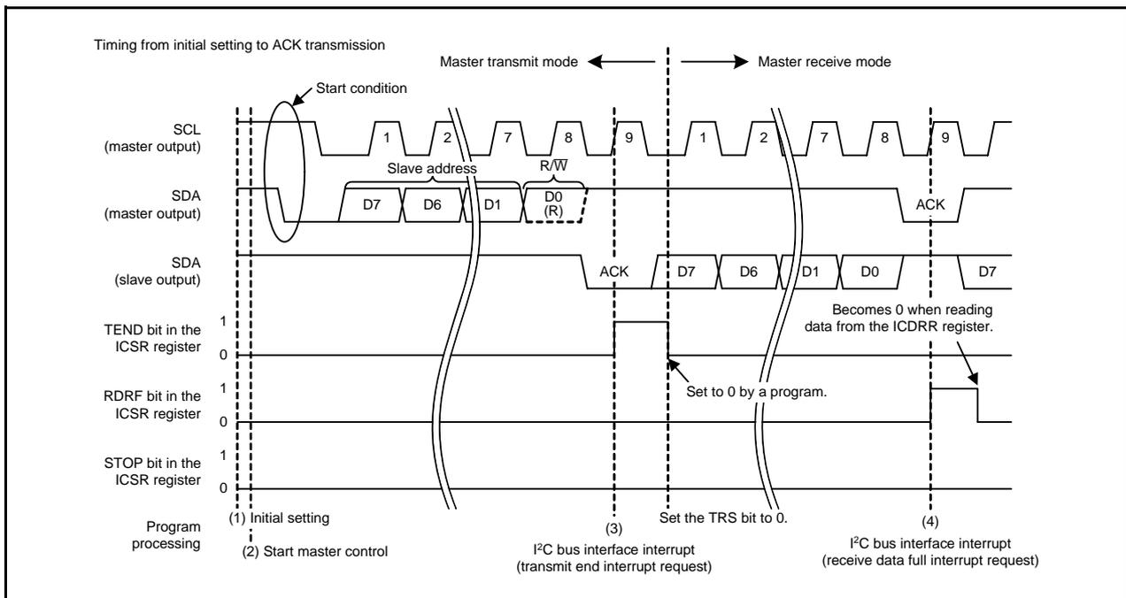
Figure 3.5 Master Receive Timing (1)
