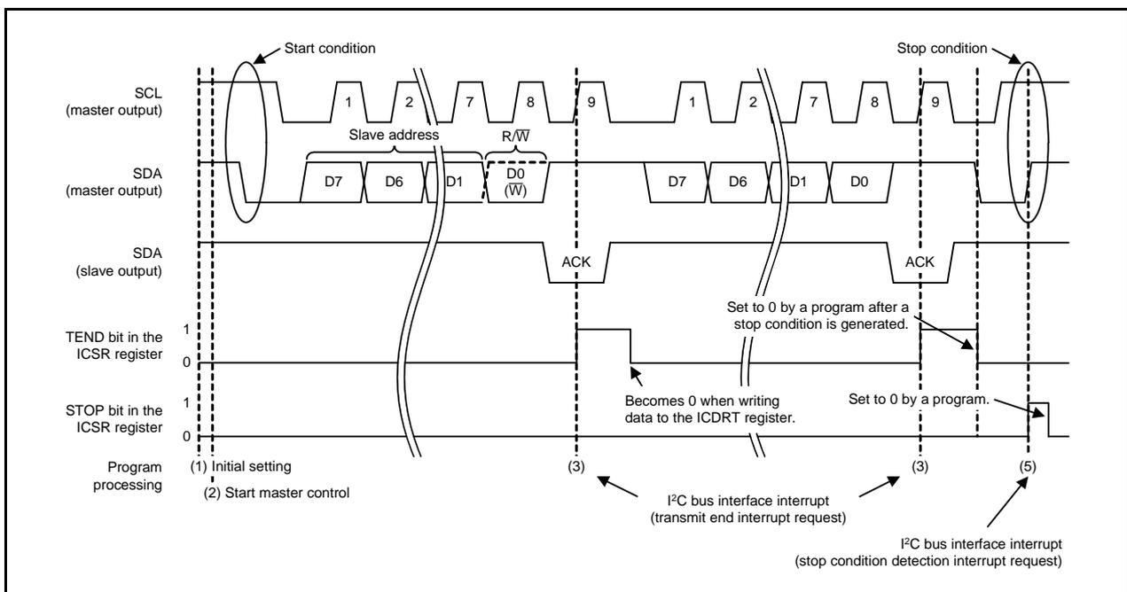
Figure 3.4 Master Transmit Timing
