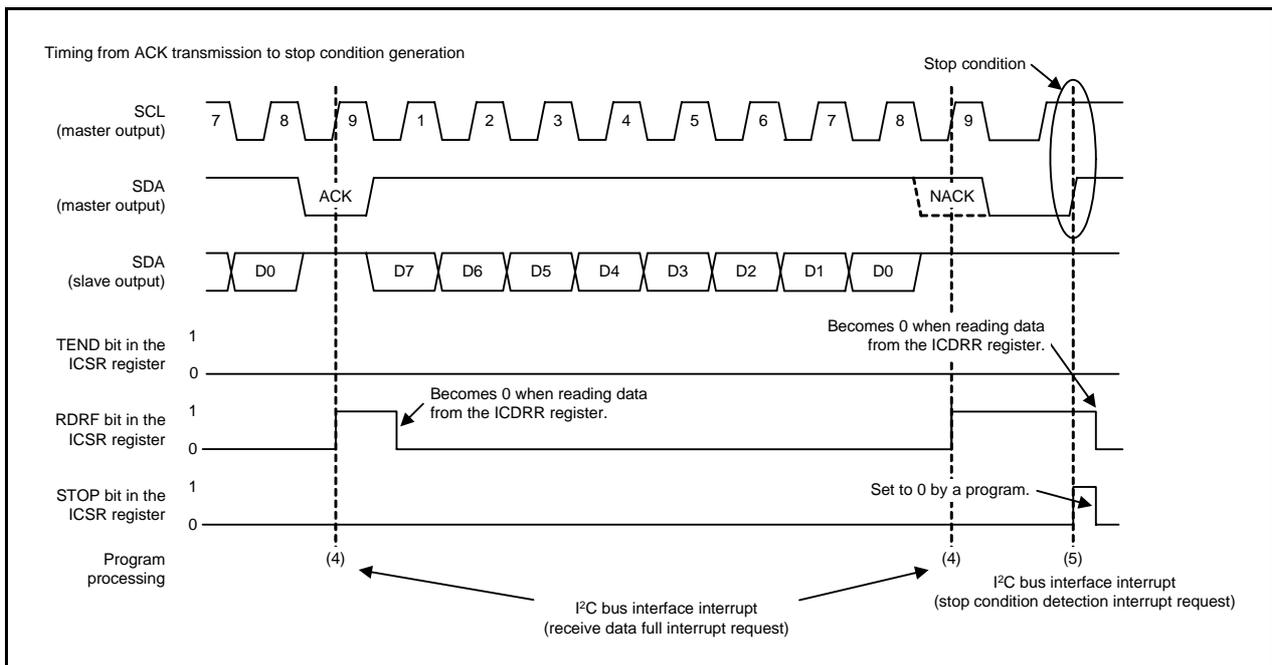
Figure 3.6 Master Receive Timing (2)
