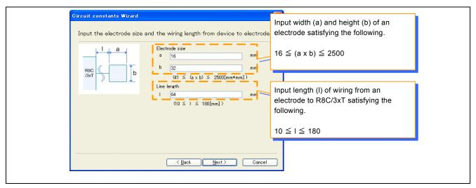
Figure 7-6 Width and Height of the electrode, wiring length settings
