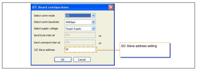
Figure 4-11 I2C Slave address setting
