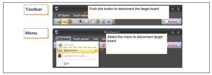
Figure 4-13 The method of disconnection with target board
