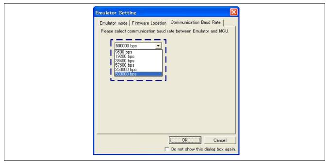
Figure 3-7 Emulator communication baud rate setting
