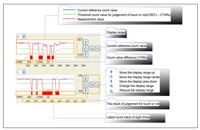
Figure 7-31 Detail explanation of graph display
