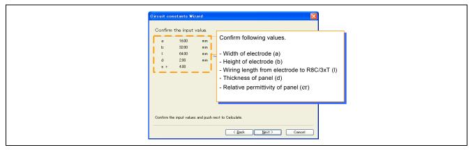
Figure 7-9 Confirmation of the input value (Electrode type is rectangle)
