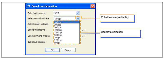
Figure 4-7 Communication baudrate(for SPI3/SPI4) selection
