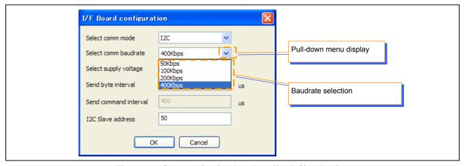
Figure 4-8 Communication baudrate(for I2C) selection
