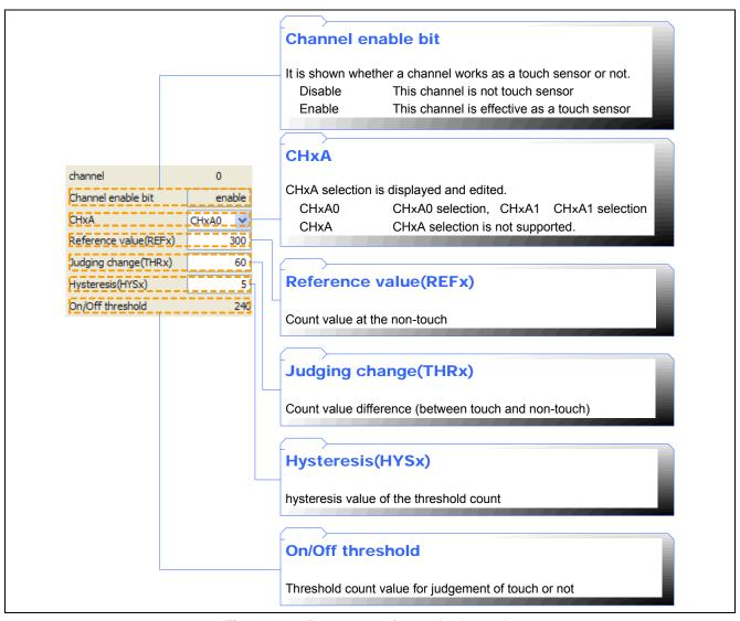
Figure 7-28 Parameters for each channels
