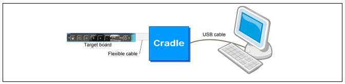
Figure 2-2 Connection between a target board and a PC using the Cradle board
