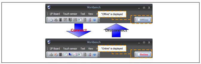
Figure 4-12 The status of connection with target board
