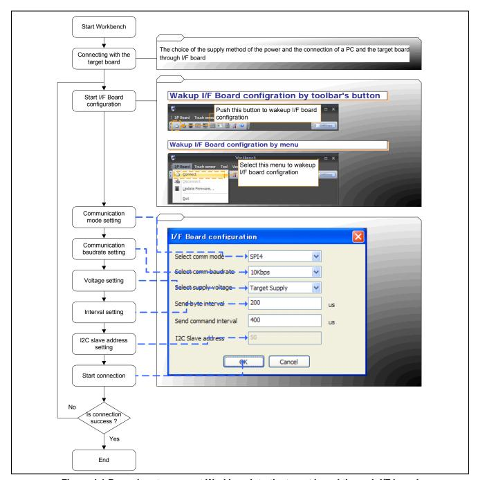
Figure 4-1 Procedure to connect Workbench to the target board through I/F board
