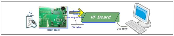
Figure 4-2 The example using the power supply circuit on the target board
