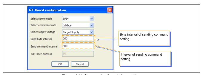
Figure 4-10 Communication timing setting
