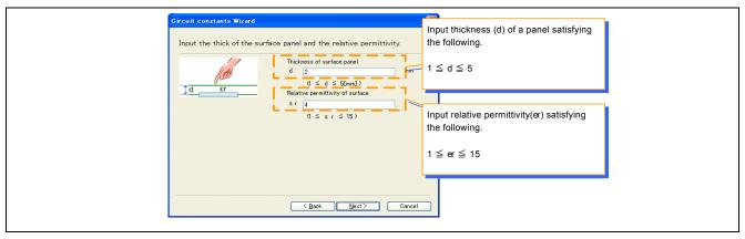
Figure 7-8 Thickness and Relative permittivity of the panel settings
