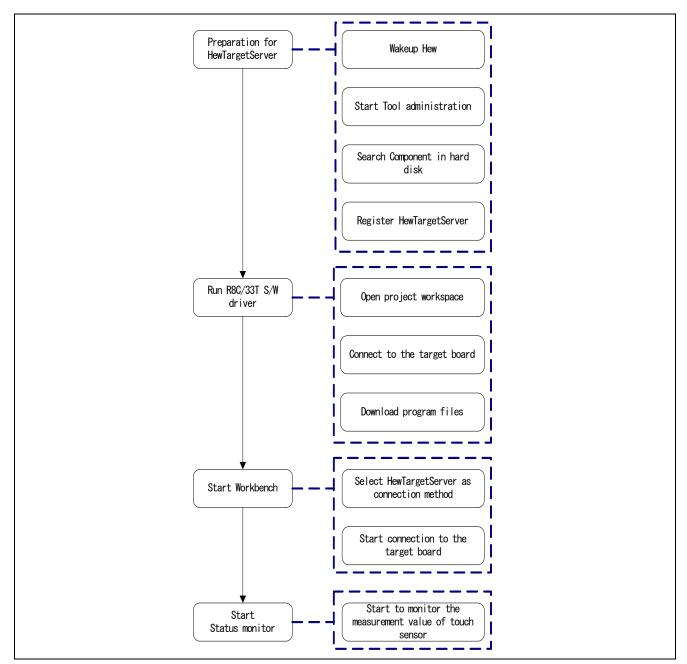
Figure 3-1 Procedure for connecting Workbench with target board through HEW
