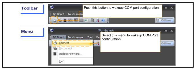
Figure 2-3 the method of starting COM Port configuration
