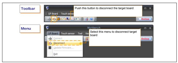
Figure 2-11 The method of disconnection with target board
