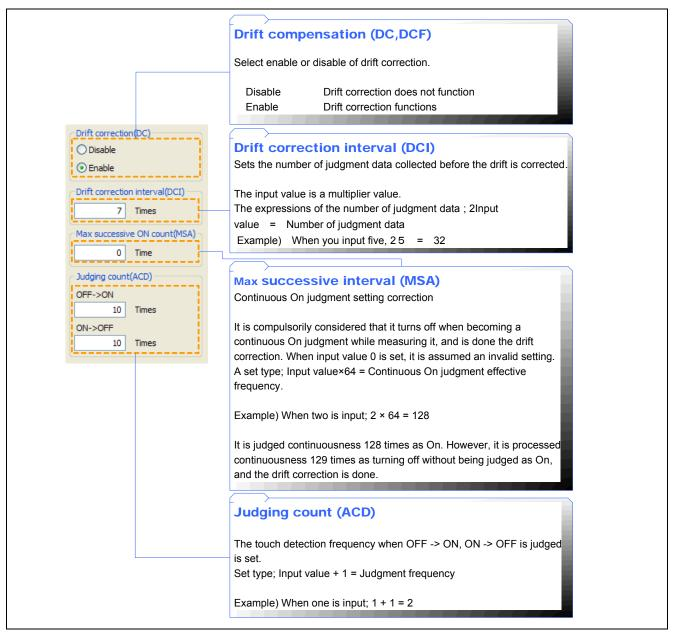
Figure 7-24 Common parameters
