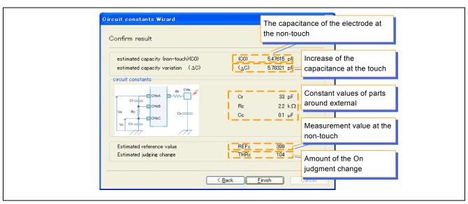
Figure 7-11 Result of calculation
