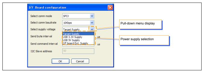
Figure 4-9 The method of supply power selection
