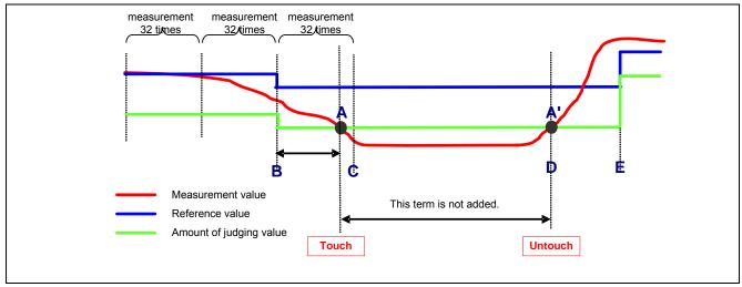
Figure 7-26 The timing of drift correction
