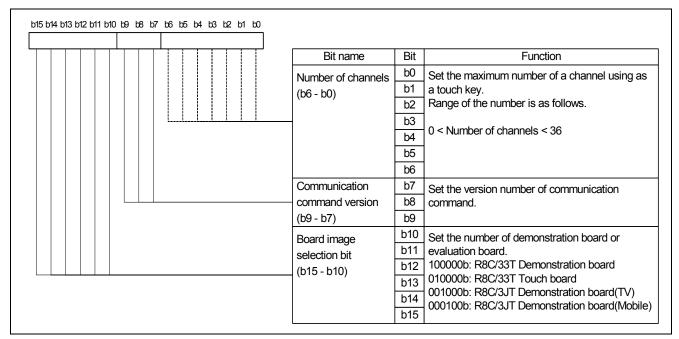
Figure 5-1 Bit pattern of ChipID
