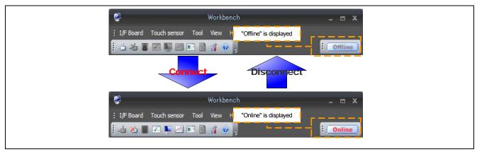
Figure 2-10 The status of connection with target board
