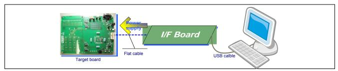
Figure 4-3 The example of power supply from the USB port
