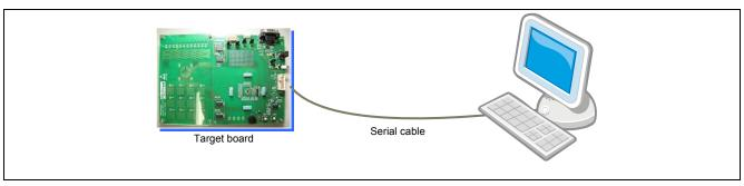
Figure 2-1 Connection between a target board and a PC using a serial cable
