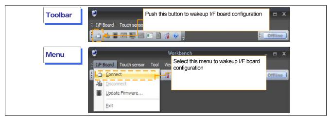
Figure 4-5 The method of starting I/F Board configuration
