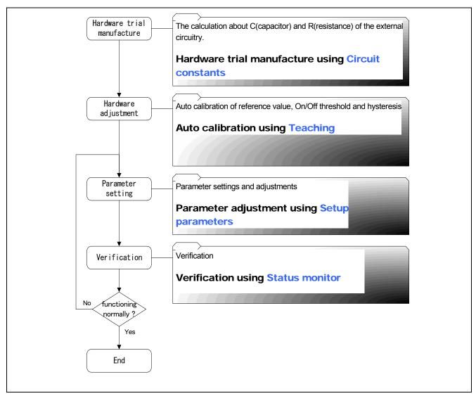
Figure 7-1 Adjustment flow chart
