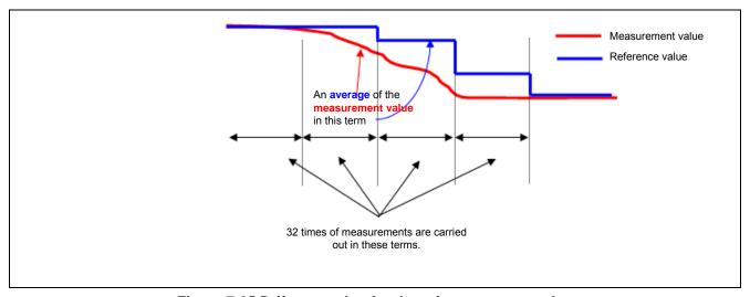
Figure 7-25 Drift correction for the reference count value
