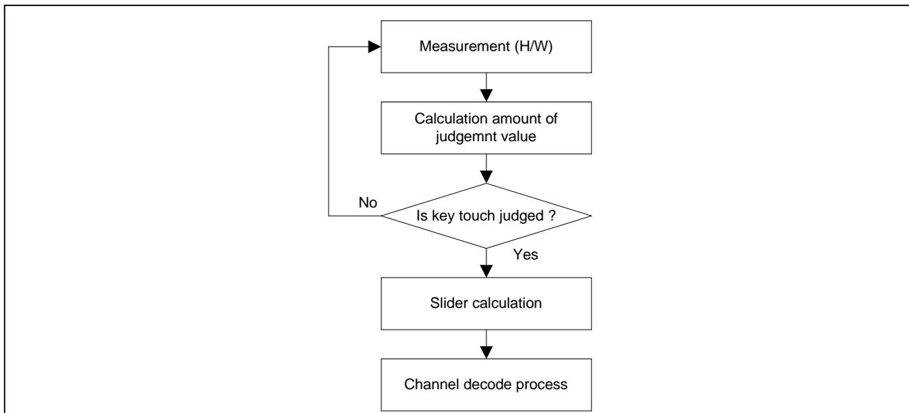
Figure 2-1 The flowchart of slider process
