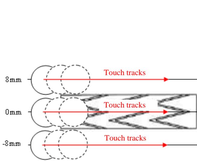
Figure 1-9 Touch tracks and starting position
