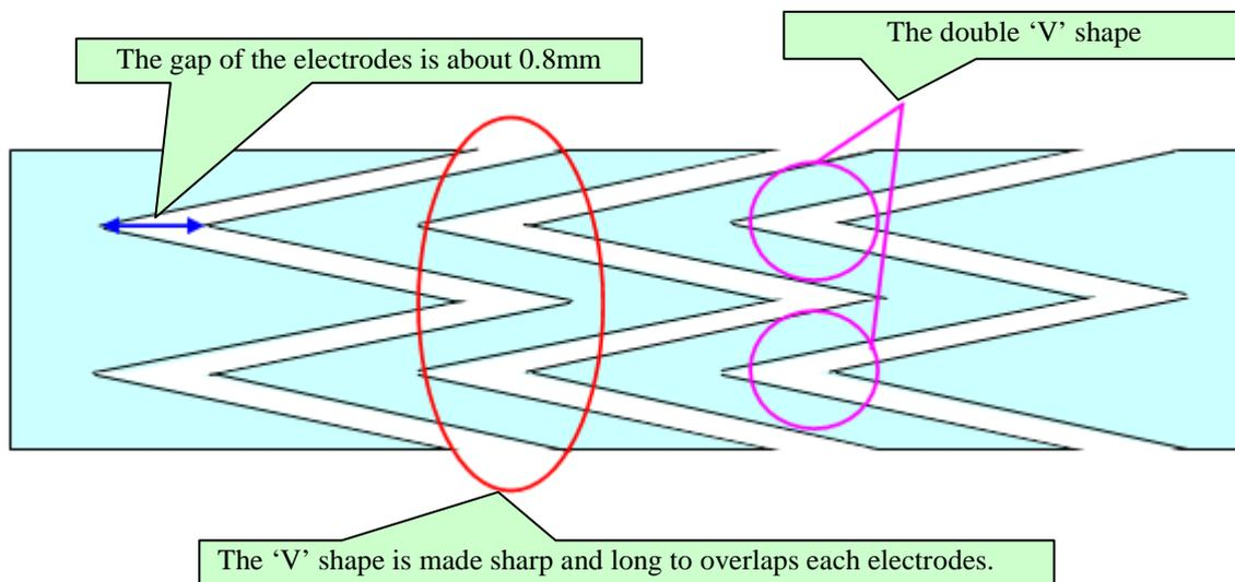
Notice; It is only an example shape of slider. Please modify it for your system, environment, and etc. Because the touch sensitivity is depend on the target of touch detecting (such as light touch or strong touch), the board condition (such as length of line, circuit constants and etc.), external or internal environments and so on.
