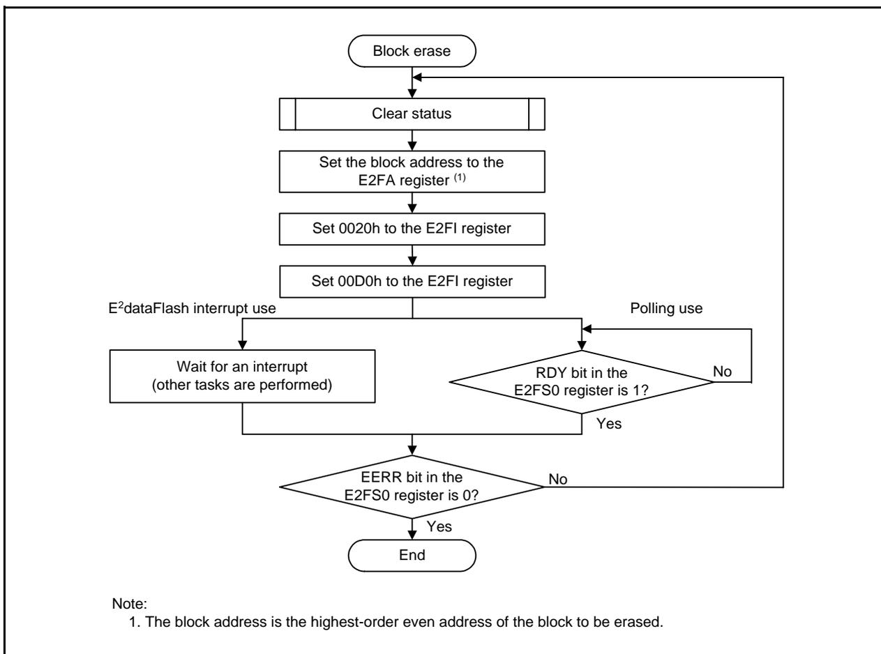
Figure 3.5 Block Erase Operation Example
