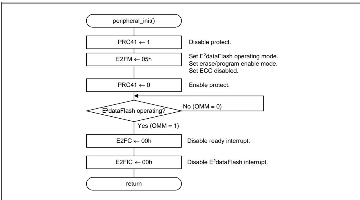
Figure 4.3 Peripheral Function Initial Setting
