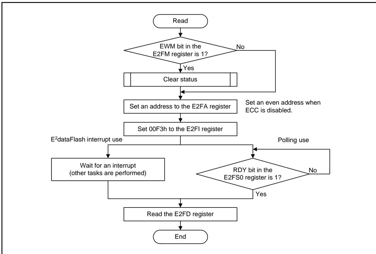
Figure 3.3 Read Operation Example
