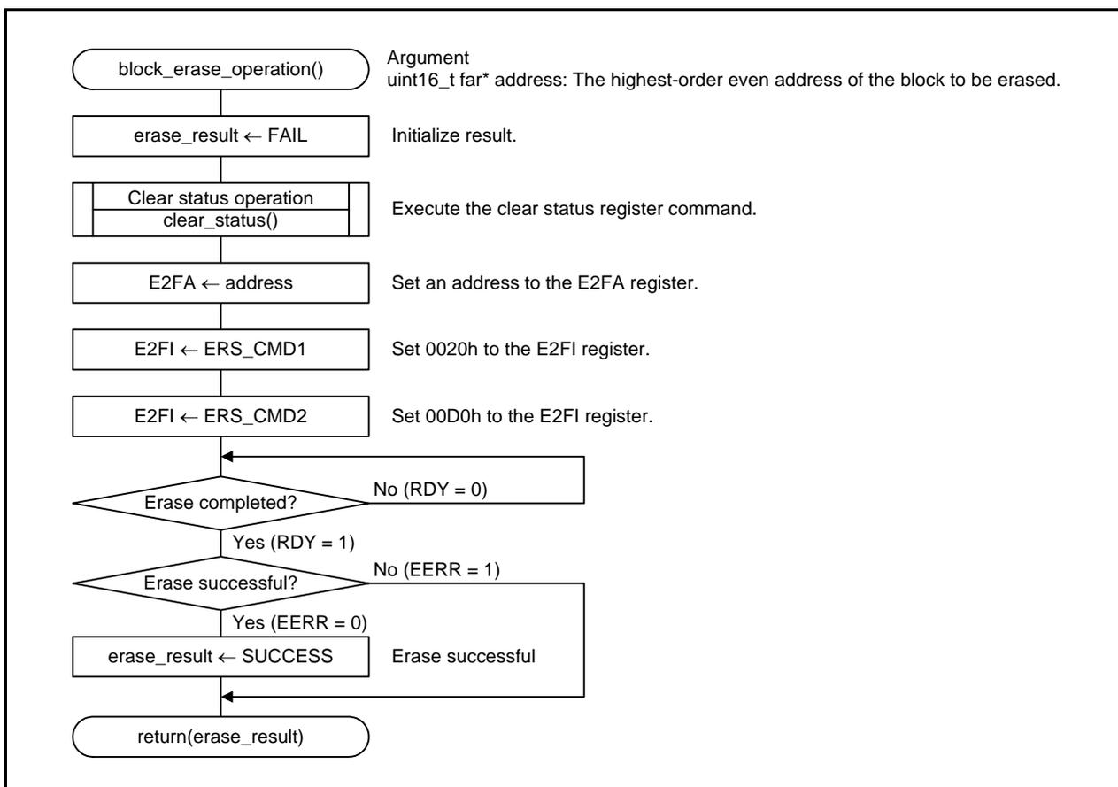
Figure 4.5 Block Erase Operation
