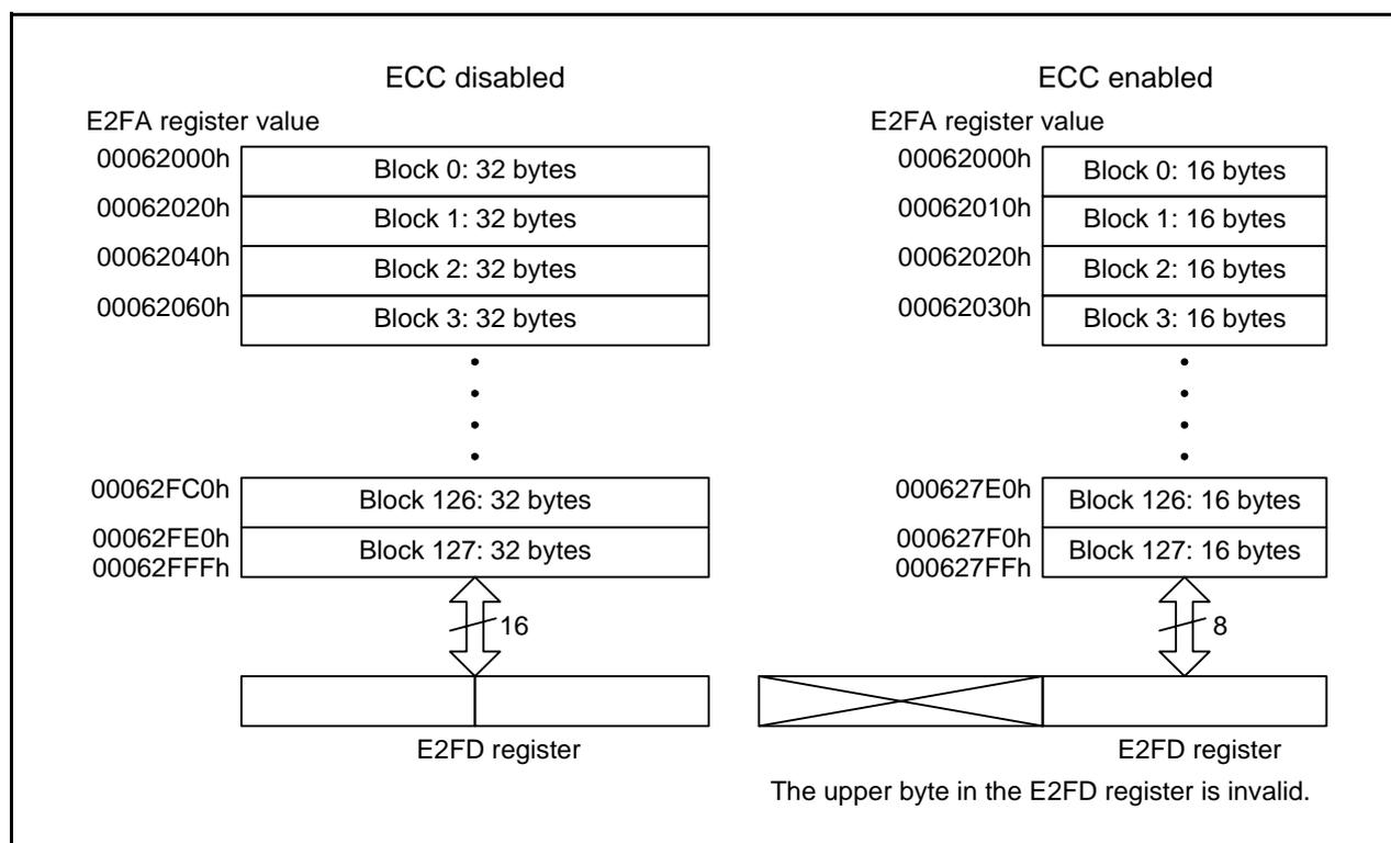
**Figure 3.1 E<sup>2</sup>dataFlash Memory Configuration**
