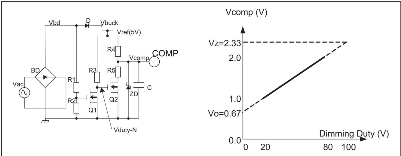
As shown in < Dimming by controlling the voltage of COMP-pin of R2A20134>, the level of the Peak-current would be controlled linearly while the control voltage of COMP-pin is in the range from 1 V to 2 V. ZCD voltage, R4 and R5 should be decided according to this range of COMP-pin control voltage.
