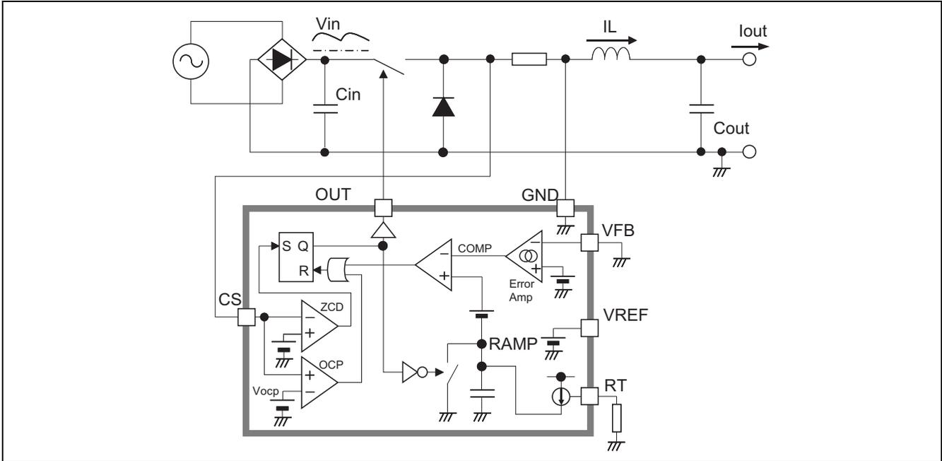
The peak current through inductor is kept constant in the range of  $V_{in} > V_{out}$ . If  $C_{in}$  is big enough to keep always  $V_{in} > V_{out}$ , peak current through inductor is kept constant. This means ripple on output current is reduced efficiently. And built-in error amplifier is not used in this example, less external components is used.
