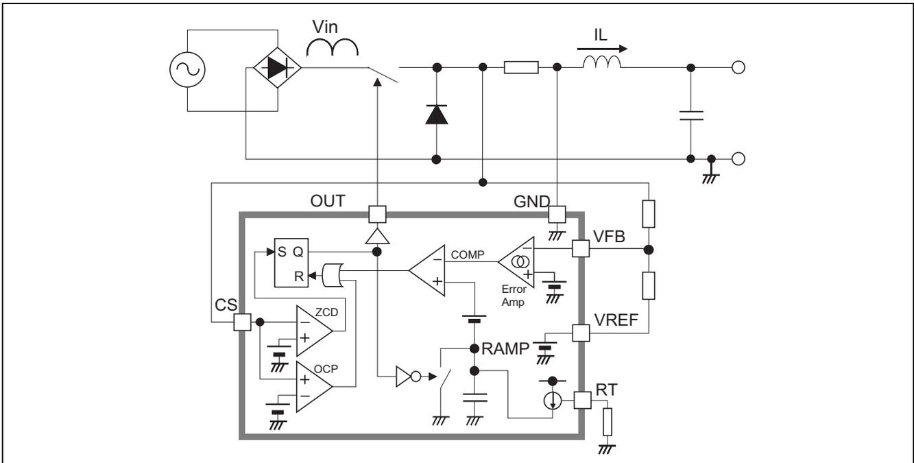
In error amplifier controlled operation, ON time is fixed to constant during nominal operation. If On time is fixed to constant, peak inductor current is changed in proportion to input voltage. This operation corrects power factor.
