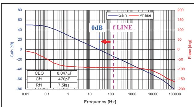
Figure 5.2 Frequency Characteristics of R2A20134EVB-NN1E
