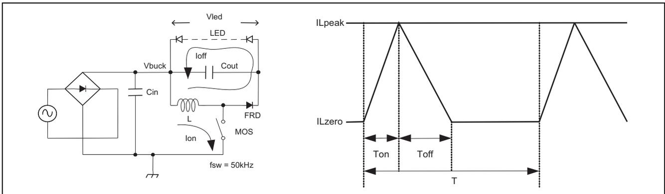
R2A20134 works at the Fixed-Frequency and in the Peak-current operation mode. So  $I_L$  flows through the MOSFET to GND, and  $I_L$  increases from  $I_{Lzero}$  to  $I_{Lpeak}$  while the MOSFET is turned on, that is, during  $T_{on}$ . And  $I_L$  flows through FRD to LED, and  $I_L$  decreases from  $I_{Lpeak}$  to  $I_{Lzero}$  while the MOSFET is turned off, that is, during  $T_{off}$ .
