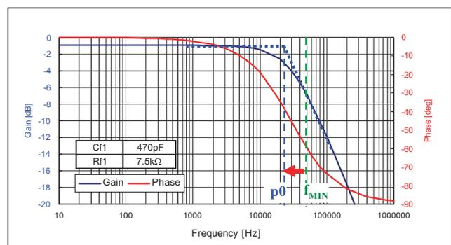
Figure 5.3 Frequency Characteristics of CR Filter of FB Terminal
