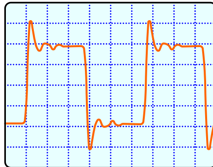
Figure 8. Line Reflections during the First Half of a Bit
