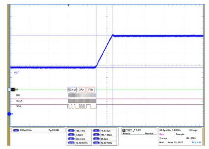
Figure 7: DVC step-up with 12.5mV/µS slew rate
