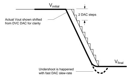
Figure 4: PV88090 DVC down transition measurement example
