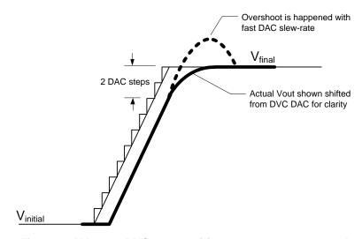
Figure 3: PV88090 DVC up transition measurement example
