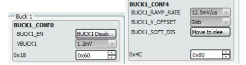
Figure 9: Setting in Dialog GUI\_Sending 0X60 to BUCK1\_CONF0
