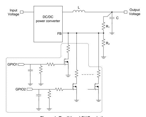
Figure 1: Traditional DVC solution
