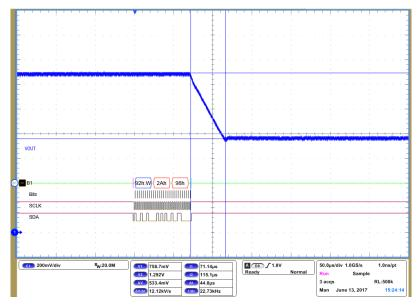
Figure 8: DVC step-down with 12.5mV/µS slew rate
