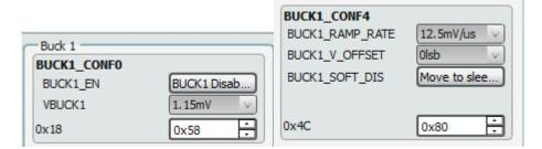
Figure 11: Setting in Dialog GUI\_Sending 0x58 to BUCK1\_CONF0
