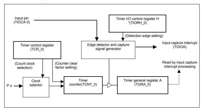
Figure 1 Block Diagram of Pulse Width Measurement
