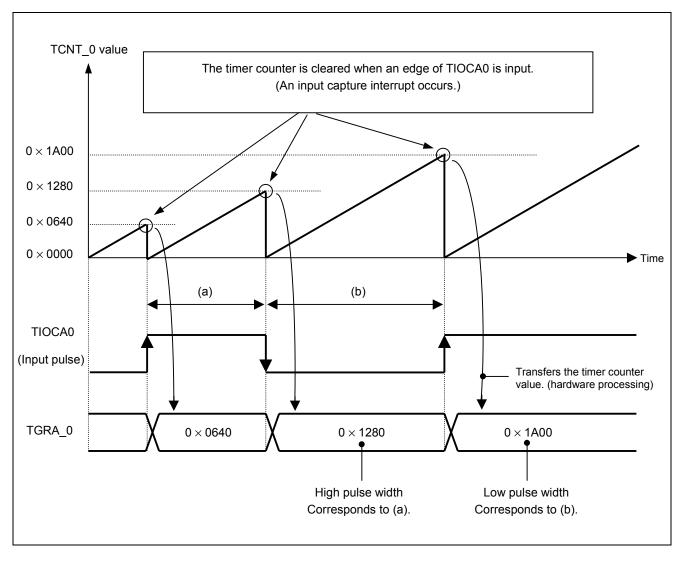
Figure 2 Example of Pulse Width Measurement
