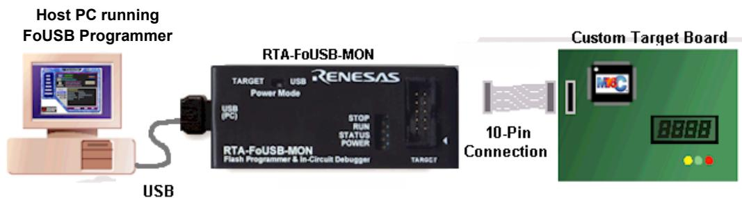
Figure 3 M16C System Connectivity for FoUSB Programmer
